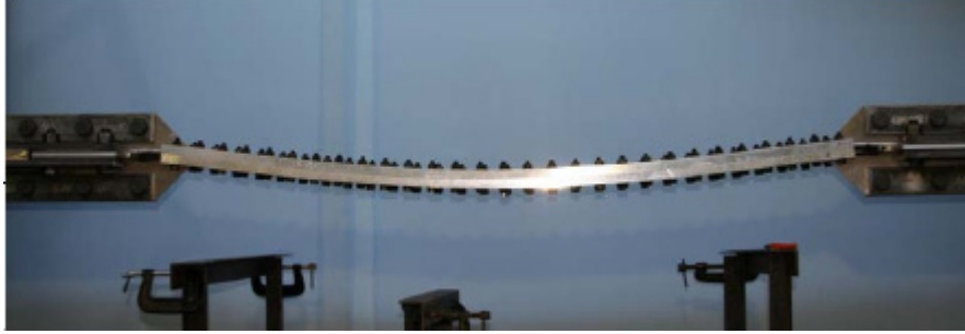
Photo 1 Over-all buckling failure in BRB specimen of B2
