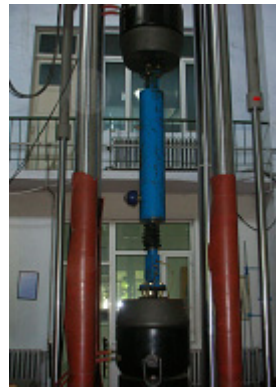
Fig. 14. Photograph of experimental setup with MR specimen.
