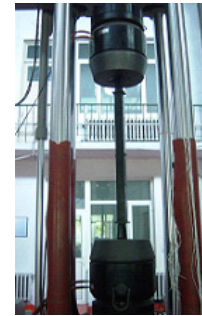
Fig. 8. Photograph of experimental setup with BRB specimen.
