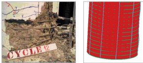
Column test by Fretag et al. (2006) (buckling length=4 hoop spacing)
