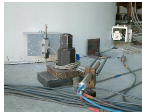
Accelerometers, DCDT's, linpots, and wire pots used to measure tank dynamics
