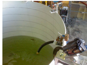
Parallel wire gauges and HD cameras used to monitor water surface dynamics. DCDT's used to measure tank deformation
