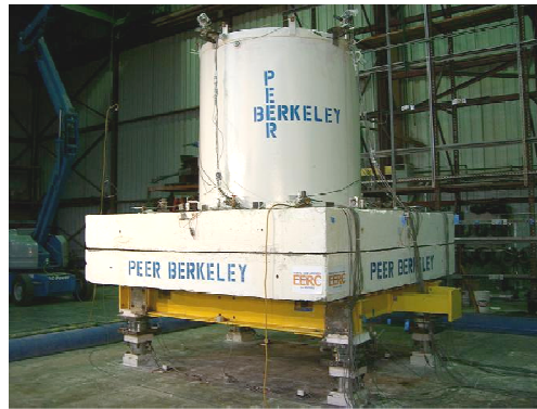
Fully instrumented test specimen on the shaking table.
