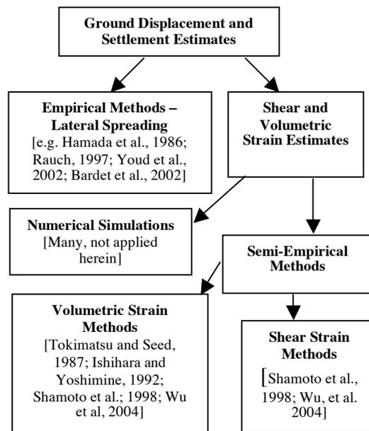
Fig 1. Methods of predicting liquefaction-induced deformation
