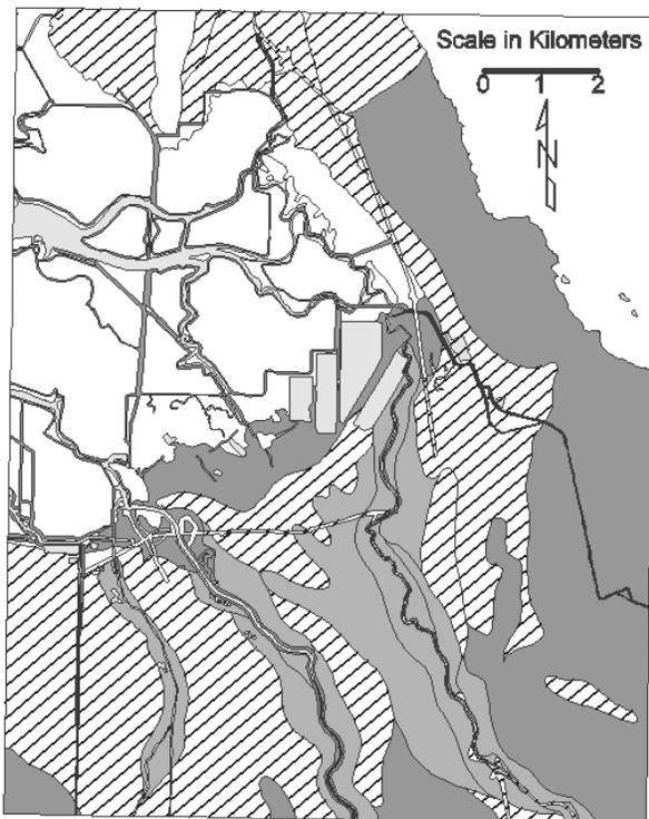
Fig. 2. Liquefaction-induced ground settlement (ft), Milpitas 7.5-minute Quadrangle, California (settlement calculated using Wu et al., 2003 method)
