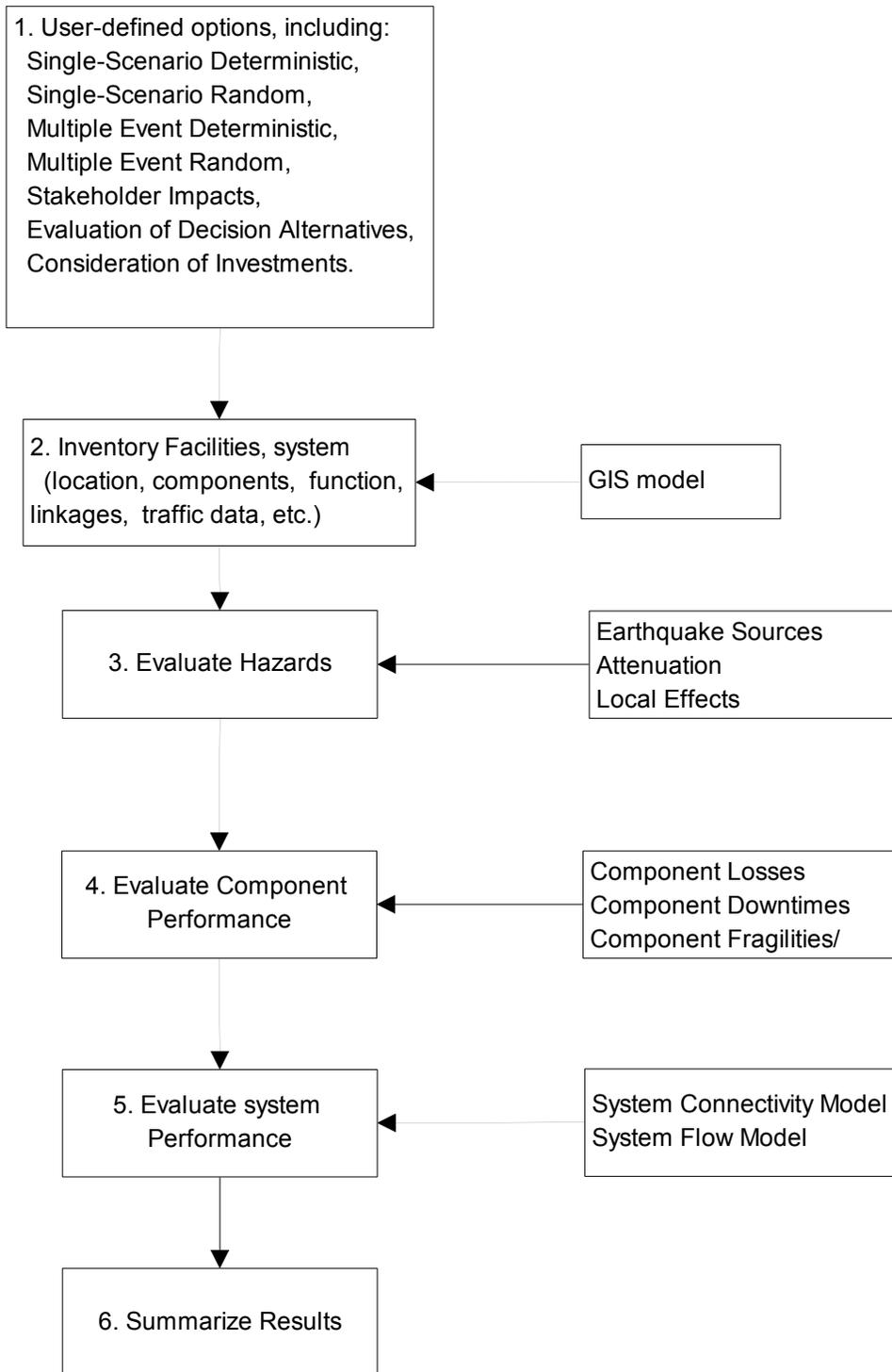
Figure 2. Basic Common Steps in a Seismic Risk/Reliability Evaluation for Lifeline Networks.
