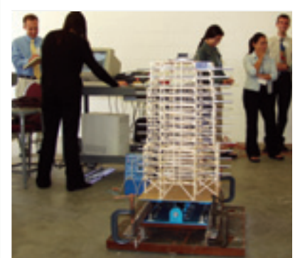
The UCSD model is prepared for testing on the mini-shaker.
