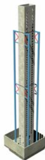
Figure 1. Schematic of seismic-force-resisting system of 60-story building in San Francisco (Magnusson – Klemencic).
