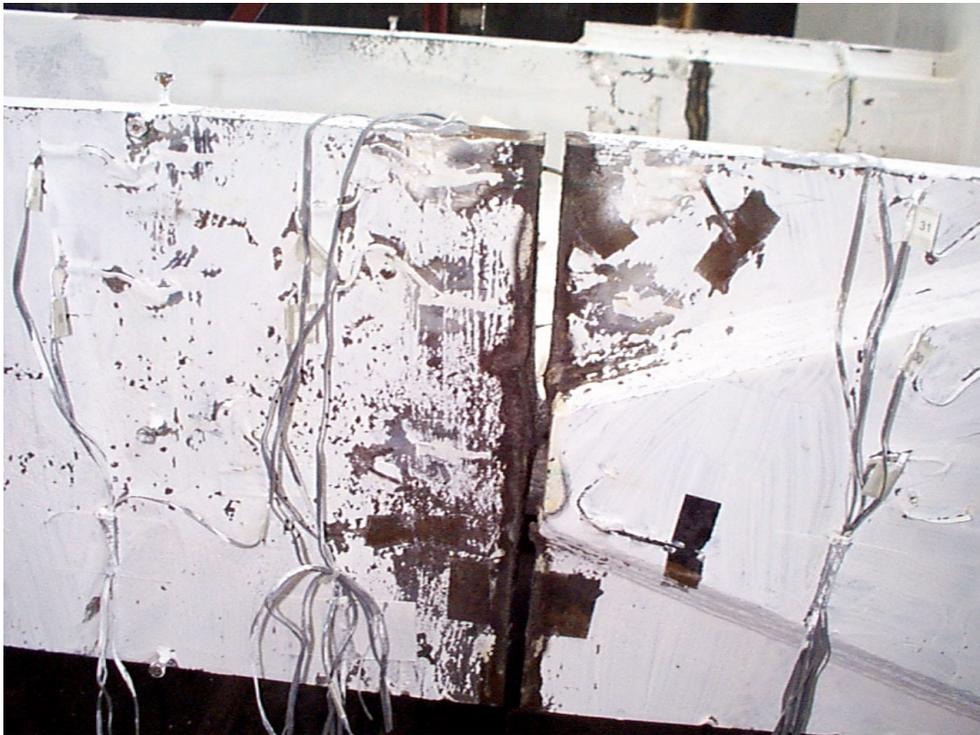
b. view of top flange of beam showing line of fracture
