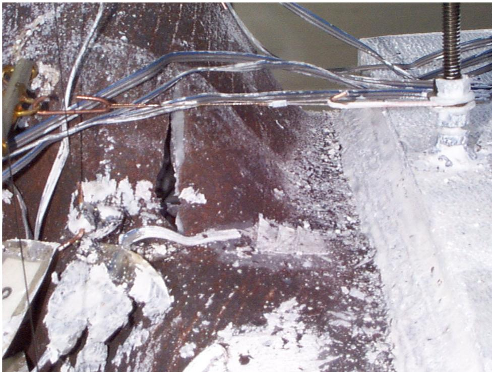
Figure 5-61 Tearing of beam top flange in RC07
