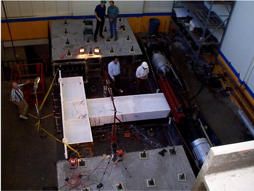
Figure 2-8 Test fixture for the RiverPark II cover-plate specimen
