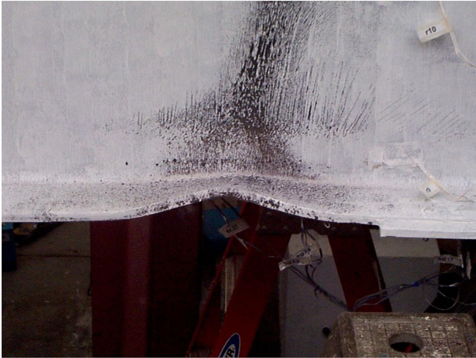
Figure 5-22 Flange local buckling at nose of cover plate in RC03
