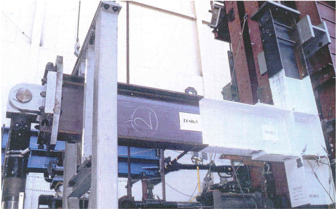
Figure 2-12 Test fixture for FUSD flange-plate specimens (Whittaker and Gilani 1996)
