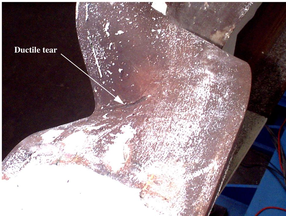
Figure 5-41 Tear in bottom flange of beam in RC05
