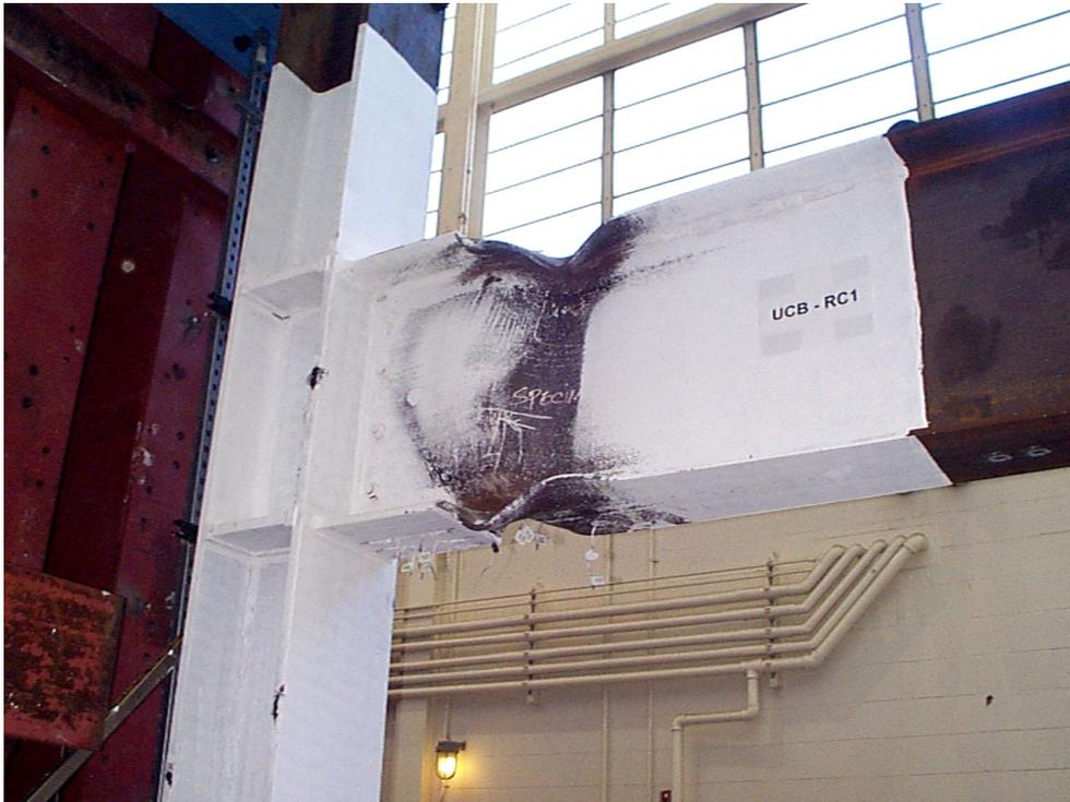
Figure 5-3 Beam FLB and WLB in RC01 at a drift angle of  $0.04h$
