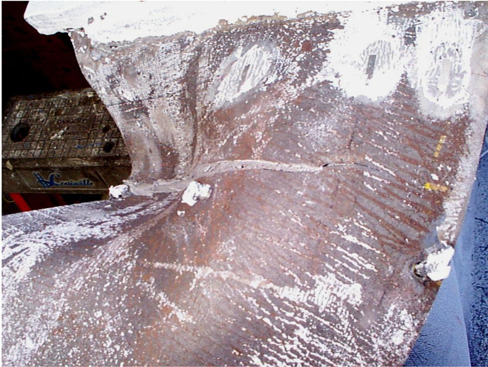
Figure 5-66 Fracture in the beam top flange of RC08
