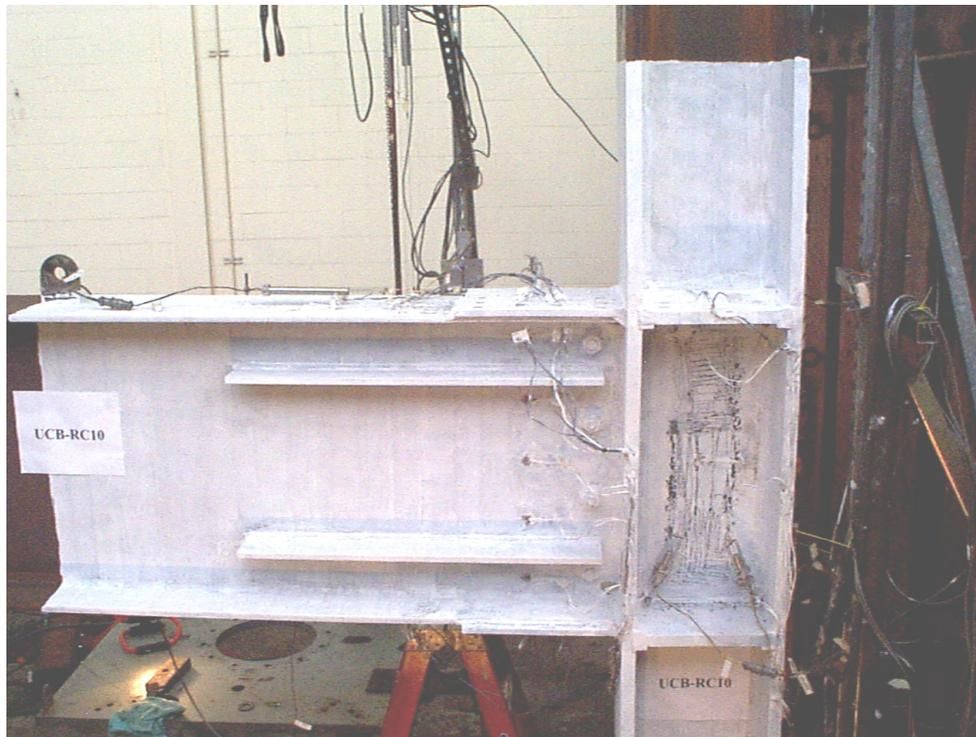
Figure 5-85 Horizontal stiffeners on RC10 to delay web local buckling
