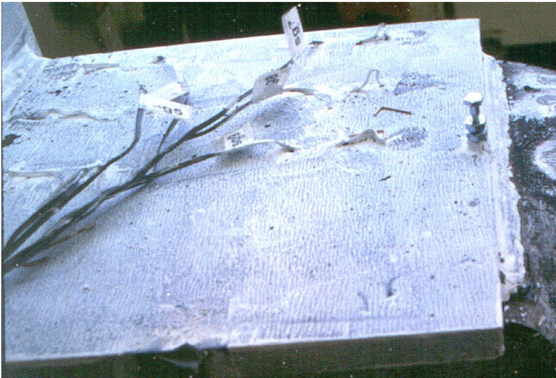
Figure 5-67 Yielding of flange plate in RC08 at a drift angle of  $0.04h$
