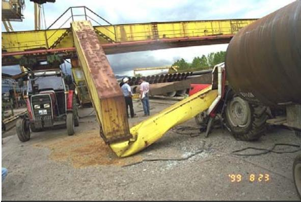
**Figure 4-60b. Collapsed crane leg, Mannesmann Boru pipe storage facility**
