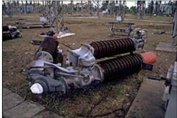
**Figure 4-50b. Failed porcelain circuit breakers**
