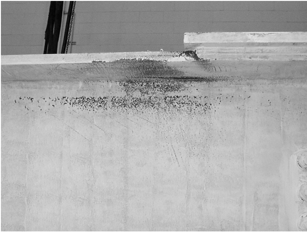
Figure 2-27. Specimen 2: top beam flange buckling
