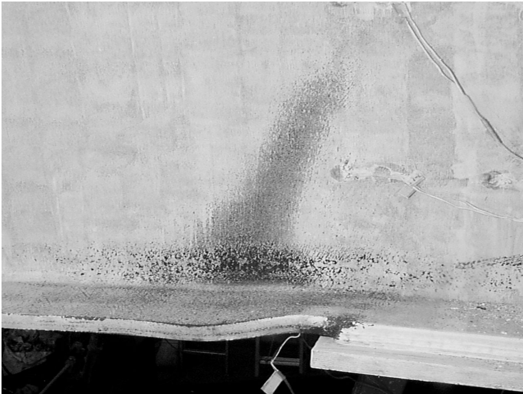
Figure 2-28. Specimen 2: bottom beam flange buckling
