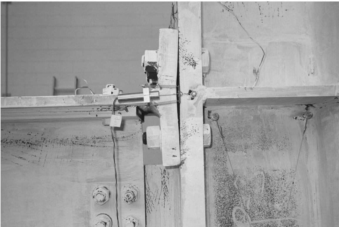
Figure 2-9. Residual gap opening in the upper T-section (after the test)
