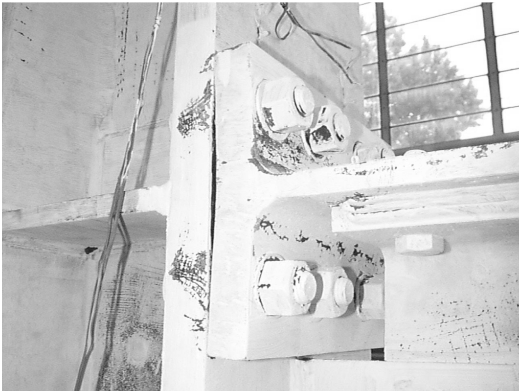
Figure 2-26. Specimen 2: residual gap opening in top T-section
