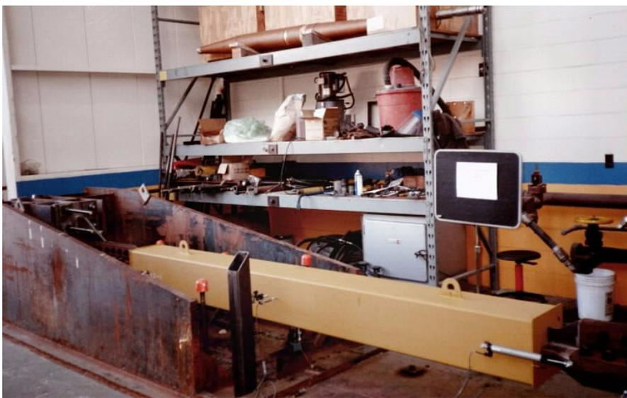
**Figure 4-7.** Views of the unbonded brace mounted on the fall 2000 test setup.
