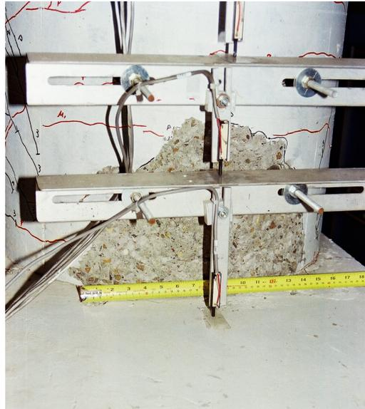
**Fig. 5.10 North plastic hinge:  $\mu=3$  current design, quasi-static test**
