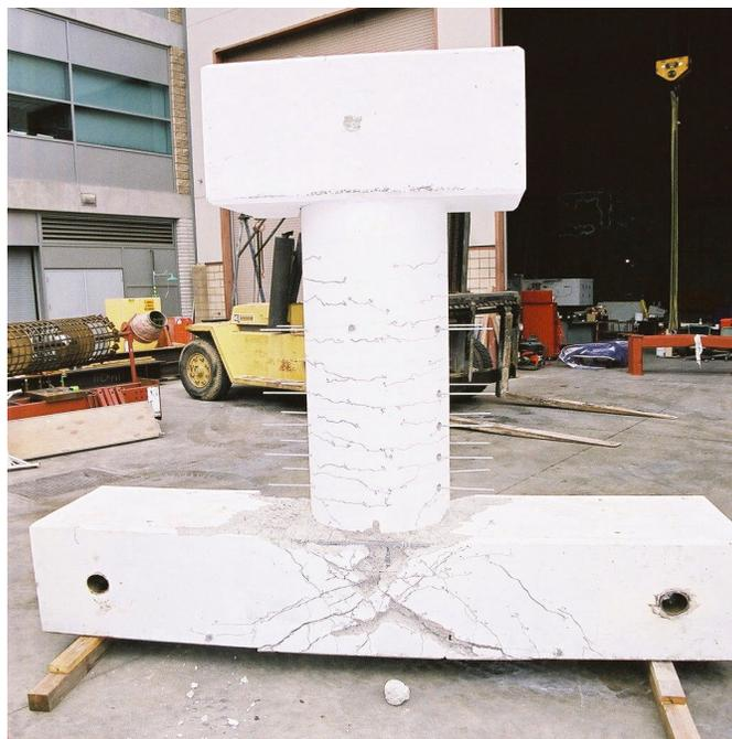
**Fig. 5.20 Pre-1971 specimen after quasi-static test (north is right)**
