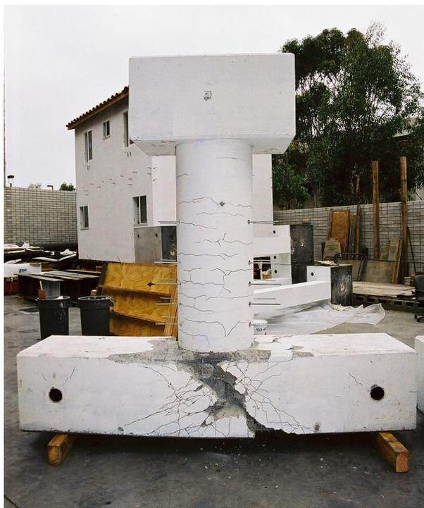
**Fig. 5.22 Pre-1971 specimen after dynamic test (north is right)**
