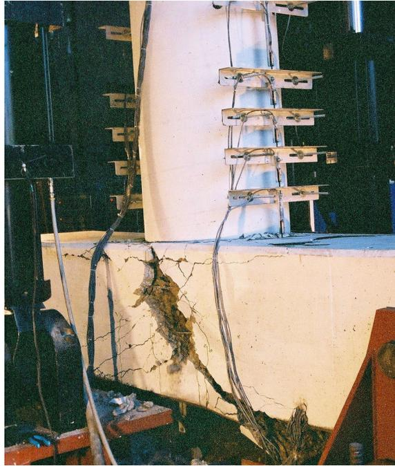
**Fig. 5.21 Pre-1971 joint at failure of dynamic test (view from north)**
