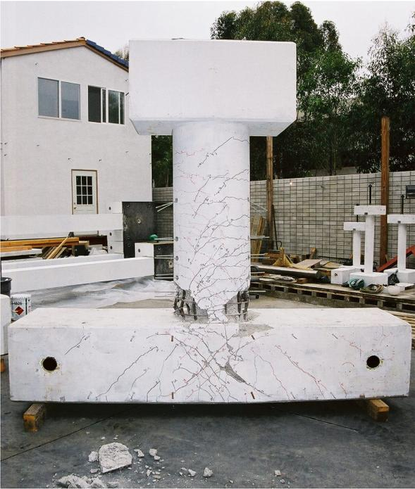
**Fig. 5.16 Current design after quasi-static test (north is left)**
