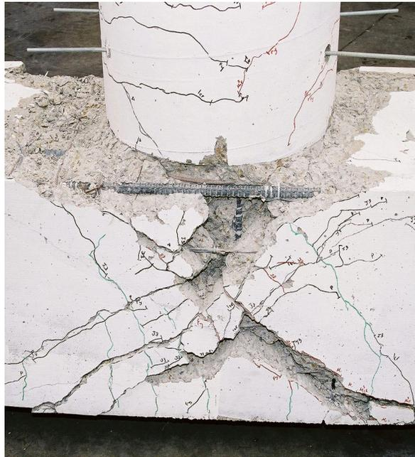
**Fig. 5.19 Pre-1971 joint after quasi-static test (east view of joint)**
