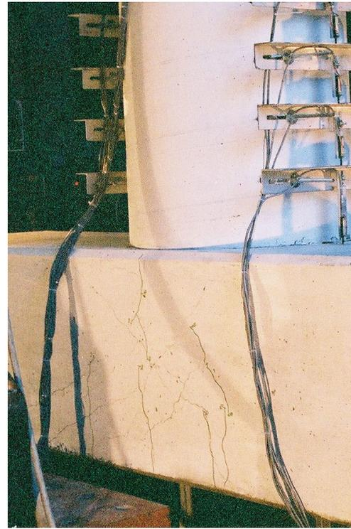
**Fig. 5.8 Peak of pulse: pre-1971 design, dynamic test**
