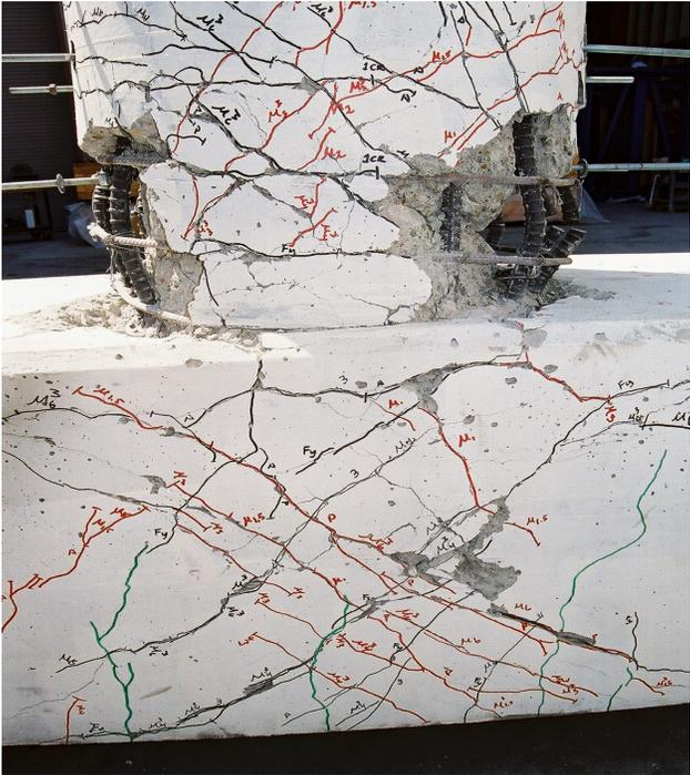
**Fig. 5.15 Current design after quasi-static test (north is right)**
