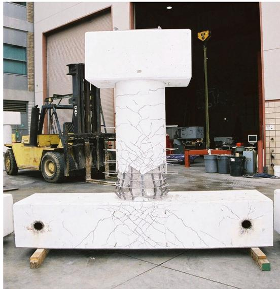
**Fig. 5.18 Current design after dynamic test (north is left)**
