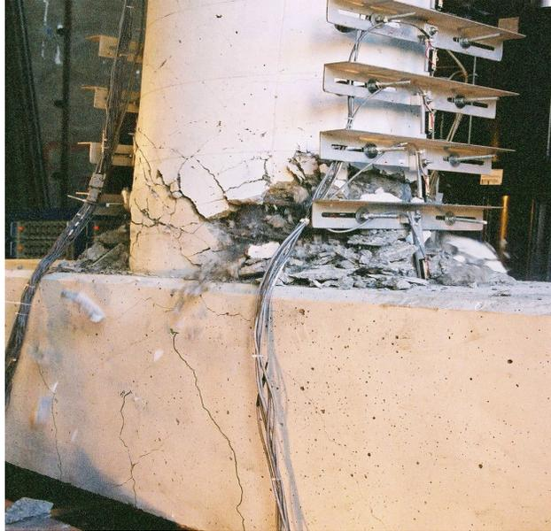
**Fig. 5.17 Failure of dynamic current design (view from north)**
