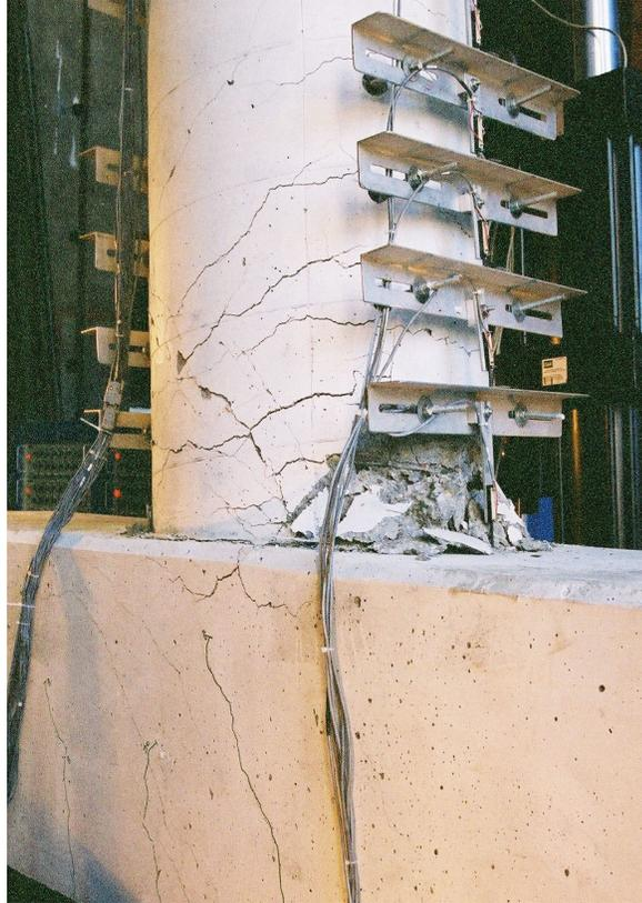
**Fig. 5.12 North plastic hinge:  $\mu=6$  dynamic test**
