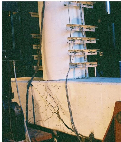
**Fig. 5.14 Joint around  $\mu=4$ : pre-1971 design, dynamic test**
