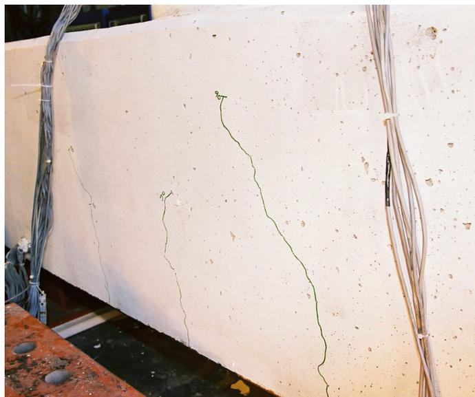
**Fig. 5.1 Cracking in beam joint from gravity load**
