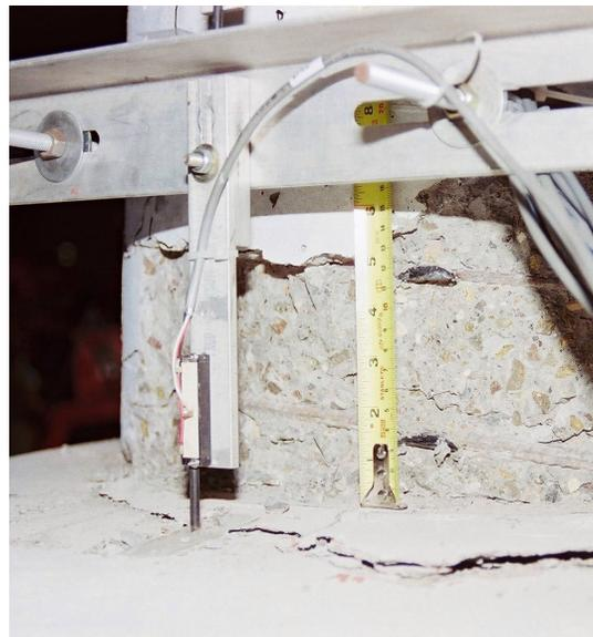
**Fig. 5.11 South plastic hinge:  $\mu=6$  current design, quasi-static test**
