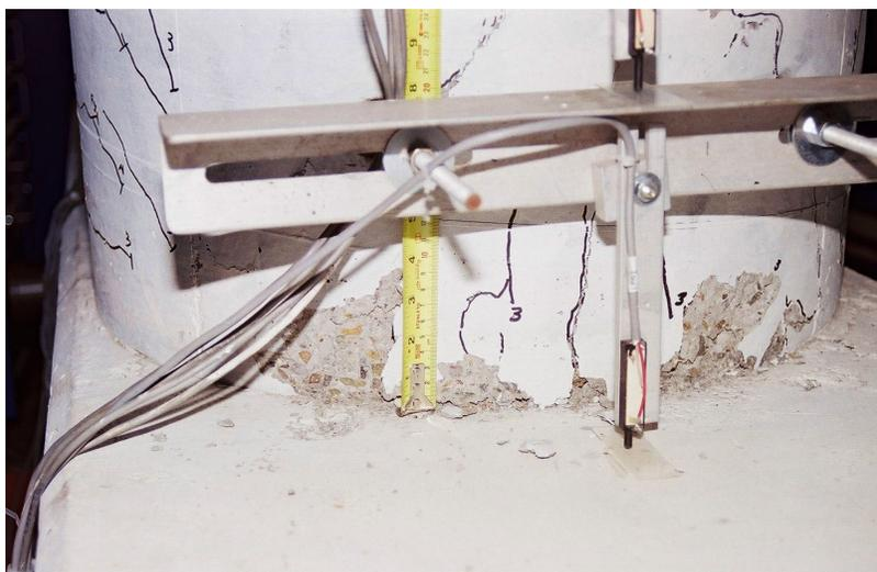
**Fig. 5.6 Peak of positive pulse: current design, quasi-static test**
