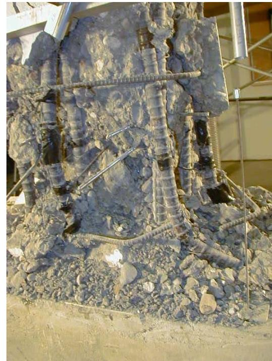
**Figure 3.17** - Specimen S20HI at 7% Lateral Drift after Axial Load Capacity Lost
