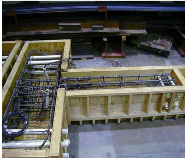
**Figure 2.7** - Reinforcement Cages before Placing Concrete
