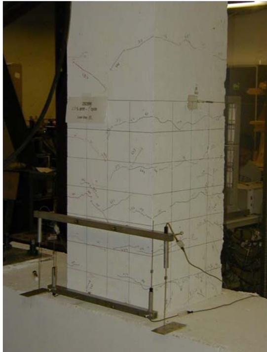
**Figure 3.5** - Specimen S20MI at 1.0% Drift (Left)
