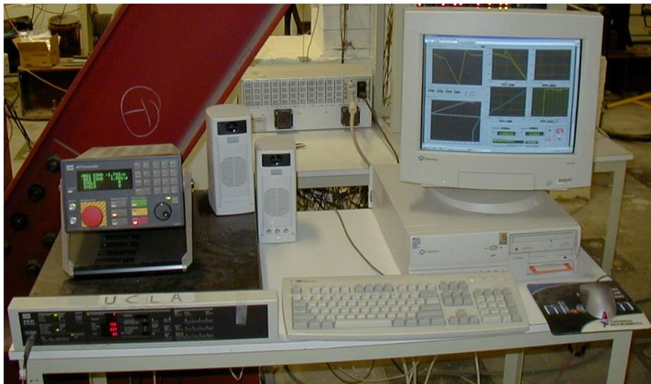
**Figure 2.25** - Data Acquisition Device and MTS 407 Controller
