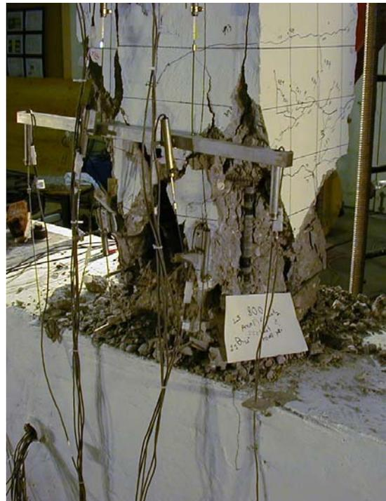
**Figure 3.19** - Specimen S30XI at 5% Lateral Drift after Axial Load Capacity Lost
