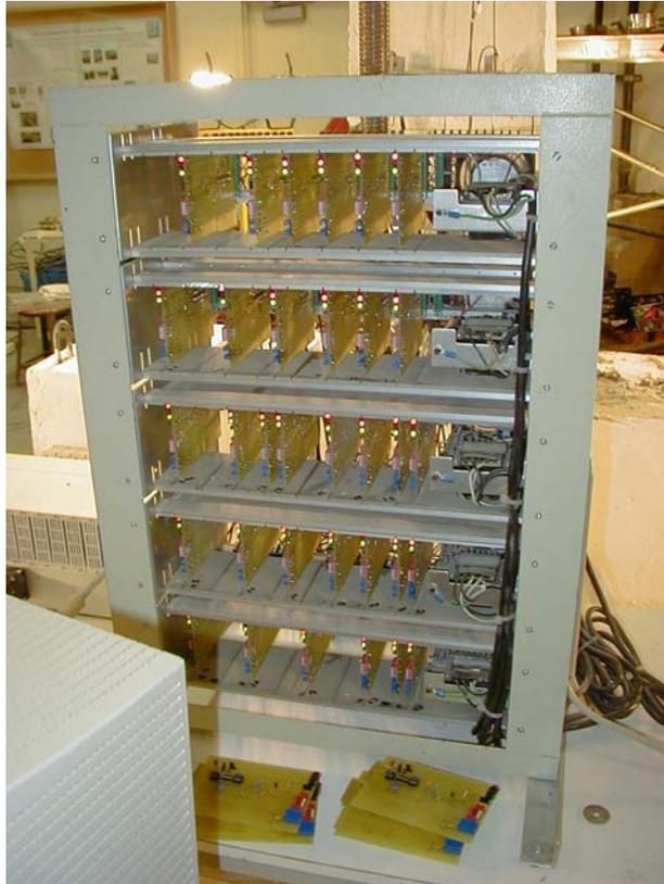
**Figure 2.27 - Strain Gauge Amplifier**
