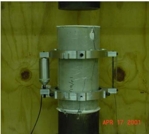
**Figure 2.2** - Standard Concrete Compressive Test
