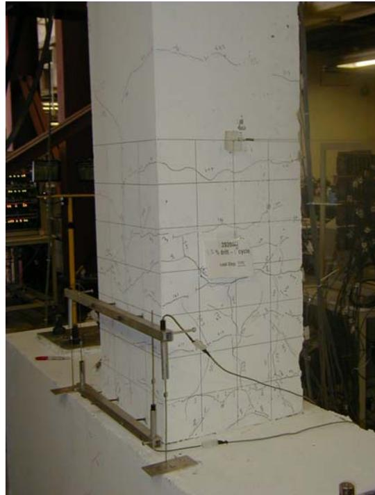
**Figure 3.7 - Specimen S20MI at 2.0% Lateral Drift**
