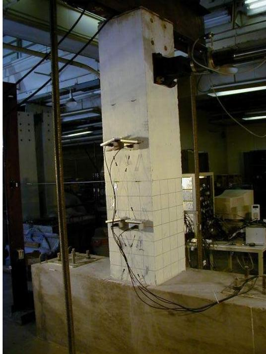
**Figure 2.21** - Shear Instrumentation (S20HI, S20HIN, S30XI)
