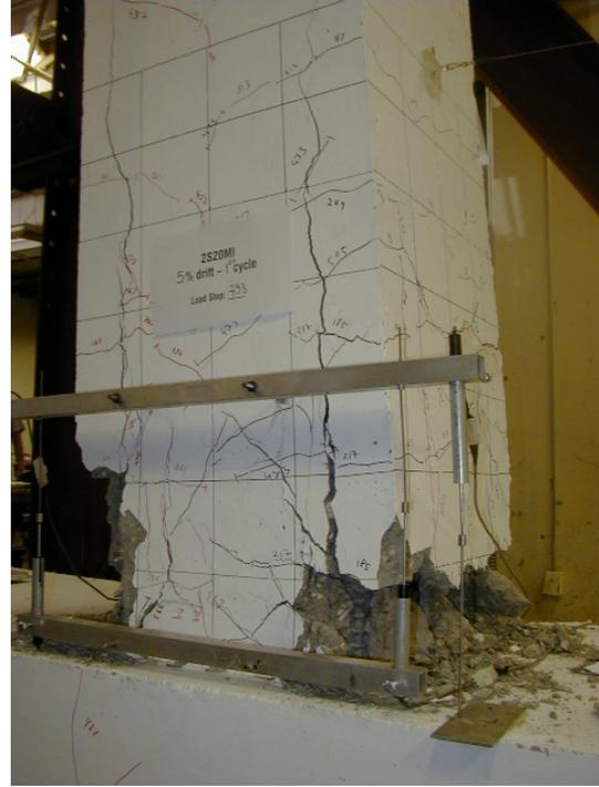
**Figure 3.9** - Specimen S20MI at 5.0% Lateral Drift
