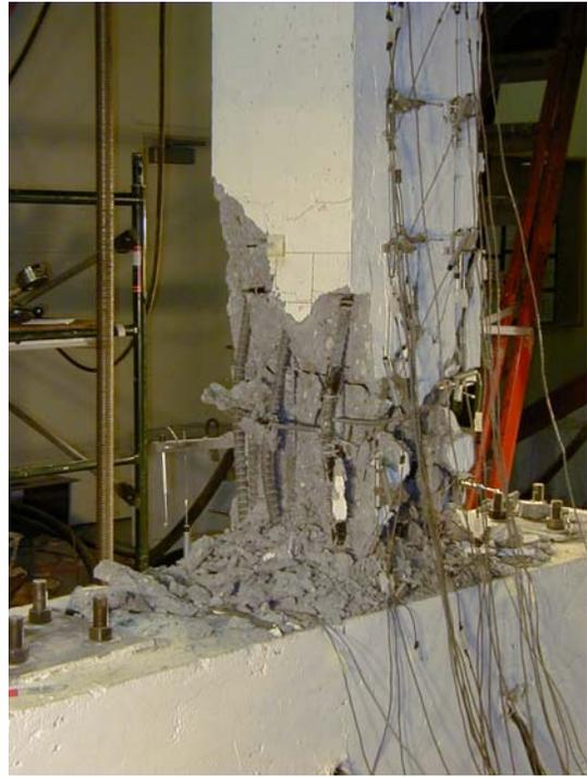
**Figure 3.16** - Specimen S30MI at 5% Lateral Drift after Axial Load Capacity Lost
