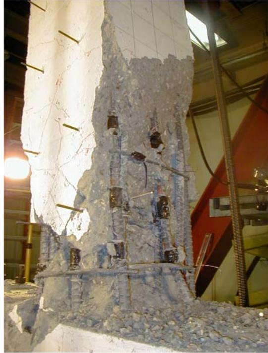
**Figure 3.14** - Specimen S10MI at 10% Lateral Drift—Axial Load Capacity Maintained
