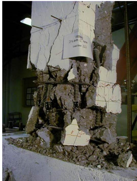
**Figure 3.15** - Specimen S20MI at 7% Lateral Drift after Axial Load Capacity Lost
