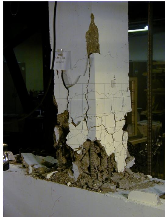
**Figure 3.10** - Specimen S20MI at 7.0% Lateral Drift
