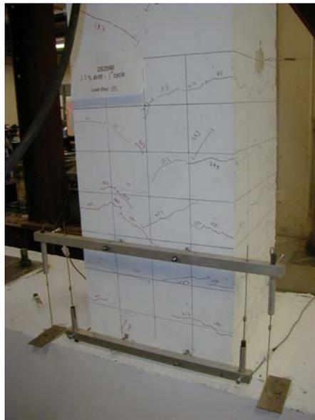
**Figure 2.19** - Transducers Used to Measure Total and Slip Rotation at Column Base (S10MI, S20MI, S30MI)
