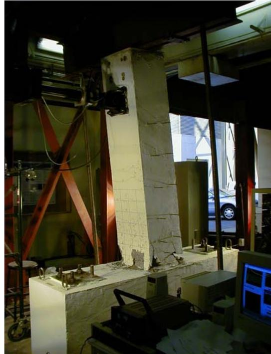
**Figure 3.18** - Specimen S20HIN at 12% Lateral Drift—Axial Load Capacity Maintained
