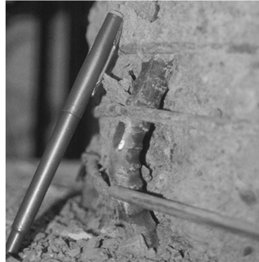
**Figure 1.1 (a) Cover Spalling, and (b) Longitudinal Bar Buckling (Lehman 2003)**
