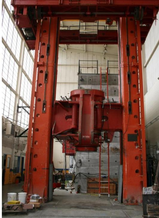
**Figure 6: 4,000 kip capacity compression machine**
