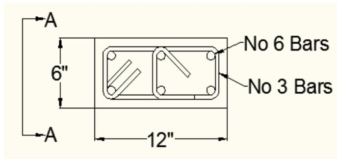
**Figure 3: Cross-section of boundary element**
