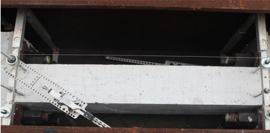
**Figure 16: Specimen 1 before tension test**
