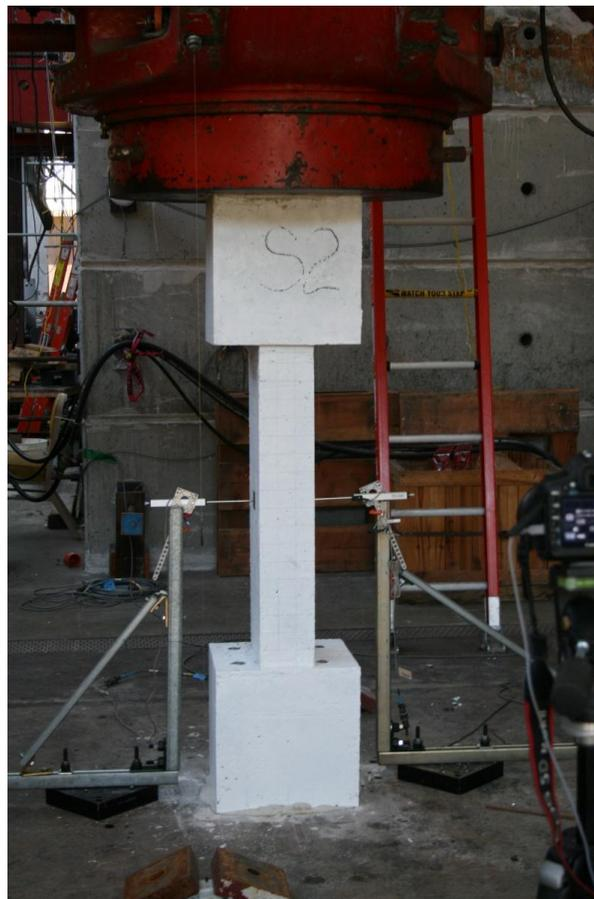
**Figure 15: Compression test set up**
