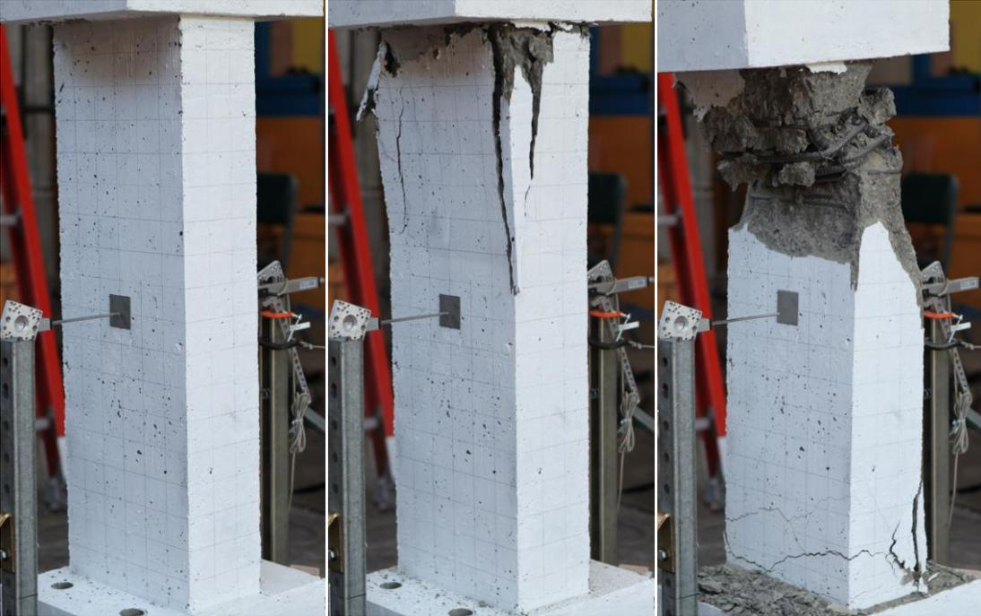
**Figure 19: Specimen 2 compression test results**
