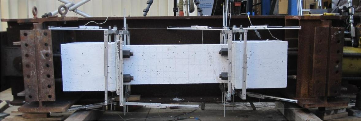
**Figure 14: Tension apparatus before wide flange was attached**
