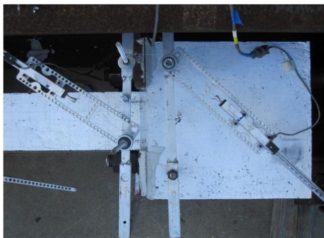
**Figure 11: Aerial view of Novatechnik transducers used in tension test**
