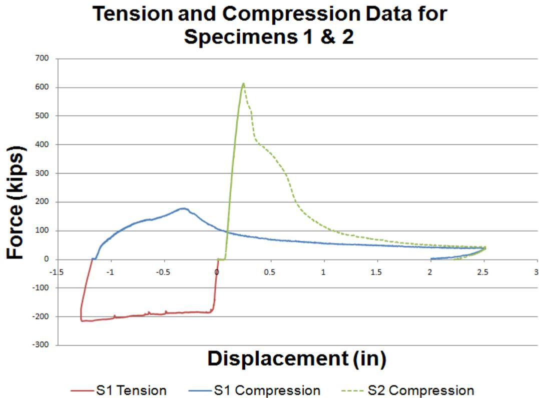
**Figure 20: Force vs displacement chart of Specimens 1 and 2**
