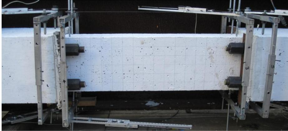
**Figure 12: Side view of brackets and Novatechnik locations in tension test**
