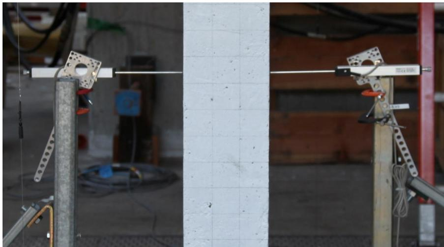
**Figure 13: Novatechnik orientations in compression test**
