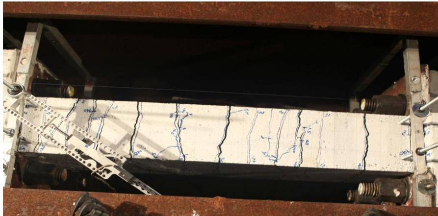
**Figure 17: Specimen 2 after tension test**
