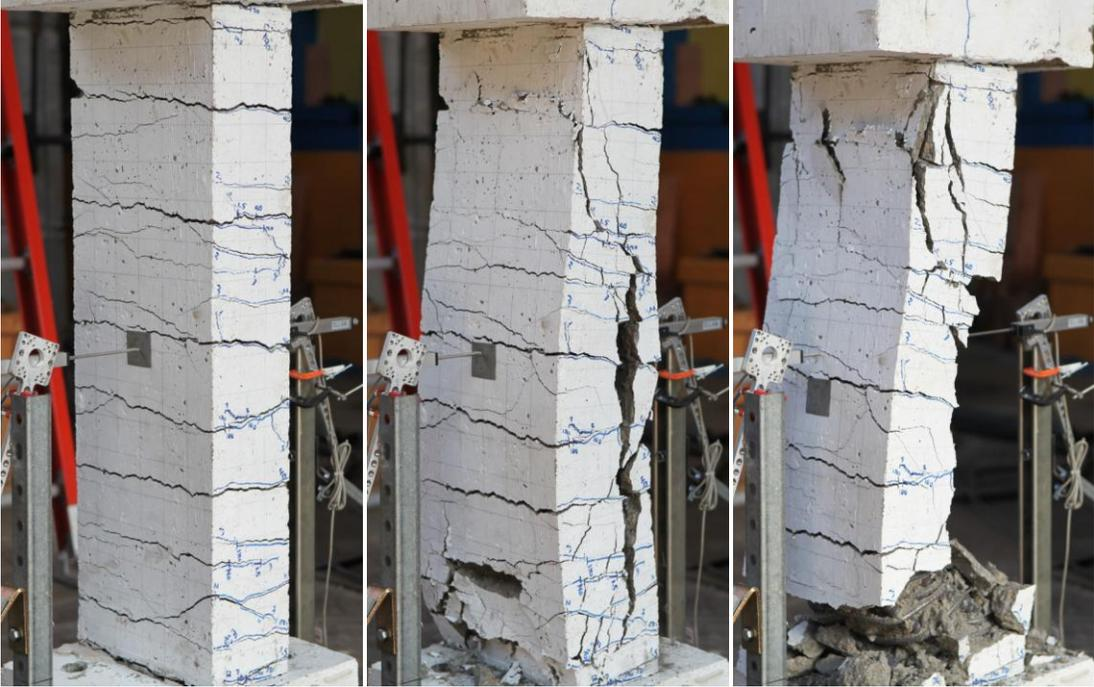
**Figure 18: Specimen 1 compression test results**
