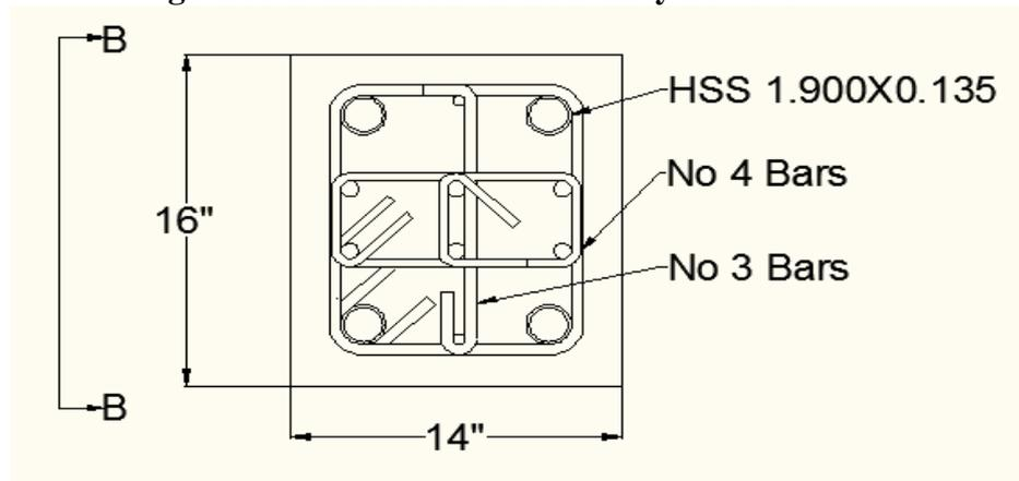
**Figure 4: Cross-section of tension head**
