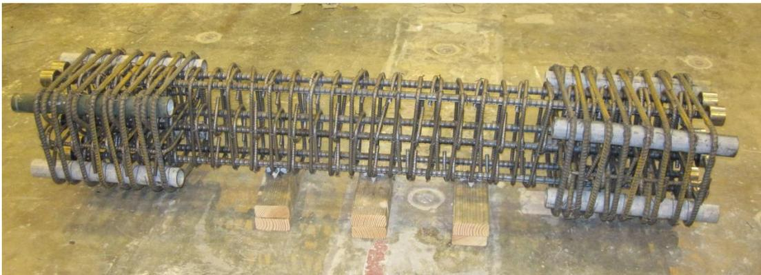
**Figure 7: Reinforcement cage**
