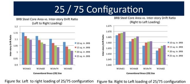
Figure 9a: Left to right loading of 25/75 configuration Figure 9b: Right to Left loading of 25/75 configuration
