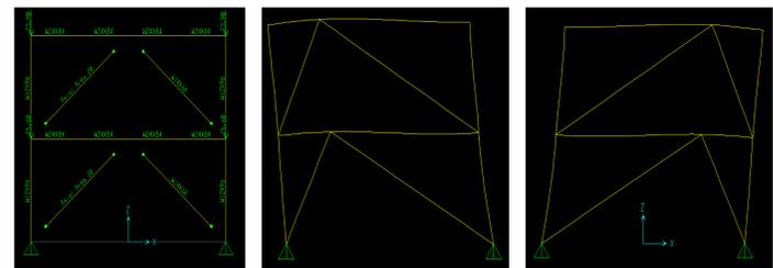
Figure 6a: 50/50 Configuration before analysis with dead load shown Figure 6b: 25/75 configuration after analysis of right to left earthquake loading Figure 6c: 75/25 Configuration after analysis of left to right earthquake loading
