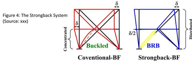
Figure 4: The Strongback System (Source: xxx)
