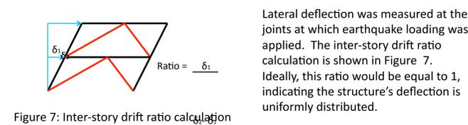
Figure 7: Inter-story drift ratio calculation
