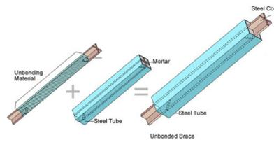
Figure 2: The BRB Components (Source: Nippon Steel)
