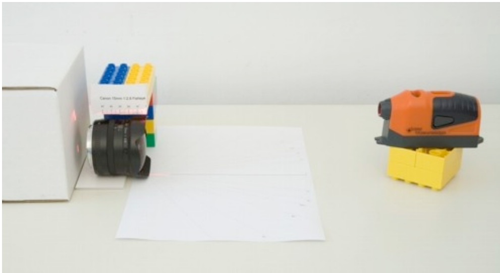
Fig. 3 Set-up for calculating nodal points on cameras ( source: Thomas Schwenger ).
