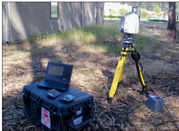
Fig. 11 Set-up of Leica ScanStation 2
