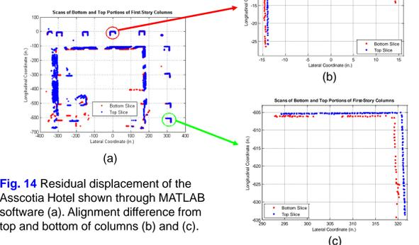
Fig. 14 Residual displacement of the Asscotia Hotel shown through MATLAB software (a). Alignment difference from top and bottom of columns (b) and (c).
