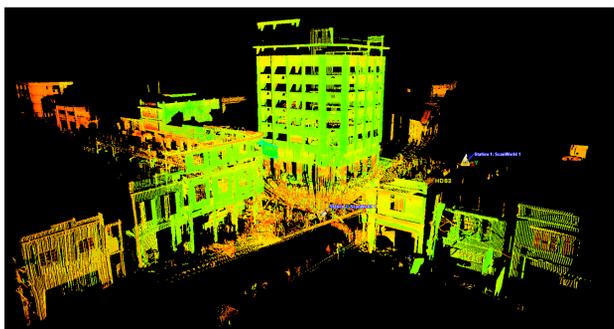
Fig. 1 Leica laser scanned image of the intersection of Mirand and Grand, Port-au-Prince, Haiti.
