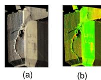
Fig. 9 Station 2: fine and coarse scans colored by colors from camera on board (a) and based on intensity of received light (b).
