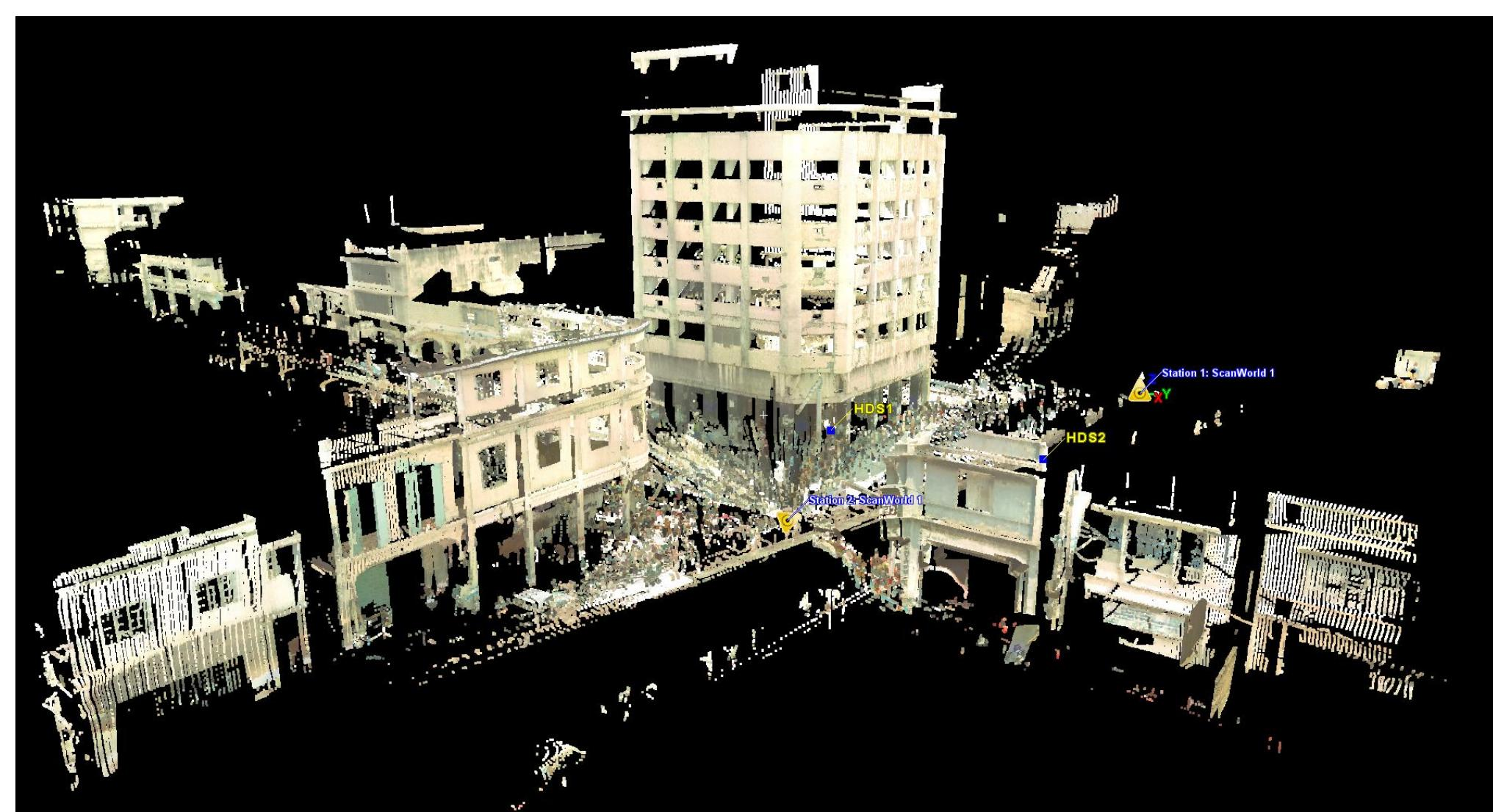
Fig. 6 Resultant image of high-definition photographs superimposed upon laser scan of Mirand and Grand intersection. This image demonstrates the advantage of having scanned and high-definition images to show earthquake damage as apposed to a satellite's aerial view.
