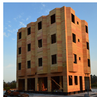
The NEES-Soft Project's four-story soft-story building specimen prior to testing on the NEES@UCSD shaking table (source: M. Gershfeld)
