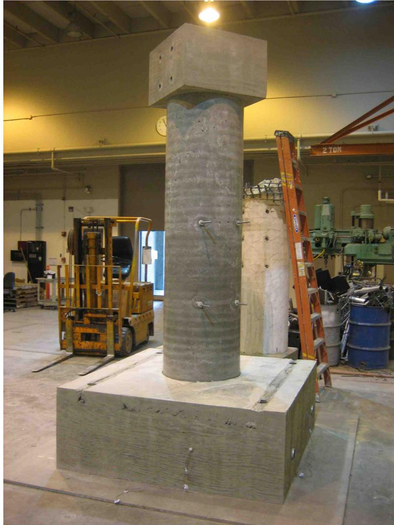
Figure 3.28: Column C4 Inside Laboratory Before Testing
