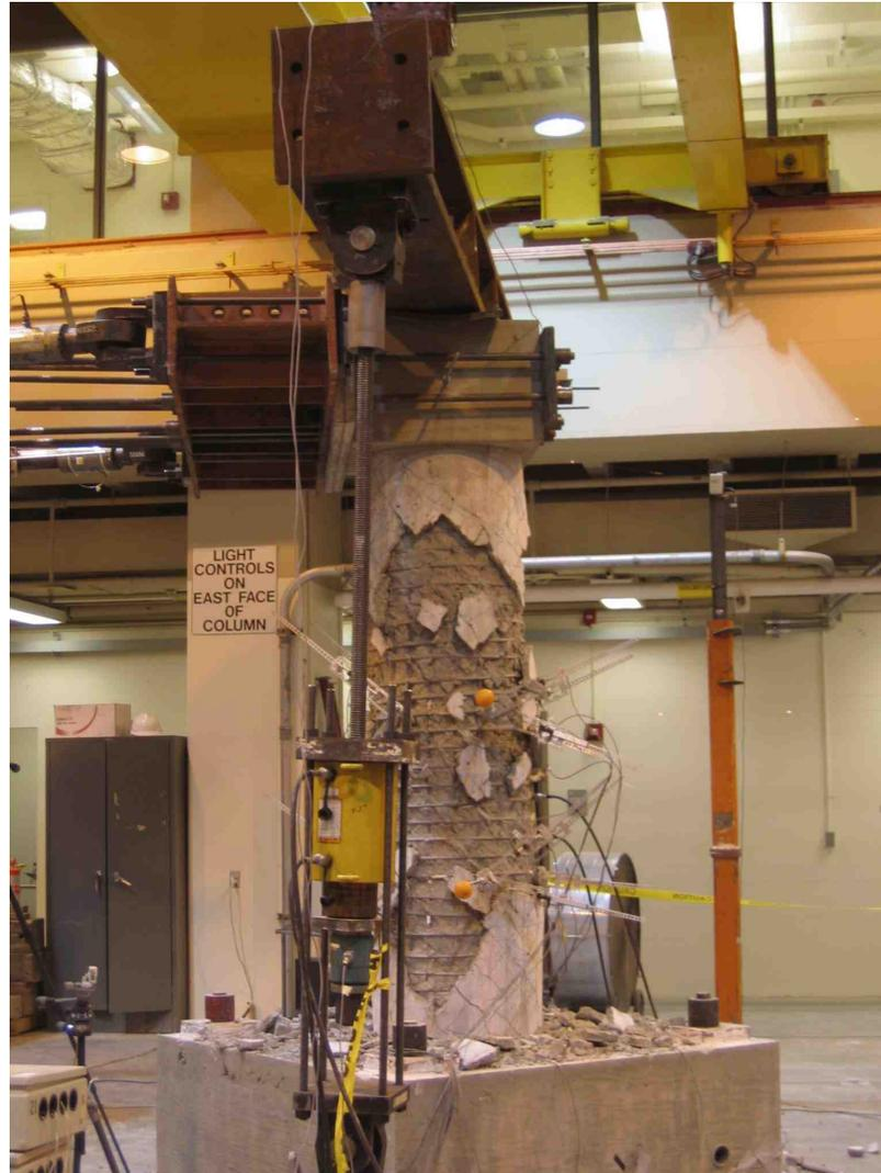
Figure 5.14: Spreader Beam and Column Cap Not Twisting in Unison During First 5 deg Twist Amplitude Cycle (Le, 2008)
