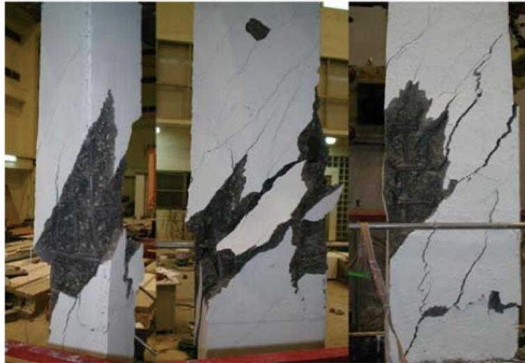
Figure 2.8: Failure Mechanism of Members Subjected to Pure Torsion (from Hsu and Liang, 2002)
