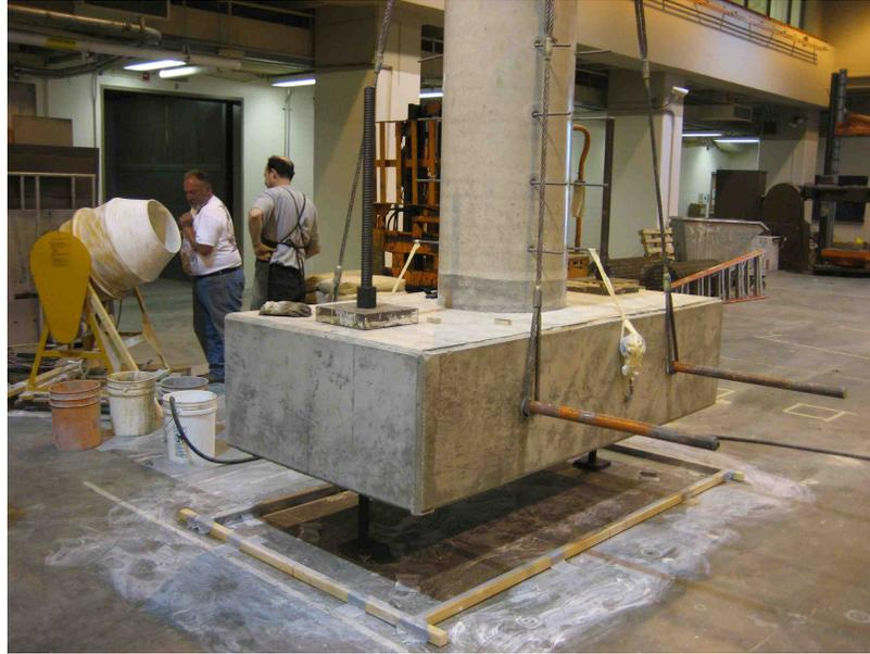
Figure A.1: Positioning of Specimen on Laboratory Floor
