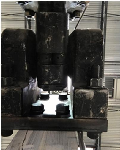
**Figure C.11** Connecting link to specimen column flange.
