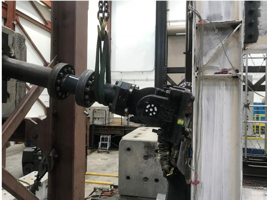
**Figure C.10     Raising link attached to mass rig.**
