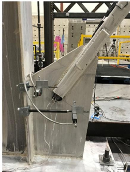
**Figure C.20** LVDT's Attached to south gusset plate.
