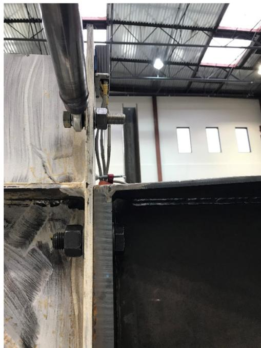
**Figure C.16** Out-of-plane restraining link attached to specimen column flange.
