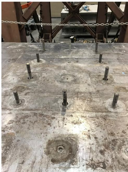
**Figure C.3** Alignment anchors on the shake table.
