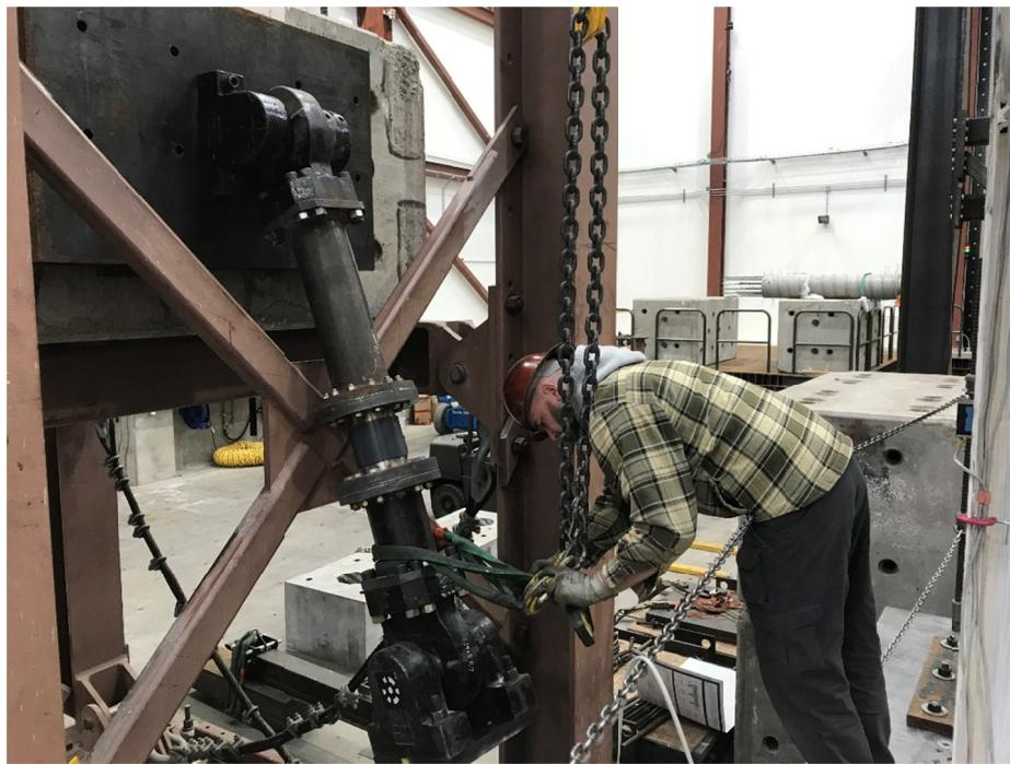
**Figure C.9     Holding link attached to mass rig.**
