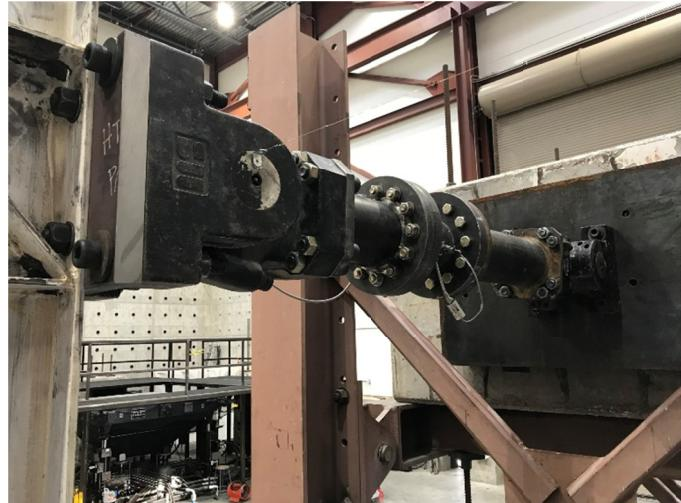
**Figure C.12** Final link attached to mass rig and specimen.
