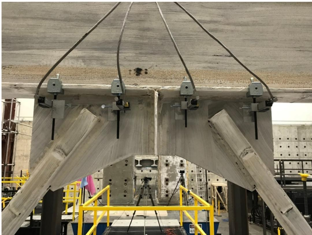
**Figure C.19** LVDT's attached to middle gusset plate.
