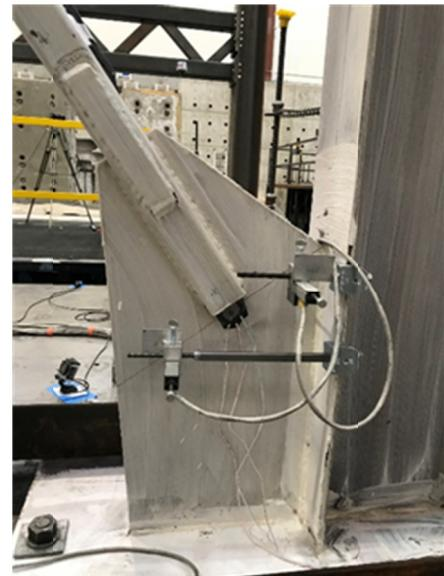
**Figure C.21** LVDT's attached to north gusset plate.
