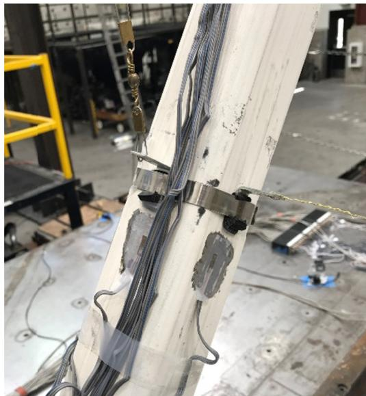
**Figure C.17** Hose clamps around braces for out-of-plane strain pots.
