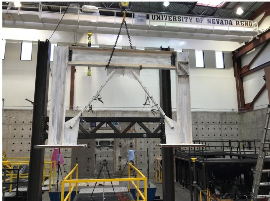
**Figure C.2** Specimen lifted for placing on the shake table.
