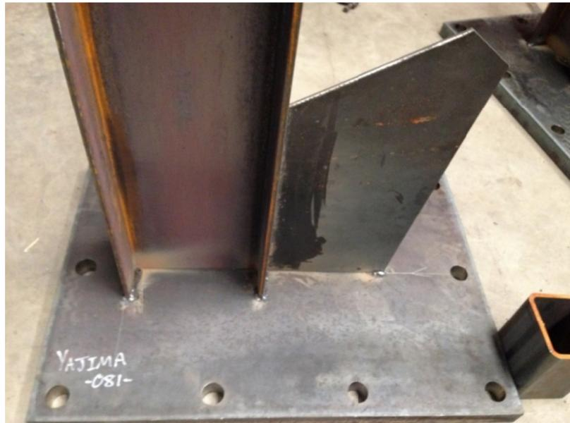
**Figure B.3** Bottom gusset plate welded to the base plate and the column flange.
