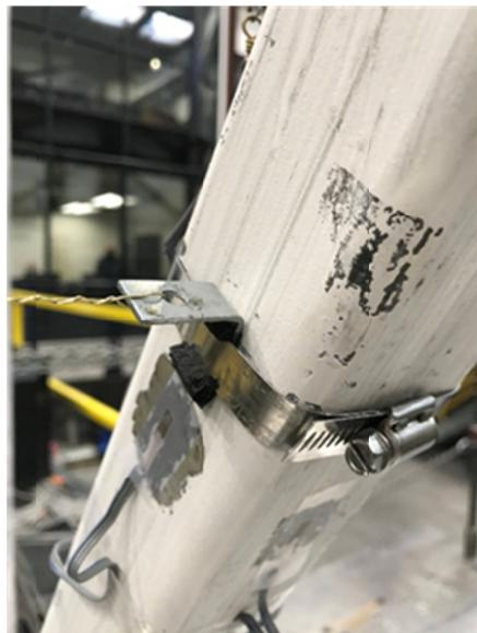
**Figure C.18** L-bracket attached to braces with wire pot attached.
