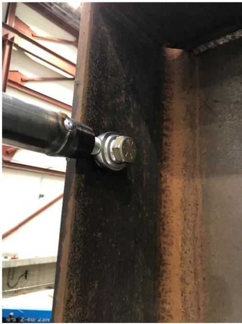
**Figure C.15** Out-of-plane restraining link attached to restraining column.
