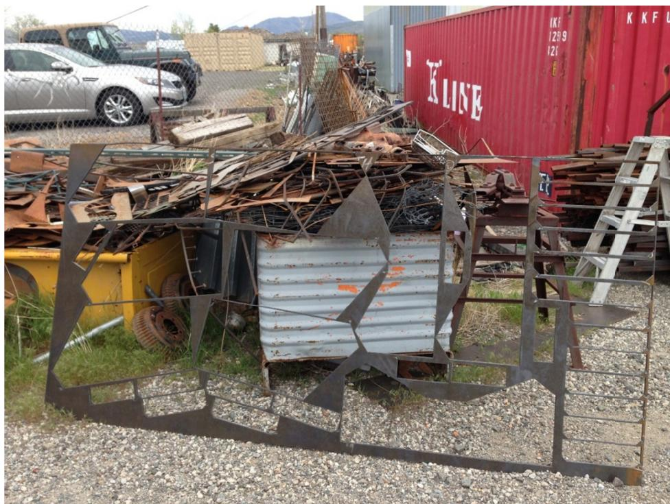
**Figure B.5** Plate after all the connecting plates where cut.
