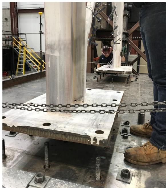
**Figure C.4** Placing specimen on the shake table.
