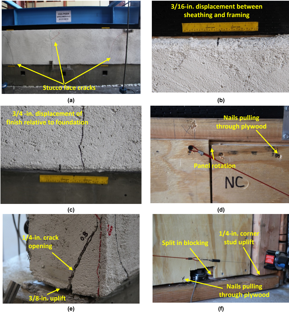
Figure 5.17 Specimen A-5 damage state at lateral strength @ +5% drift, \Delta = +1.20 in.: (a) exterior elevation; (b) top of exterior wall; (c) bottom of exterior wall; (d) close-up of plywood panel joint; (e) close-up of south-end exterior corner; and (f) bottom of south-end interior wall corner.
