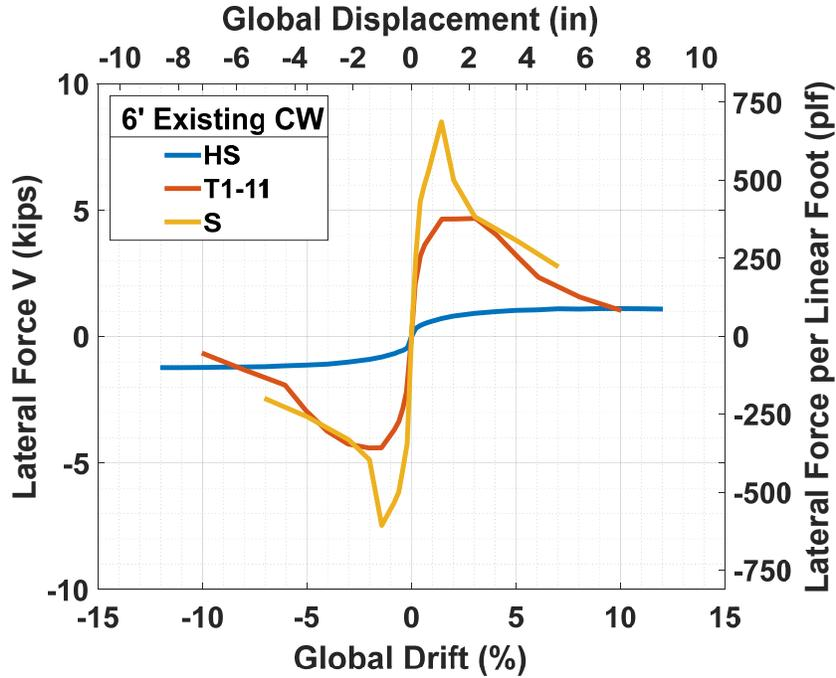
Figure 3.4 Envelope of lateral force versus *global* lateral drift and displacement hysteresis of the existing 6-ft-tall specimens with various exterior finishes.
