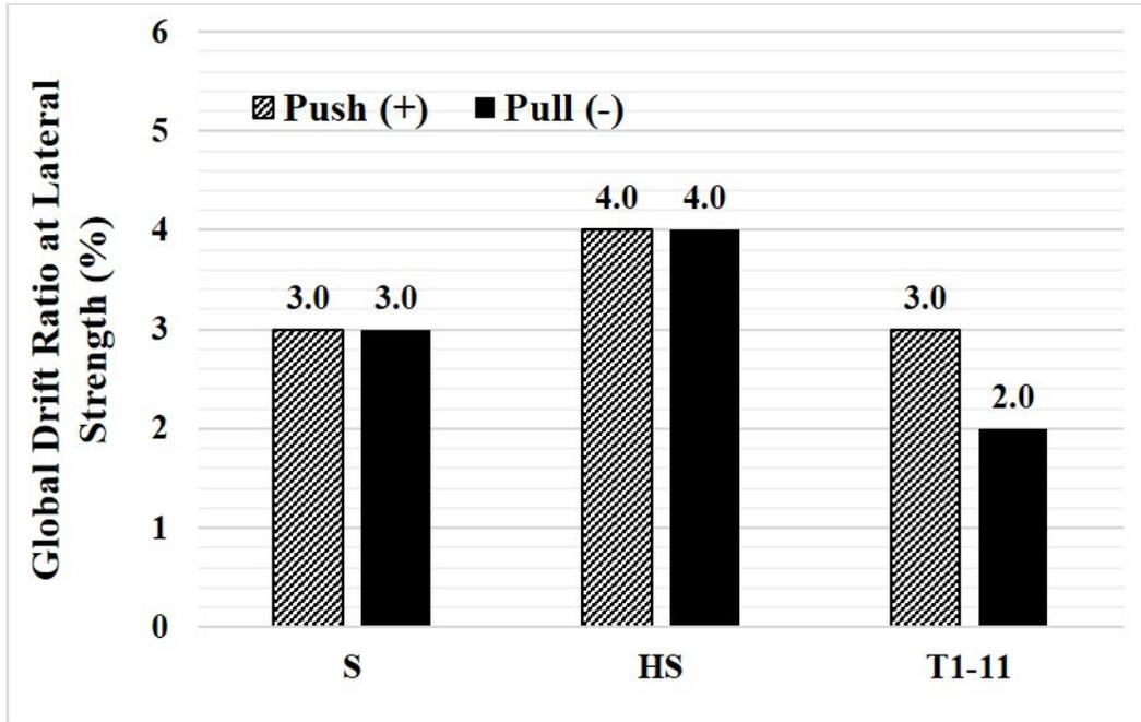
Figure 3.33 Comparison of *global* drift at strength of the retrofitted 6-ft-tall cripple walls with various exterior finishes.
