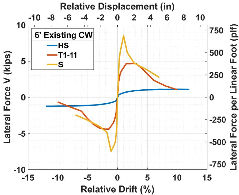
Figure 3.5 Envelope of lateral force versus *relative* lateral drift and displacement hysteresis of existing 6-ft-tall specimens with various exterior finishes.
