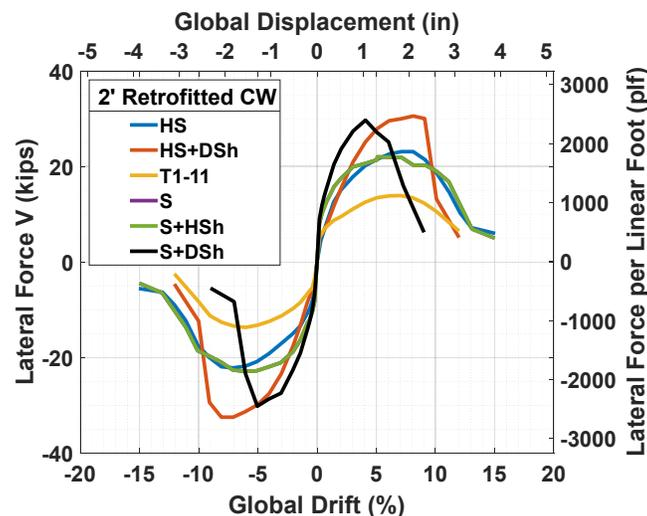
**Figure 3.7** Envelope of lateral force versus *global* lateral drift and displacement hysteresis of the retrofitted 2-ft-wall specimens with various exterior finishes.
