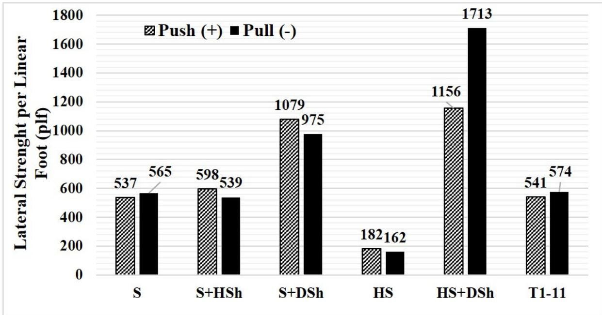
**Figure 3.3** Comparison of lateral strength per linear foot of the existing 2-ft-tall cripple walls with various exterior finishes.
