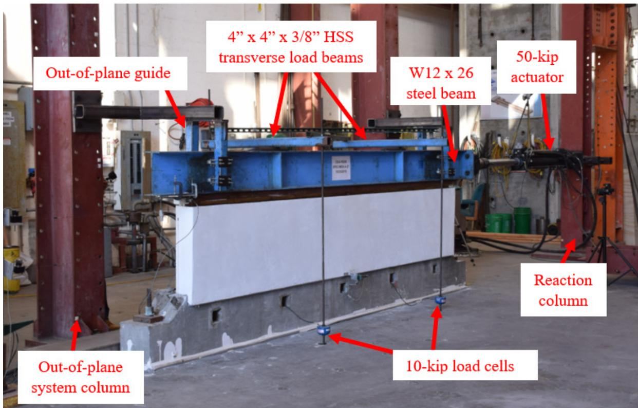
**Figure 2.2 Specimen A-27 isometric view of the test setup for 2-ft-tall cripple walls.**
