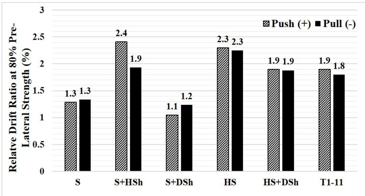
Figure 3.29 Comparison of *relative drift at 80% pre-lateral strength* of the retrofitted 2-ft-tall cripple walls with various exterior finishes.
