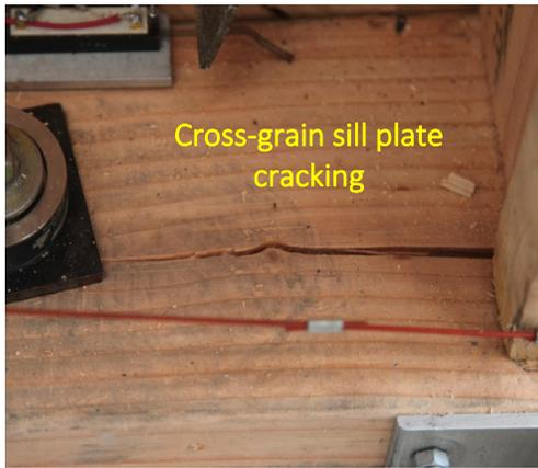
Cross-grain sill plate cracking
