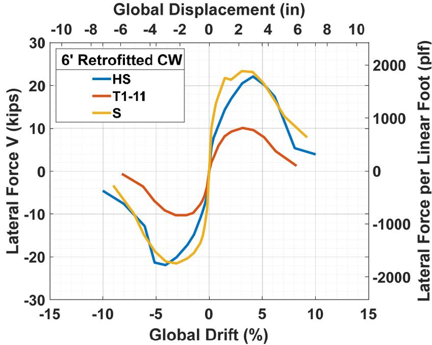
Figure 3.11 Envelope of lateral force versus *global* lateral drift and displacement hysteresis of the retrofitted 6-ft-tall specimens with various exterior finishes.
