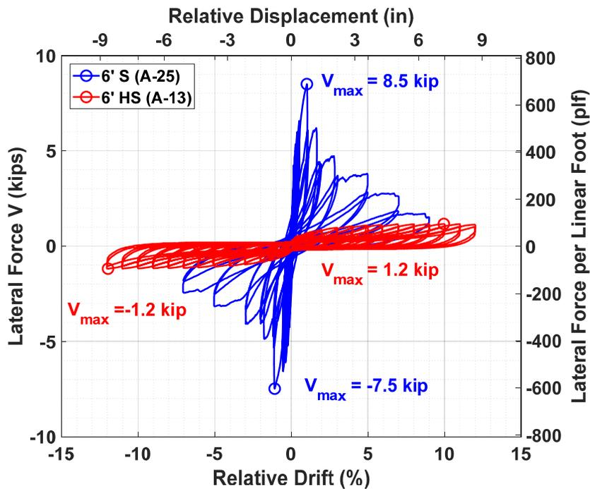
Figure 3.26 Lateral force versus relative lateral drift and displacement hysteresis of the existing 6-ft-tall specimens with stucco and horizontal siding exterior finishes.
