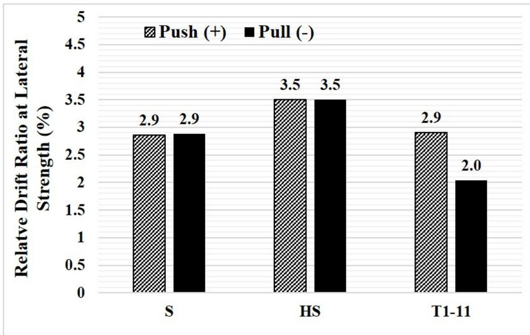
Figure 3.34 Comparison of *relative* drift at strength of the retrofitted 6-ft-tall cripple walls with various exterior finishes.
