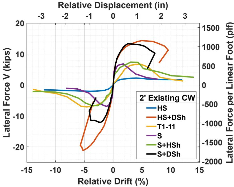
**Legend:** HS = horizontal siding; S = stucco only; HS+DSh = horizontal siding over diagonal sheathing; T1-11 = T1-11 wood structural panels; S+HSh = stucco over horizontal sheathing; S+DSh = stucco over diagonal sheathing.
