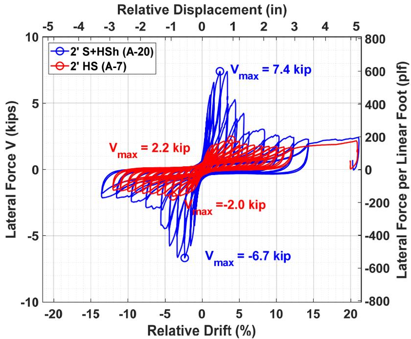
Figure 3.20 Lateral force versus relative lateral drift and displacement hysteresis of the existing 2-ft-tall specimens with stucco over horizontal sheathing and horizontal siding exterior finishes.
