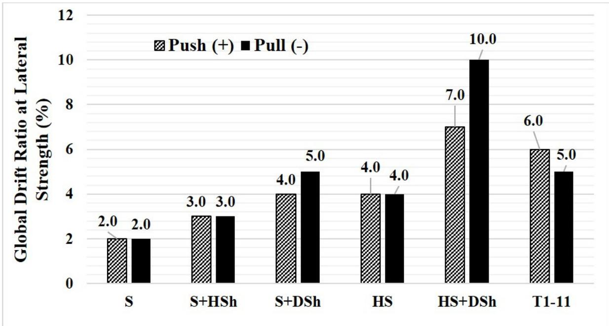
Figure 3.16 Comparison of *global* drift at strength of existing 2-ft-tall cripple walls with various exterior finishes.
