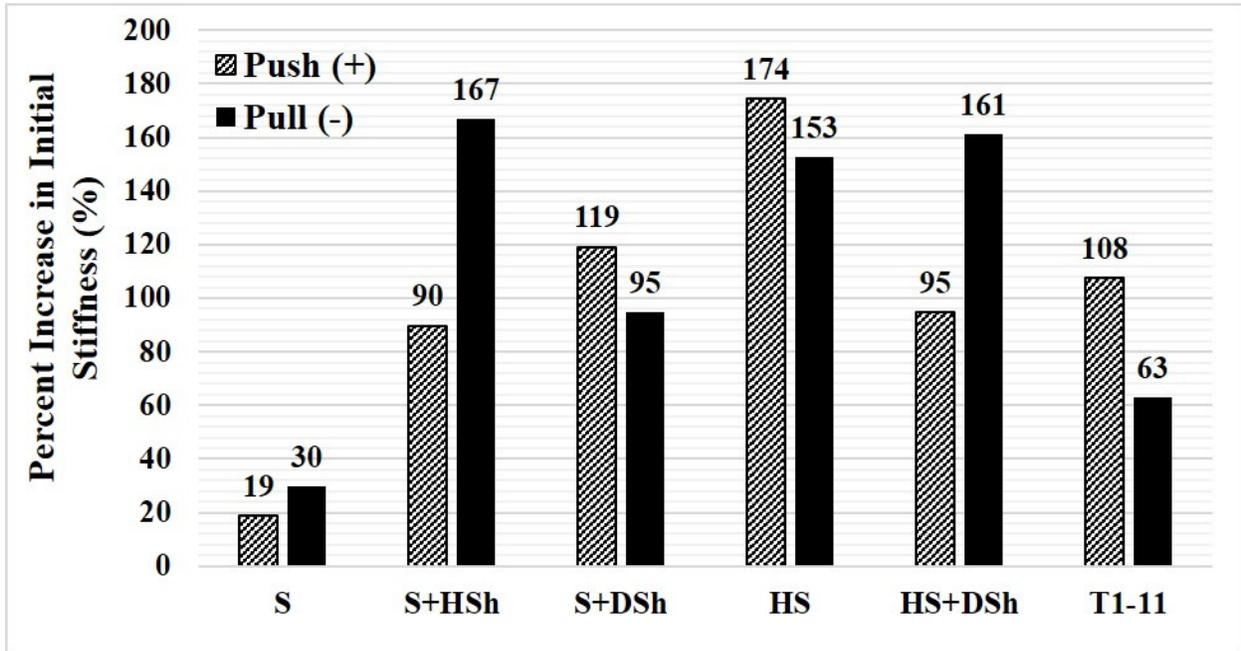
Figure 3.40 Contribution of the retrofit to initial stiffness for relative drift at 80% pre-strength for all 2-ft-tall specimens with various exterior finishes.
