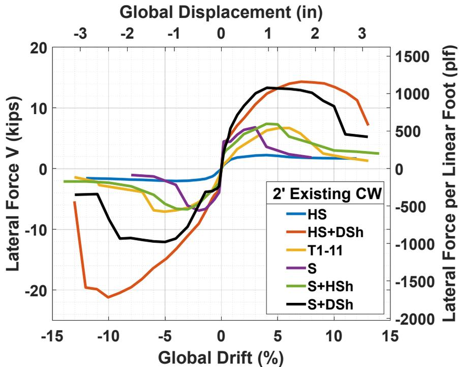
**Legend:** HS = horizontal siding; S = stucco only; HS+DSh = horizontal siding over diagonal sheathing; T1-11 = T1-11 wood structural panels; S+HSh = stucco over horizontal sheathing; S+DSh = stucco over diagonal sheathing.
