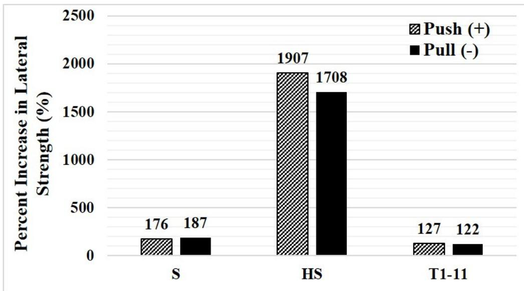
Figure 3.14 Contribution of retrofit to lateral strength for all retrofitted 6-ft-tall specimens with various exterior finishes.
