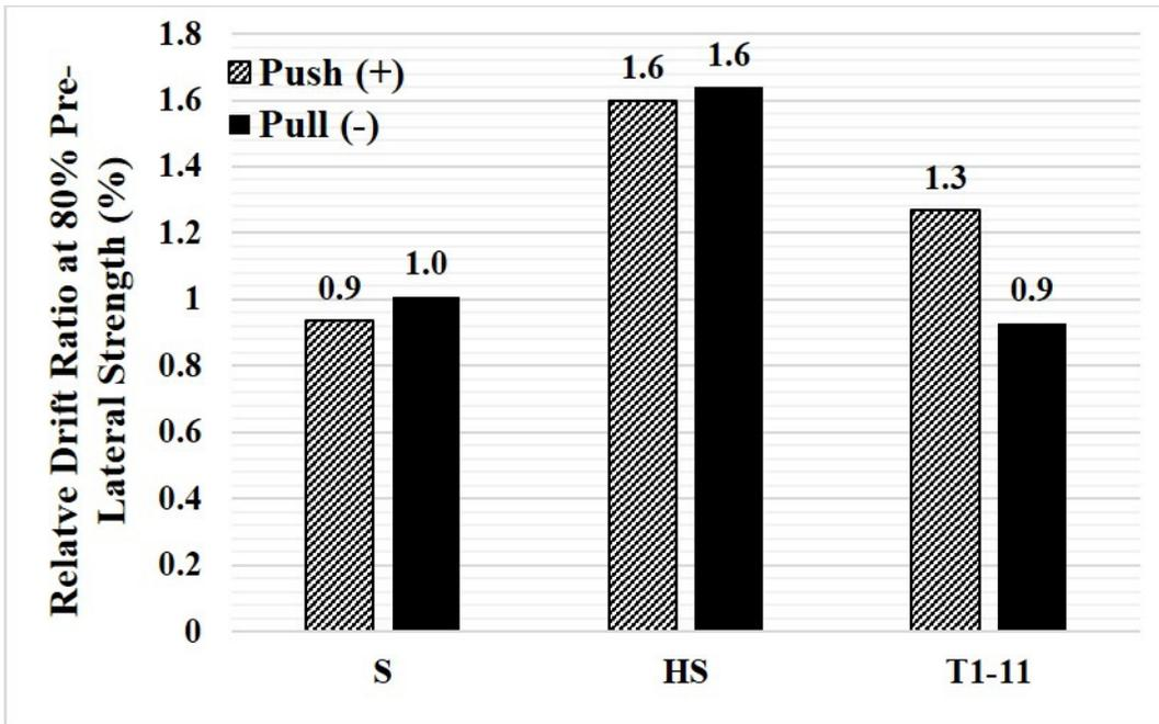
Figure 3.35 Comparison of *relative drift* at 80% pre-lateral strength of the retrofitted 6-ft-tall cripple walls with various exterior finishes.
