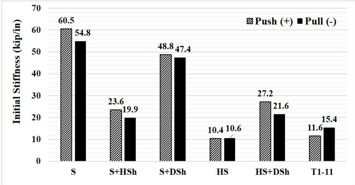
Figure 3.38 Comparison of initial stiffness for *relative drift* at 80% pre-lateral strength of existing 2-ft-tall cripple walls with various exterior finishes.
