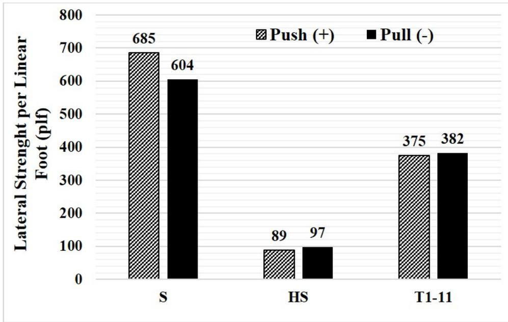
**Figure 3.6 Comparison of lateral strength per linear foot of the existing 6-ft-tall cripple walls with various exterior finishes.**
