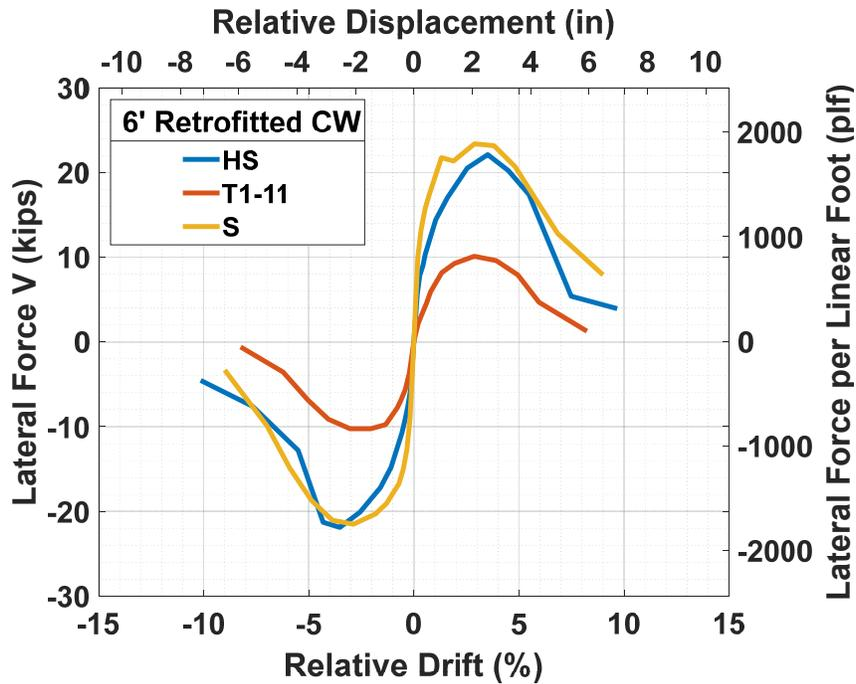
Figure 3.12 Envelope of lateral force versus *relative* lateral drift and displacement hysteresis of the retrofitted 6-ft-tall specimens with various exterior finishes.
