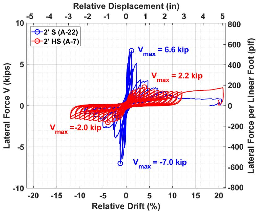
Figure 3.21 Lateral force versus relative lateral drift and displacement hysteresis of the existing 2-ft-tall specimens with stucco and horizontal siding exterior finishes.
