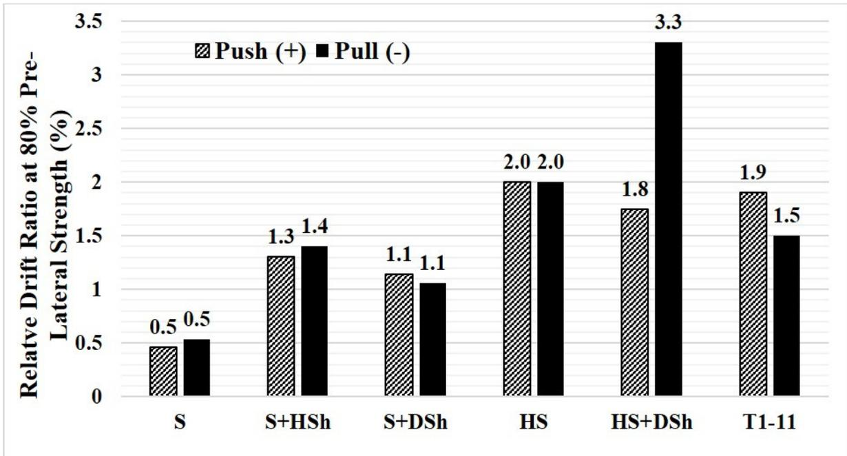
Figure 3.18 Comparison of *relative drift* at 80% pre-lateral strength of the existing 2-ft-tall cripple walls with various exterior finishes.
