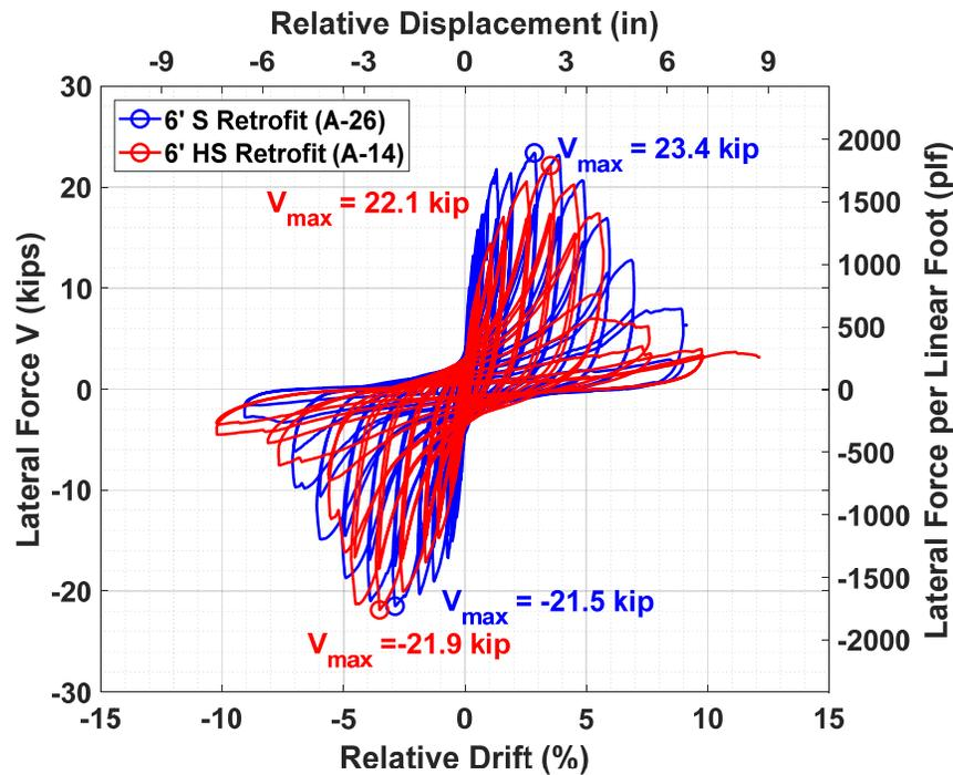
**Figure 3.37** Lateral force versus relative lateral drift and displacement hysteresis of the retrofitted 6-ft-tall specimens with stucco and horizontal siding exterior finishes.
