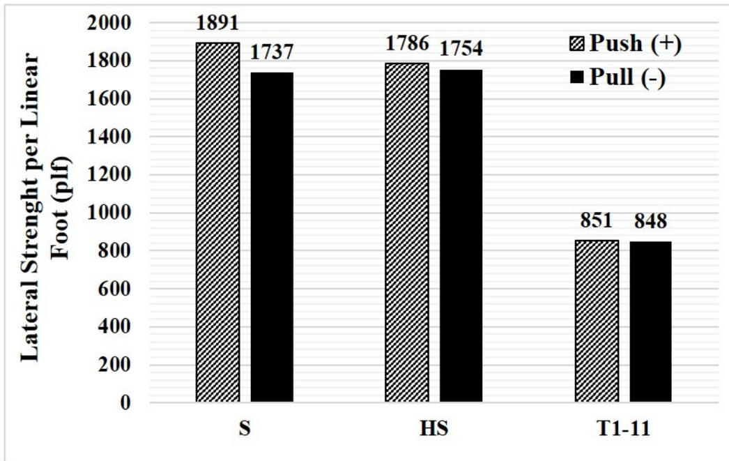
Figure 3.13 Comparison of lateral strength per linear foot of the retrofitted 6-ft-tall cripple walls with various exterior finishes.
