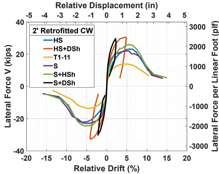
**Figure 3.8** Envelope of lateral force versus *relative* lateral drift and displacement hysteresis of the retrofitted 2-ft-wall specimens with various exterior finishes.
