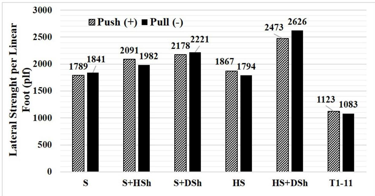
**Figure 3.9** Comparison of lateral strength per linear foot of the retrofitted 2-ft-wall cripple walls with various exterior finishes.
