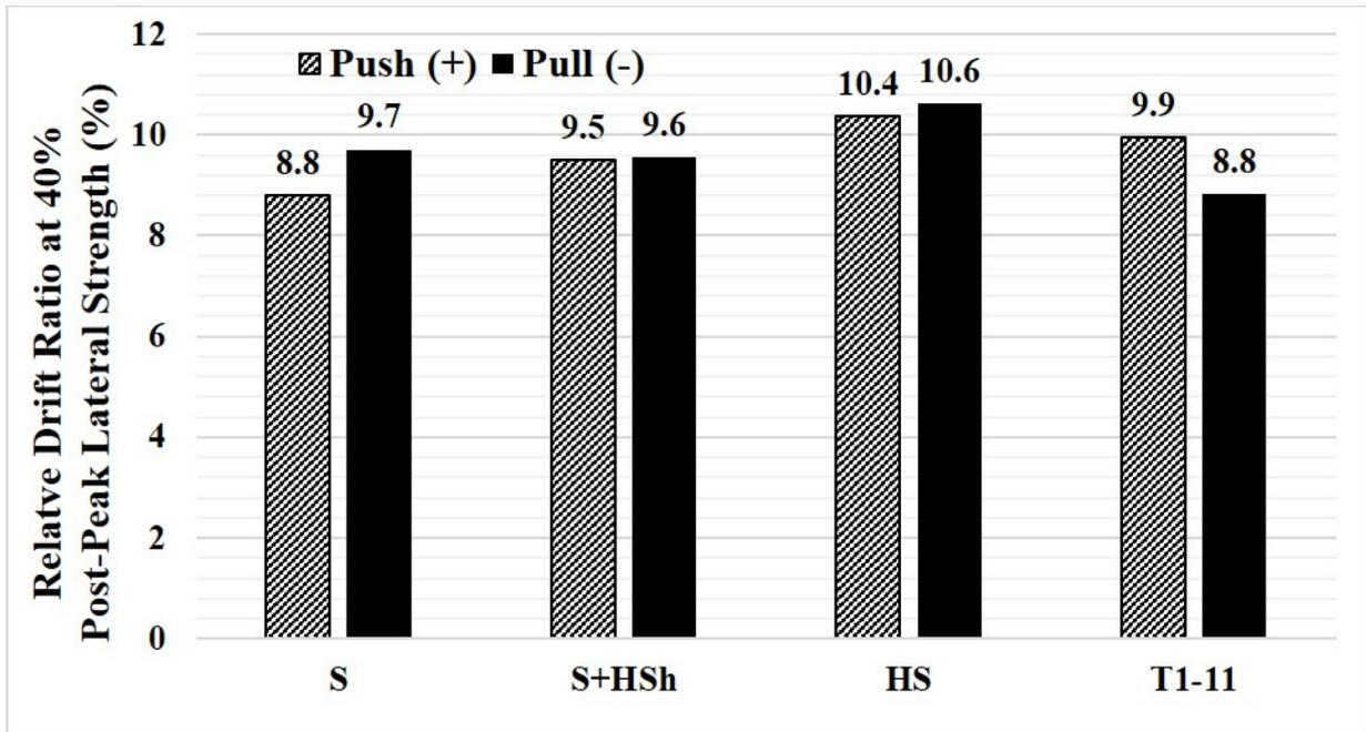
Figure 3.30 Comparison of *relative drift* at 40% post-peak strength of the retrofitted 2-ft-tall cripple walls with various exterior finishes.
