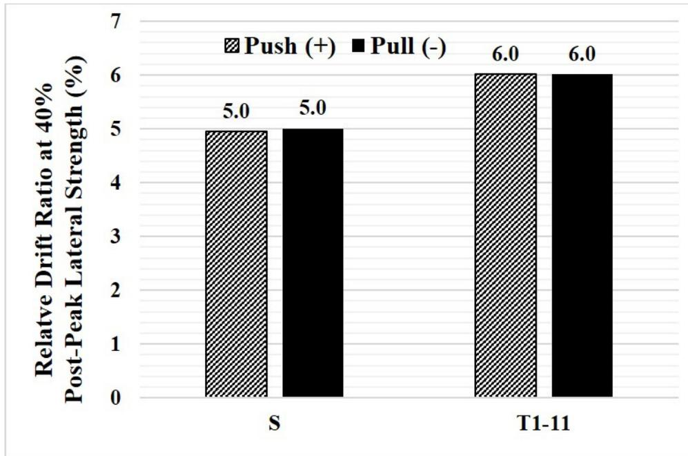
Figure 3.25 Comparison of *relative drift* at 40% post-peak strength of the existing 6-ft-tall cripple walls with various exterior finishes.
