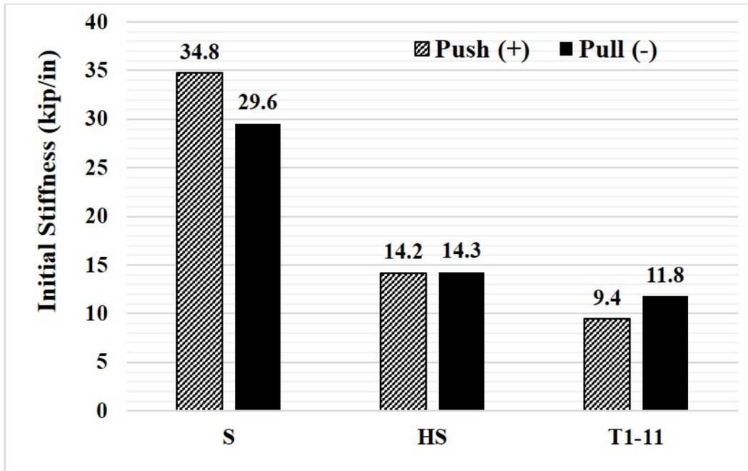
Figure 3.43 Comparison of initial stiffness for *relative drift* at 80% pre-lateral strength of the retrofitted 6-ft-tall cripple walls with various exterior finishes.
