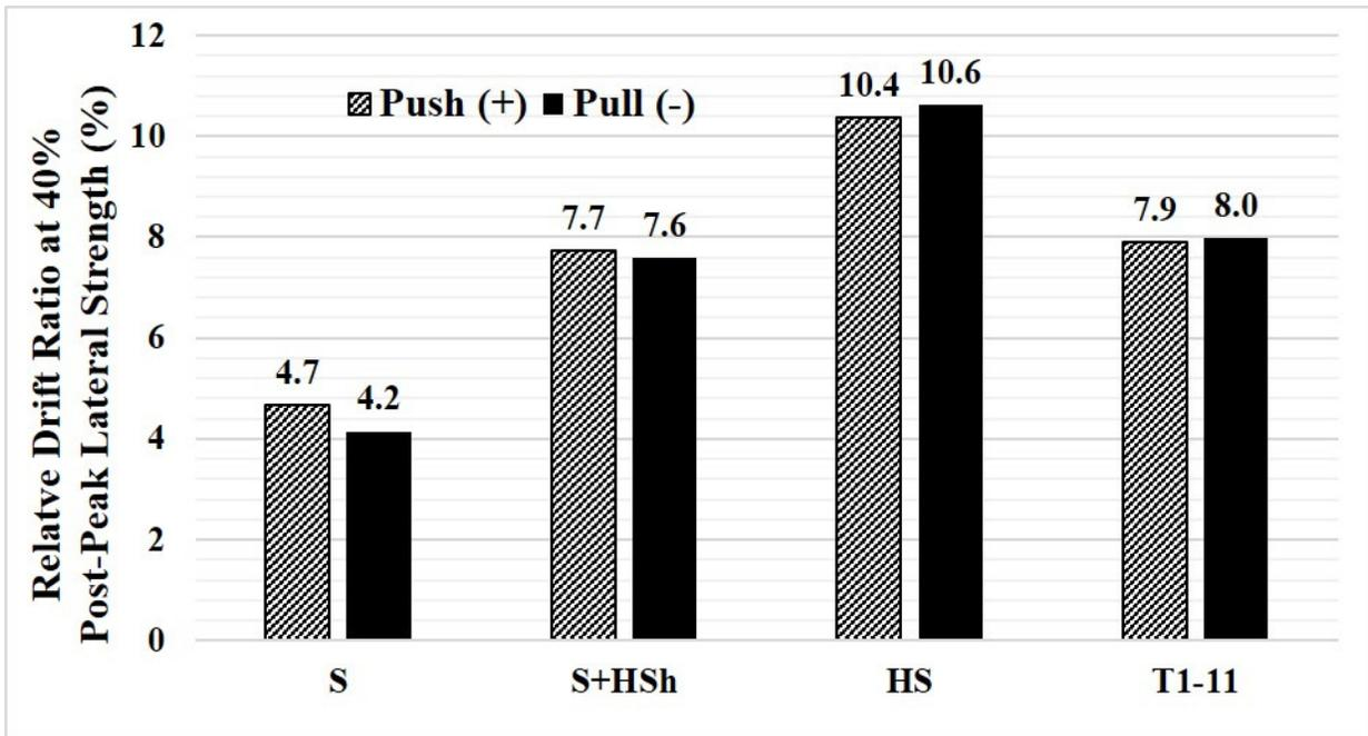
Figure 3.19 Comparison of *relative drift* at 40% post-peak strength of the existing 2-ft-tall cripple walls with various exterior finishes.
