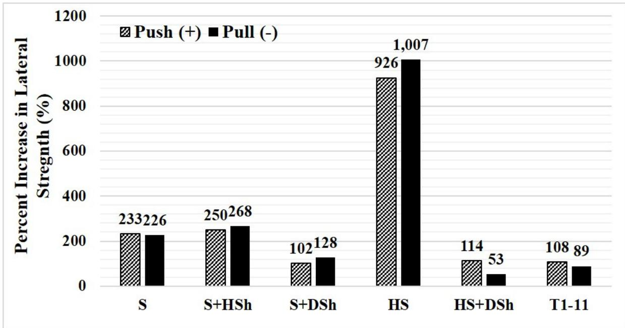
**Figure 3.10 Contribution of retrofit to lateral strength for all retrofitted 2-ft-wall specimens with various exterior finishes.**
