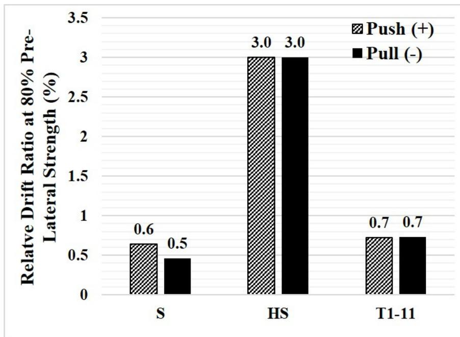
Figure 3.24 Comparison of *relative drift at 80% pre-lateral strength* of the existing 6-ft-tall cripple walls with various exterior finishes.
