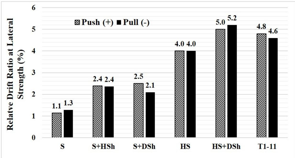
Figure 3.17 Comparison of *relative* drift at strength of existing 2-ft-tall cripple walls with various exterior finishes.
