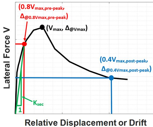
Figure 3.15 Schematic defining key parameters compared amongst specimens in report: initial stiffness  $K_{sec}$ , drift at strength (drift capacity), relative drift at 80% lateral strength (pre-strength), and relative drift at 40% lateral strength (post-strength) from an envelope of the response.
