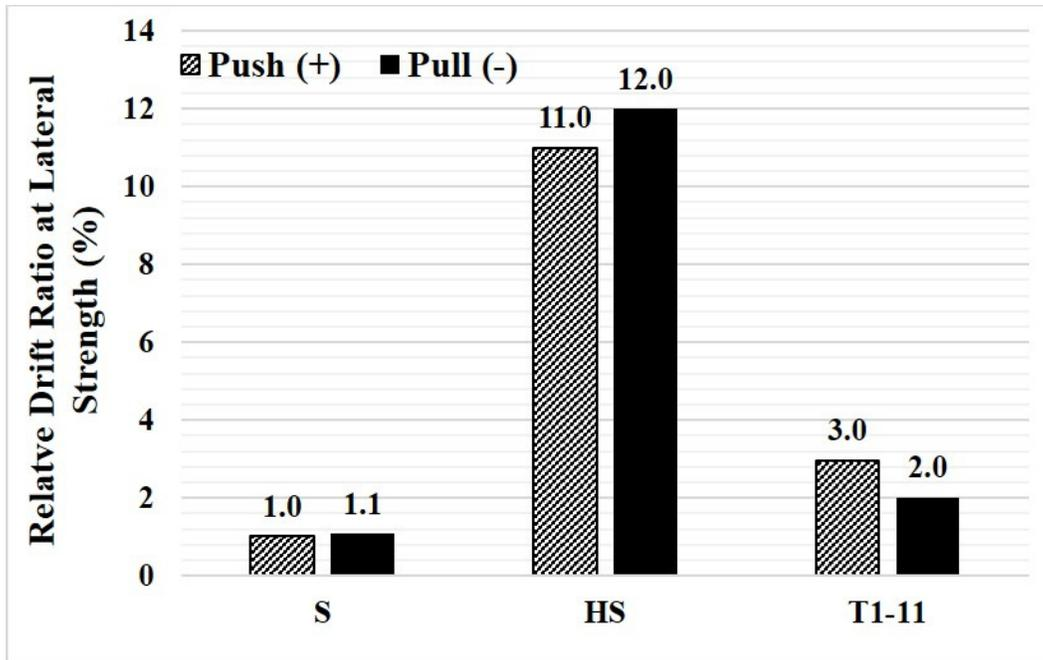
Figure 3.23 Comparison of *relative drift at strength* of the existing 6-ft-tall cripple walls with various exterior finishes.
