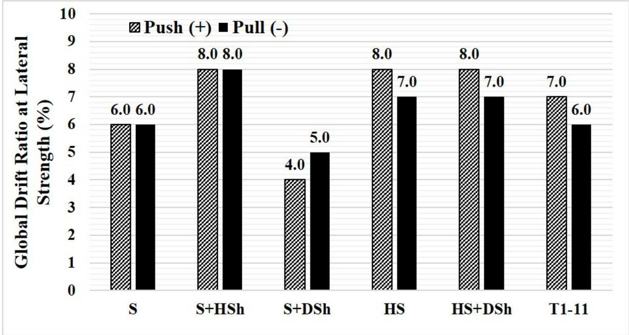
**Figure 3.27 Comparison of global drift at strength of the retrofitted 2-ft-tall cripple walls with various exterior finishes.**
