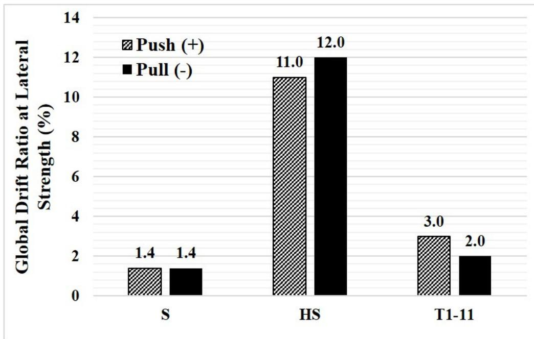
Figure 3.22 Comparison of *global* drift at strength of the existing 6-ft-tall cripple walls with various exterior finishes.
