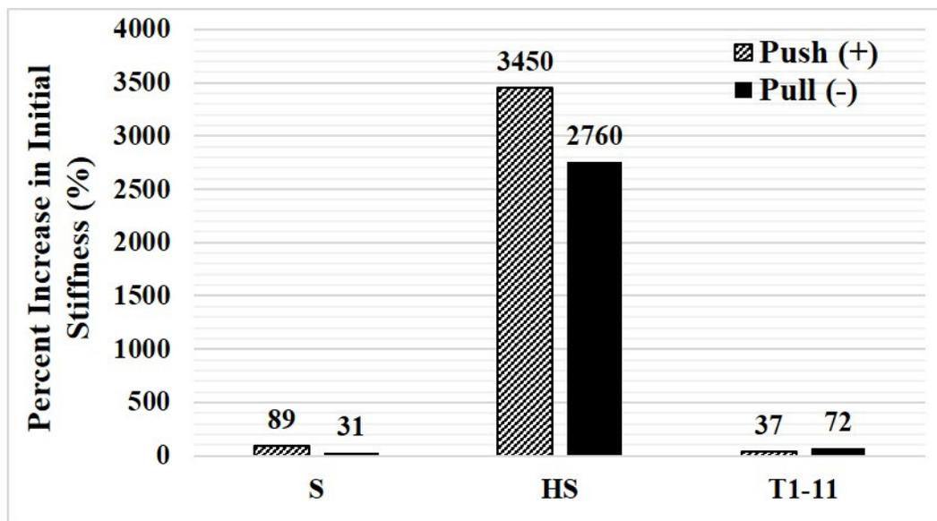
Figure 3.42 Contribution of the retrofit to initial stiffness for relative drift at 80% pre-strength for all 6-ft-tall specimens with various exterior finishes.
