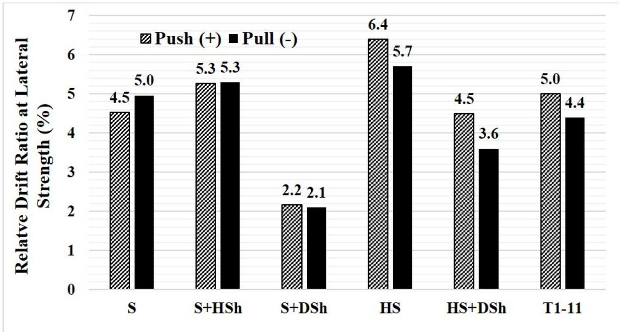
Figure 3.28 Comparison of *relative drift at strength* of the retrofitted 2-ft-tall cripple walls with various exterior finishes.
