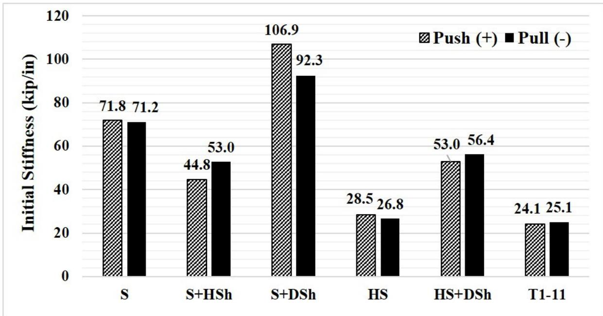
Figure 3.41 Contribution of the retrofit to initial stiffness for relative drift at 80% pre-strength for all 2-ft-tall specimens with various exterior finishes.
