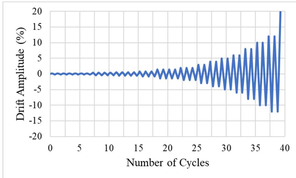
**Figure 2.3 Loading protocol for Specimen A-7 (2-ft-tall specimen).**
