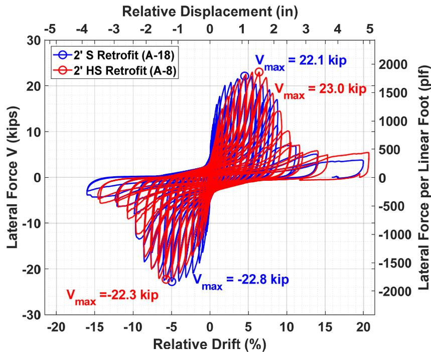
Figure 3.31 Lateral force versus relative lateral drift and displacement hysteresis of the retrofitted 2-ft-tall specimens with stucco and horizontal siding exterior finishes.
