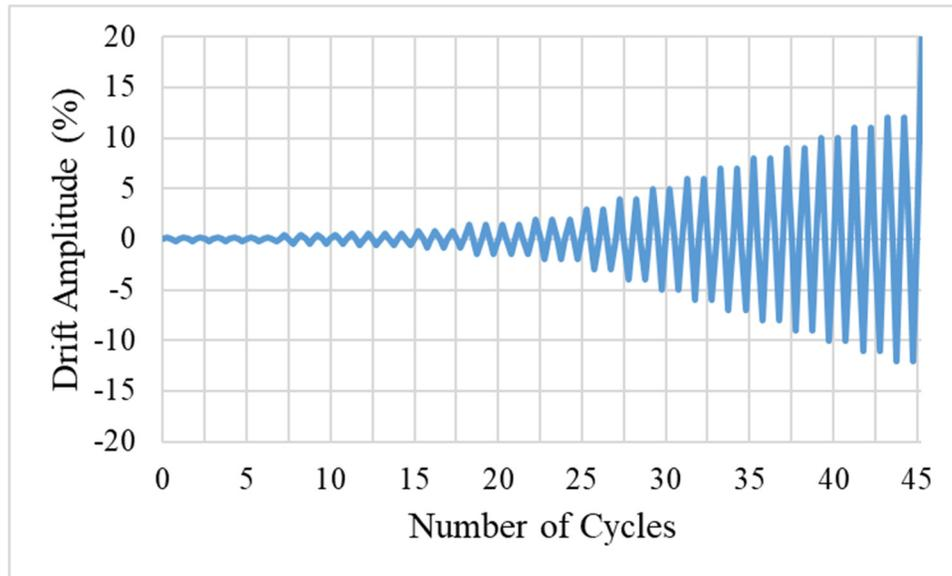
Figure 2.4 Loading protocol for Specimen A-13 (6-ft-tall specimen).
