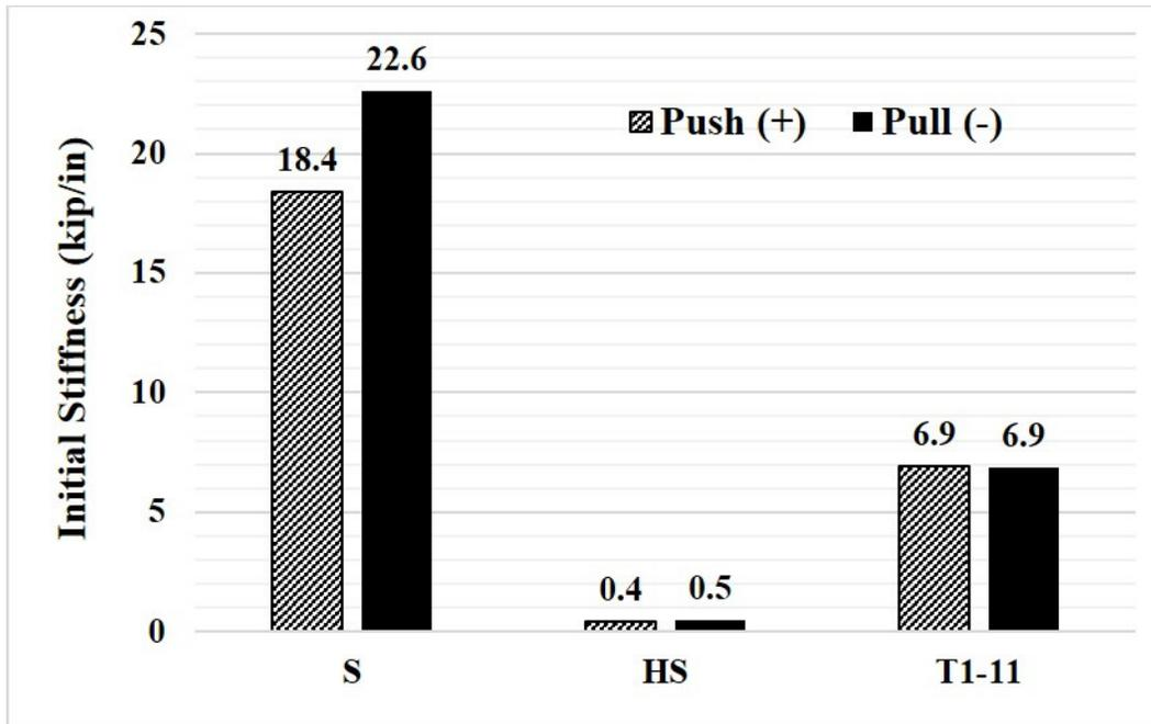
Figure 3.39 Comparison of initial stiffness for *relative drift* at 80% pre-lateral strength of existing 6-ft-tall cripple walls with various exterior finishes.
