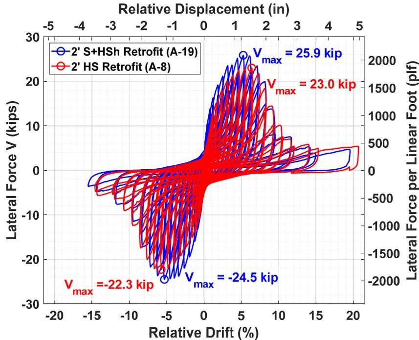
**Figure 3.32** Lateral force versus relative lateral drift and displacement hysteresis of the retrofitted 2-ft-tall specimens with stucco over horizontal sheathing and horizontal siding exterior finishes.
