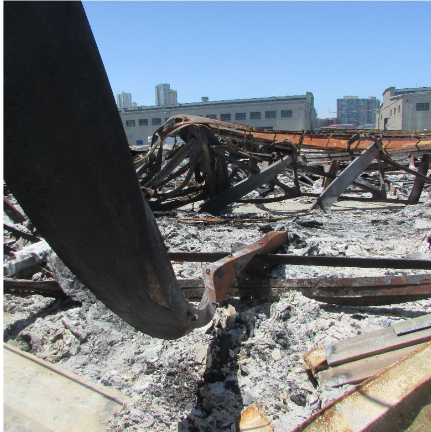
Figure 4.10: Significant out-of-plane deformation in collapsed beams.
