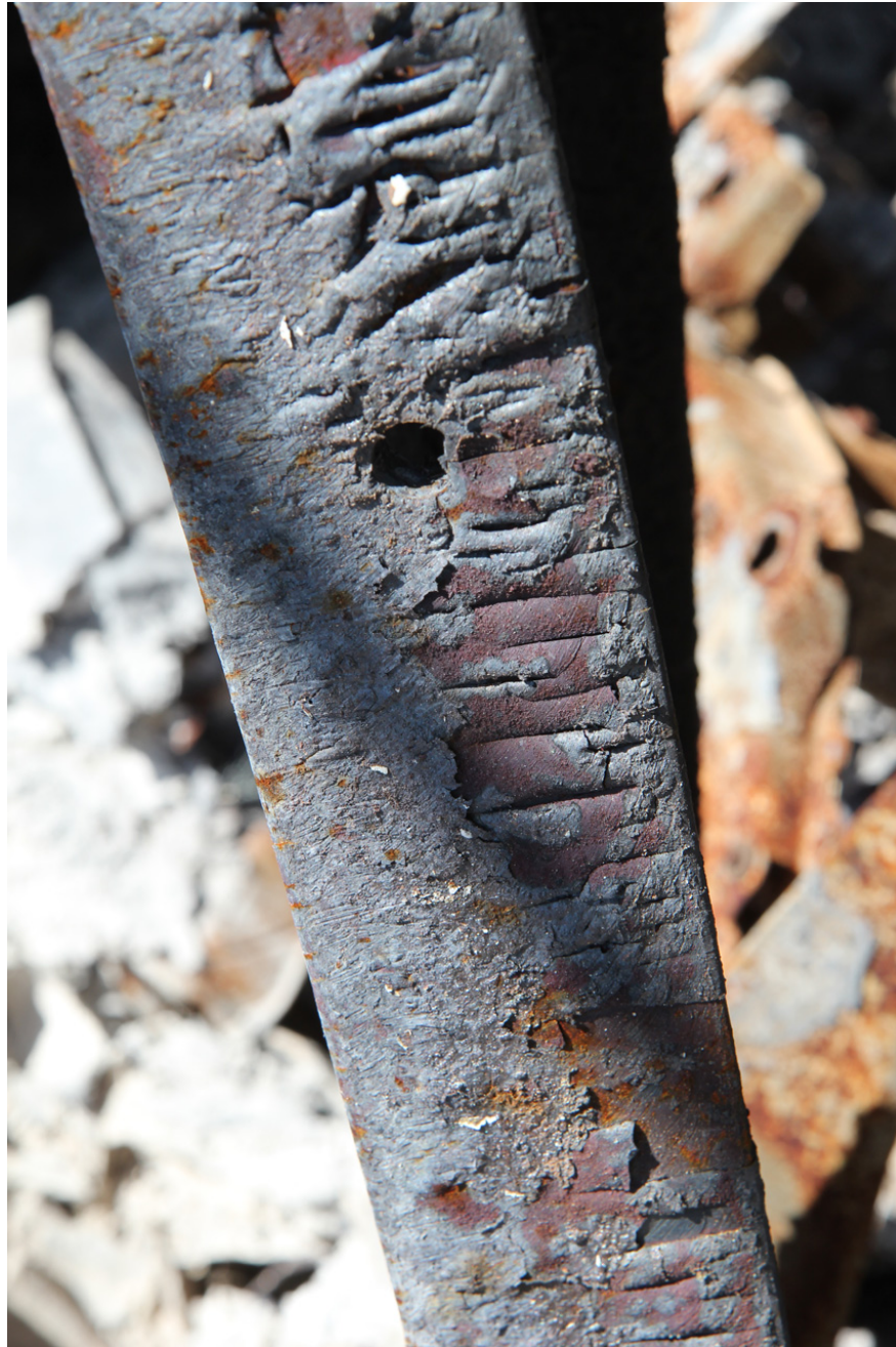
Figure A.28: Signs of heat-induced material flow in the compression flange of the steel beam.
