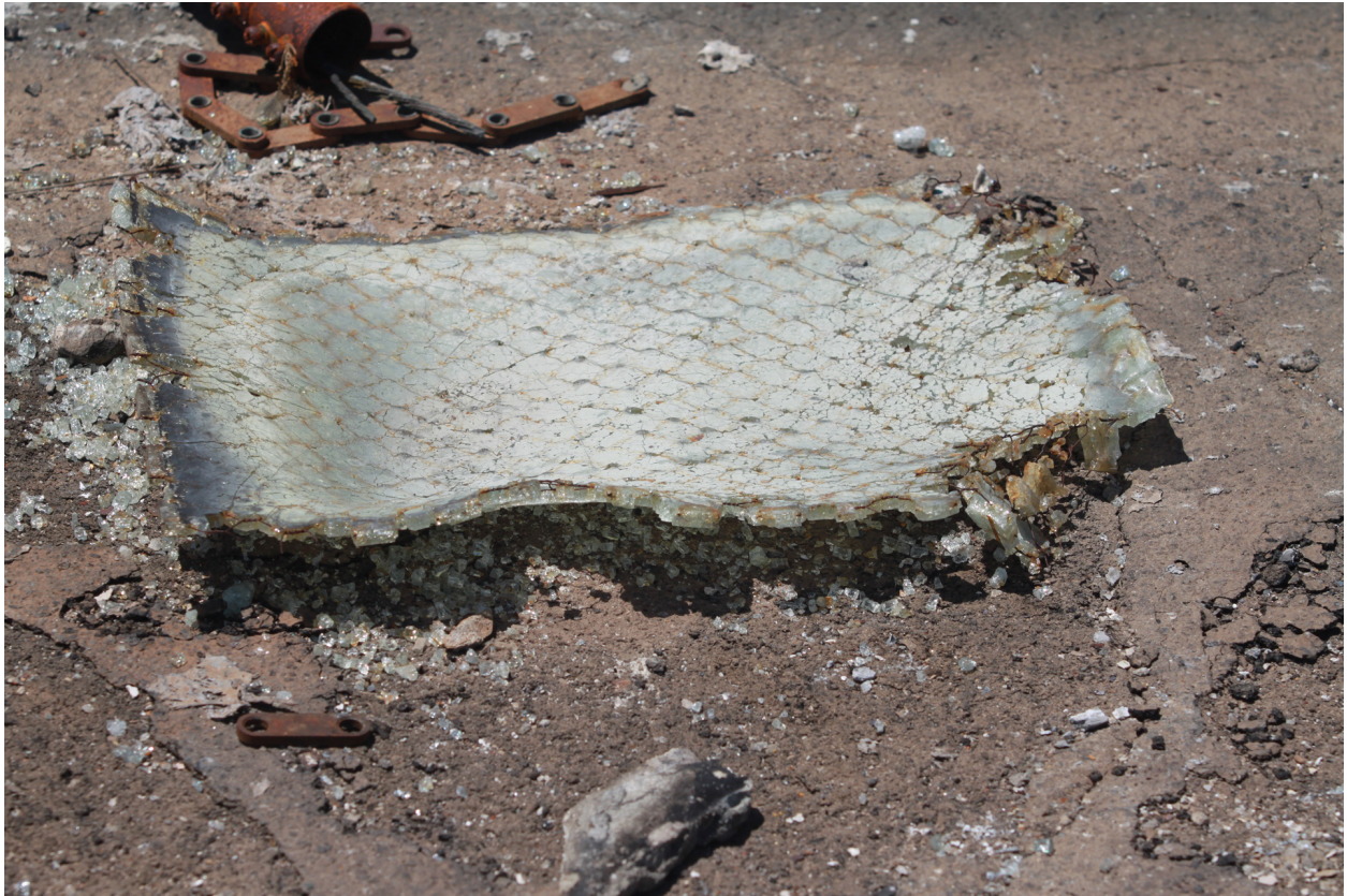
Figure 4.22: Deformed glass in east side of the structure.
