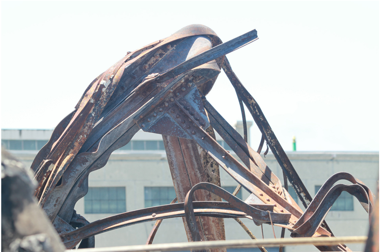
Figure A.32: Intact gusset plate and connection between twisted steel members.
