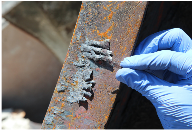
Figure 4.15: Mill-scale and material-flow patterns had formed on the outer surfaces of a truss member.
