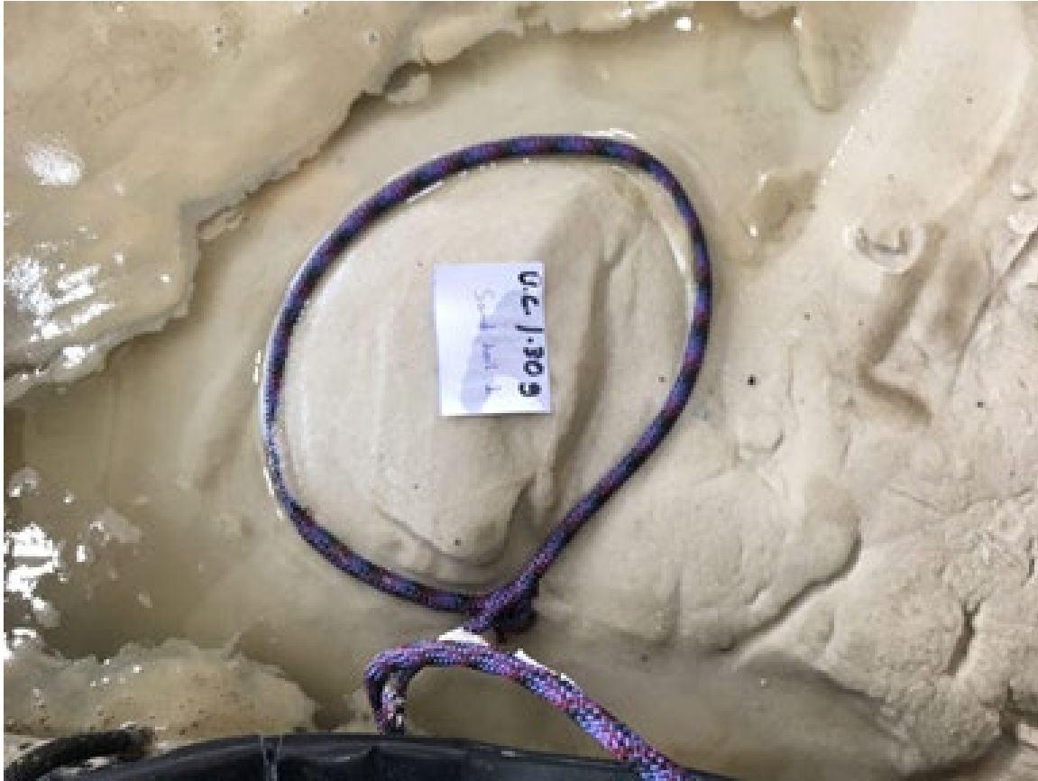
Figure 3.6 Observed sand ejecta after Shake 1-1 (Baseline test).
