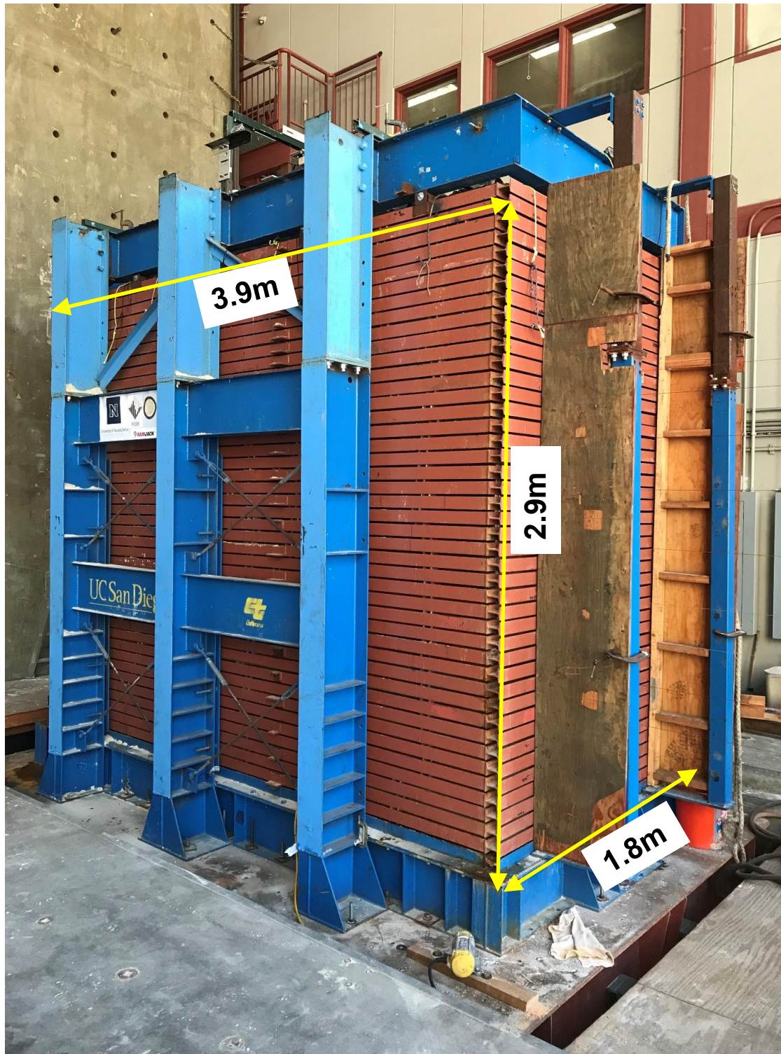
Figure 2.1 Shake table facility and laminar soil box at UC San Diego's Powell Laboratory.
