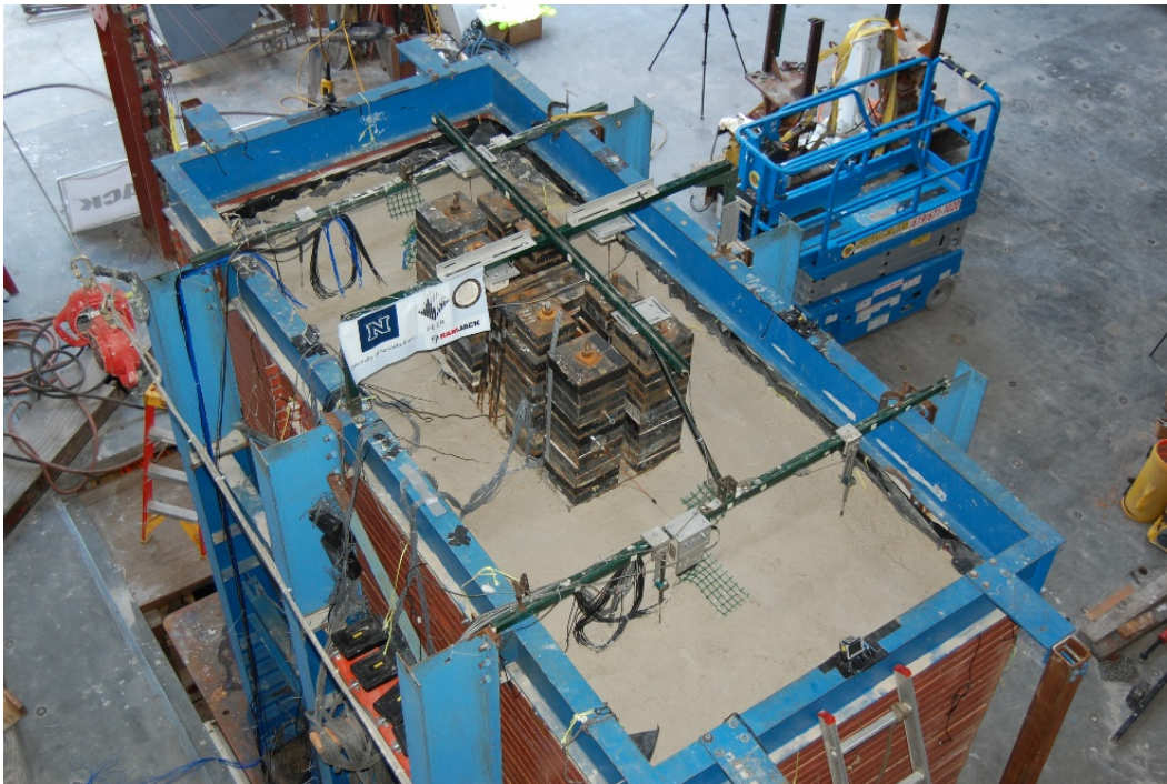
Figure 2.11 Model shallow foundation and superstructure weights in Helical Pile test.
