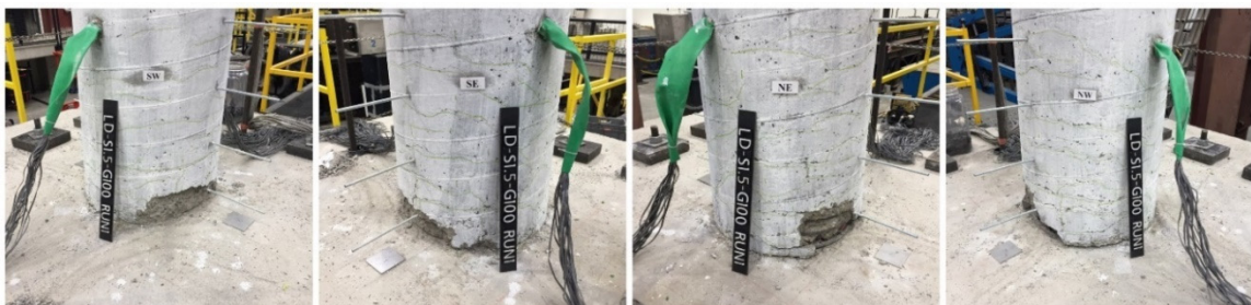
Figure 5.4 Column LD-S3-G100: progression of damage after the first run.
