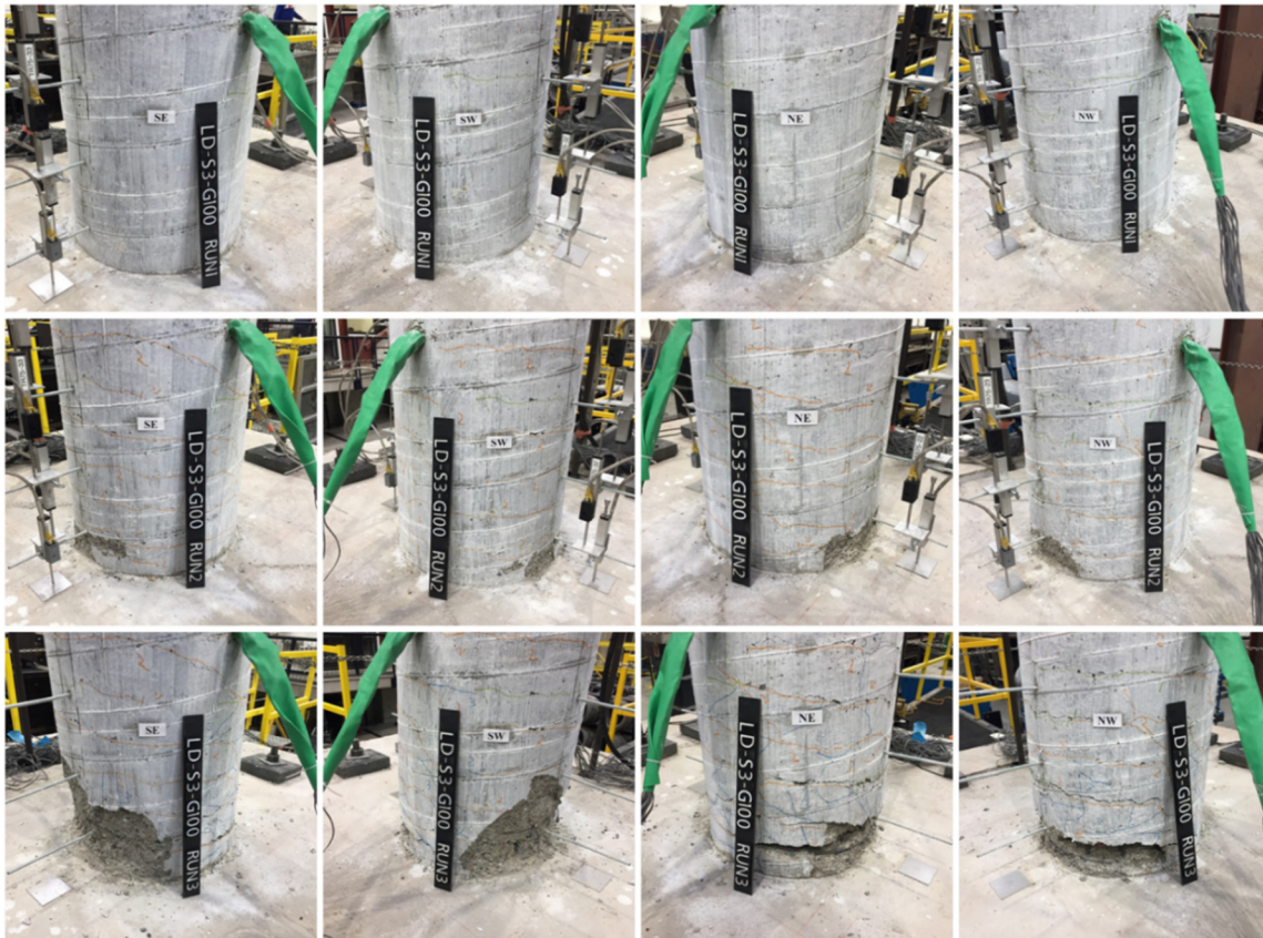
Figure 5.6 Column LD-S3-G100: progression of damage after each run.
