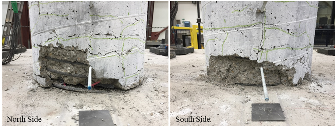
Figure 5.7 Column LD-S1.5-G100: final damage state.
