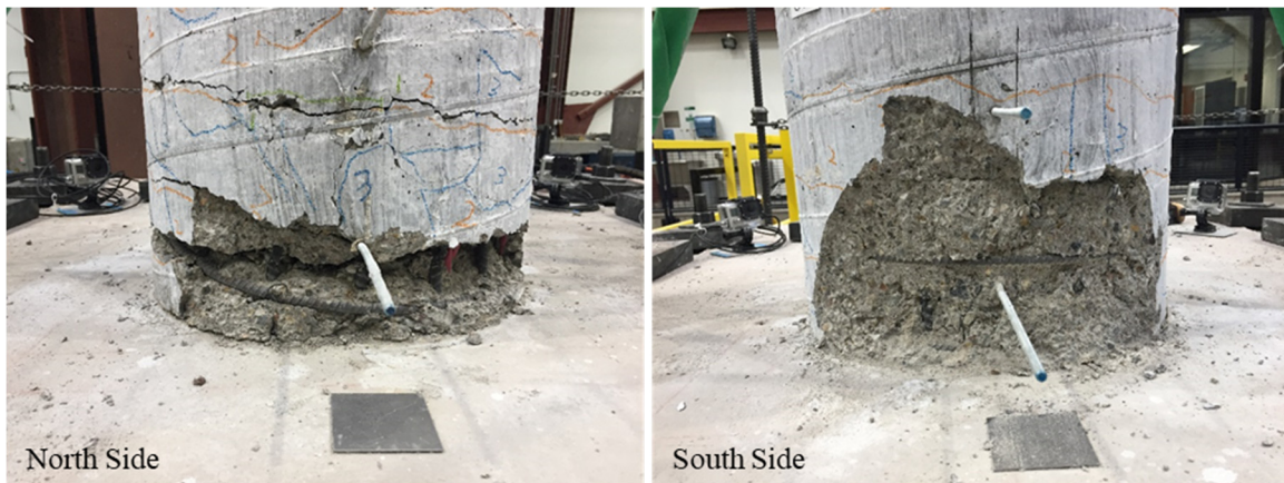
Figure 5.9 Column LD-S3-G100: final damage state.
