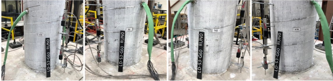
Figure 4.1 Column LD-S3-G60 before starting the test.
