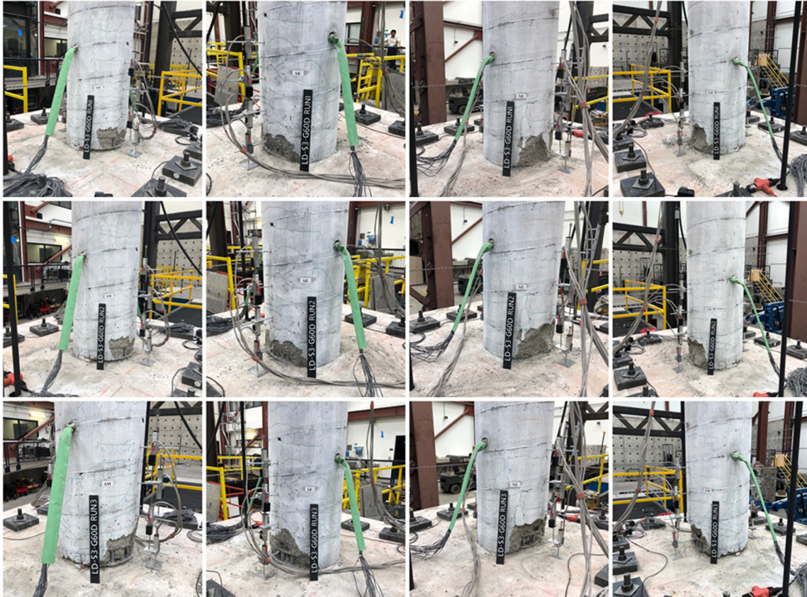
Figure 4.6 Column LD-S3-G60D: progression of damage after each run.
