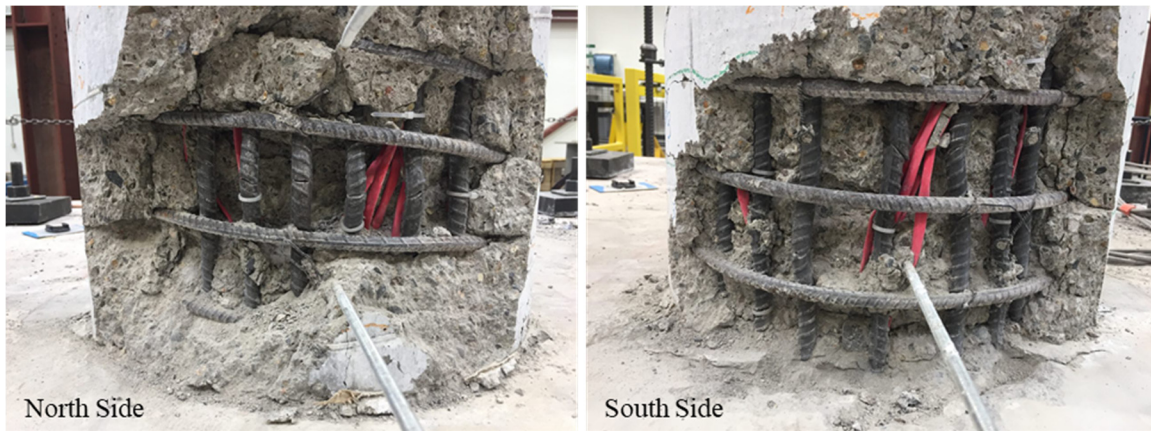
Figure 4.7 Column LD-S3-G60: final damage state.
