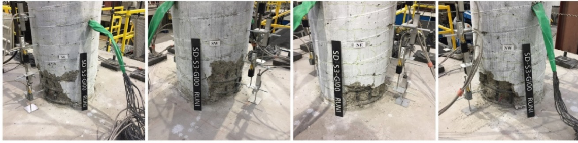
Figure 5.5 Column SD-S1.5-G100: progression of damage after the first run.
