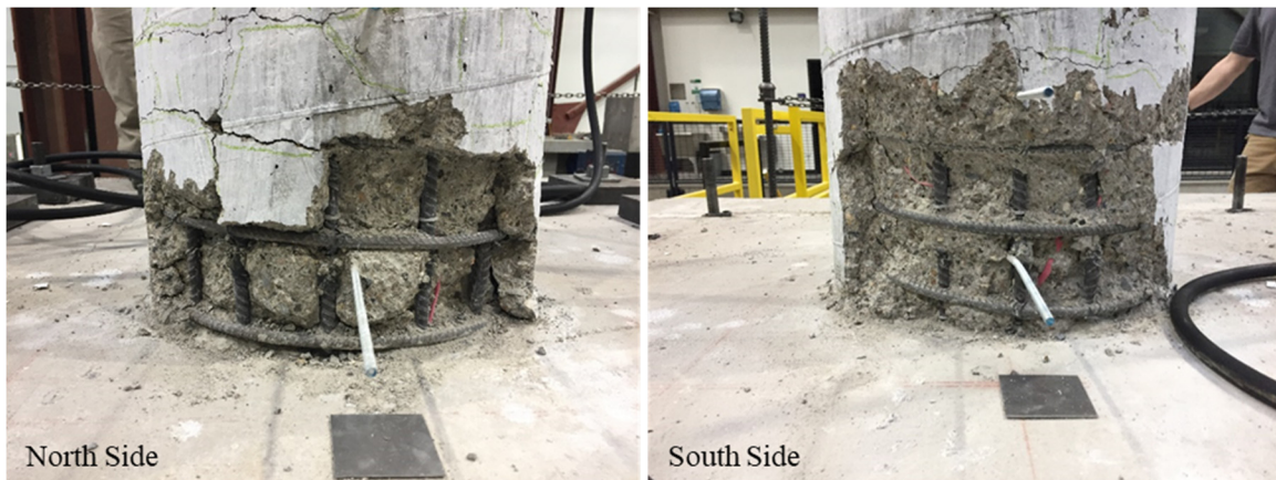
Figure 5.8 Column SD-S3-G100: final damage state.
