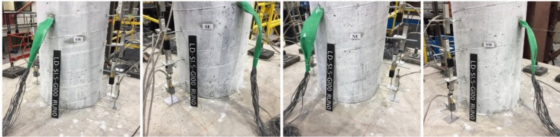
Figure 5.1 Column LD-S1.5-G100 before starting the test.
