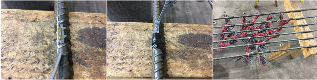
Figure 3.8 Steps of attaching strain gauges on the reinforcing bars.
