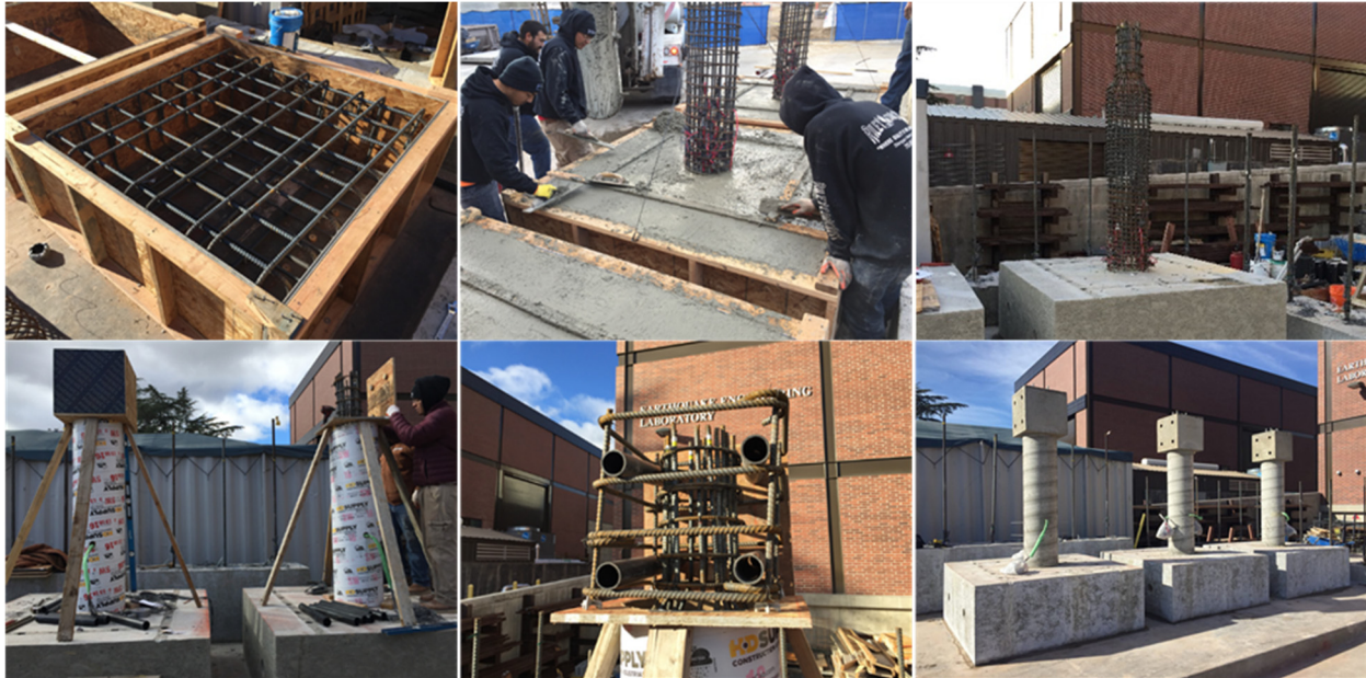
Figure 3.2 Phase I: construction stages of the specimens.
