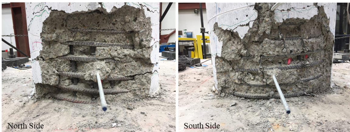
Figure 4.8 Column LD-S1.5-G60: final damage state.
