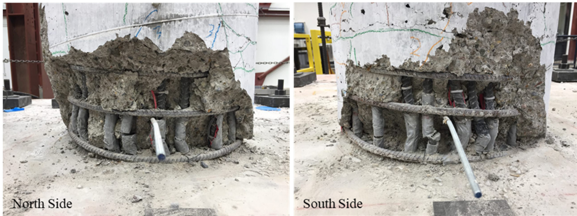
Figure 4.9 Column LD-S3-G60D: final damage state.
