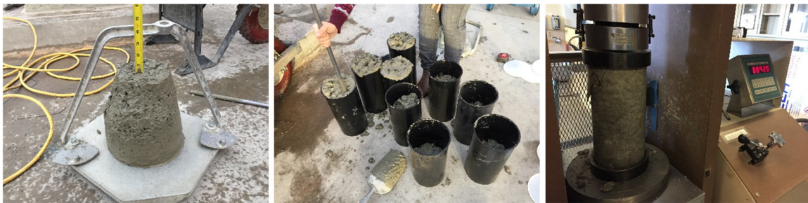
Figure 3.5 Photos of slump test, taking concrete samples, and a typical concrete cylinder compressive test.
