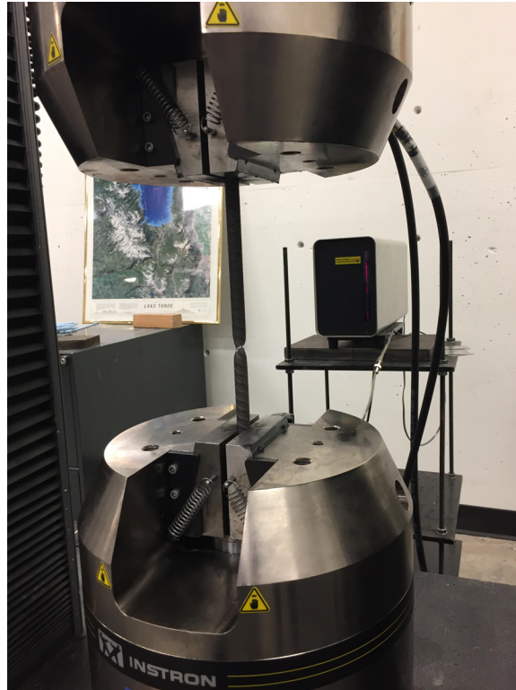
Figure 3.3 Reinforcing bar tensile test setup.
