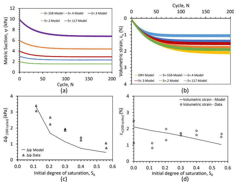
Typical results from the new model: (a) Evolution in matric suction during cyclic shearing; (b) Evolution in volumetric strain or seismic compression during cyclic shearing; (c) Predicted and measured trends in matric suction after 200 cycles of shearing; (d) Predicted and measured trends in volumetric strain or seismic compression after 200 cycles of shearing
