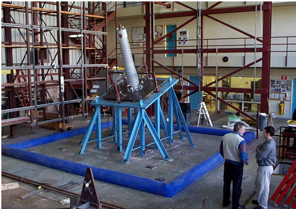
Figure 7-2 230 kV-bushing installed atop the flexible plate
