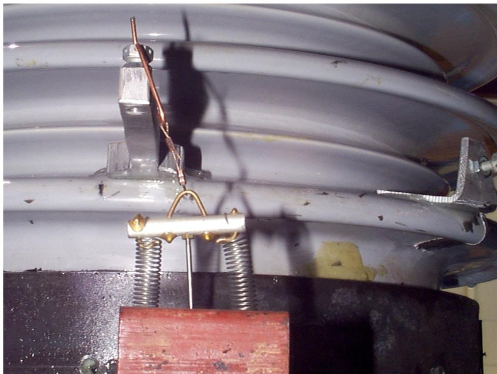
Figure 6-21 Twist of the UPPER-1 porcelain unit over the flange, Test Set 13
