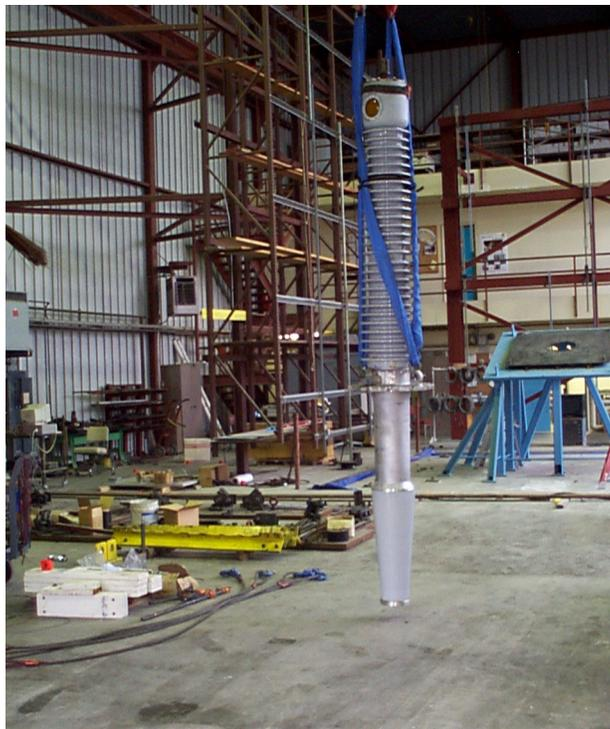
Figure 2-3 Bushing-2 prior to testing on the Berkeley simulator
