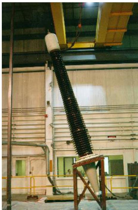
Figure 1-4 Seismic testing of a 500-kV bushing (Courtesy of CERL, Ill)
