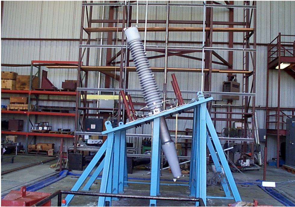
Figure 4-1 A rigidly mounted 230-kV bushing on the earthquake simulator
