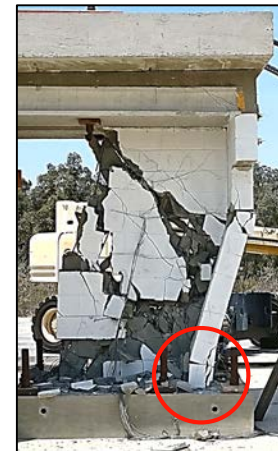
Wall damage in the test
