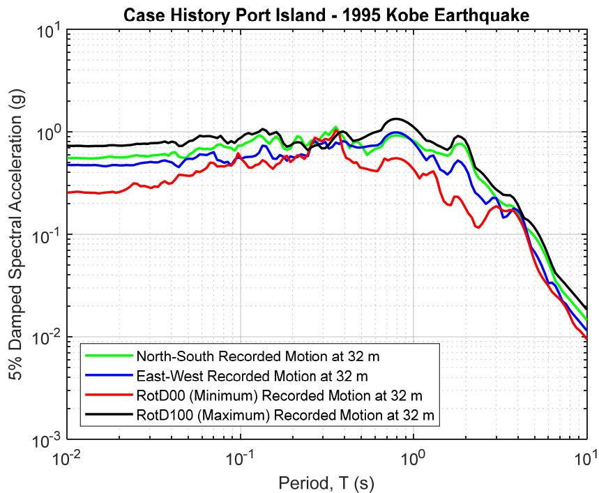
**Figure B44.1 5% Damped Response Spectra of input ground motion for Port Island**
