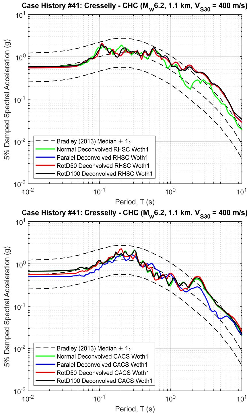
**Figure B41.1 5% Damped Response Spectra of RHSC and CACS Deconvolved Input Motion at Riccarton Gravel (multiplied by the scaling factor to represent the  $R_{rup}$  and  $V_{S30}$  of studied site)**
