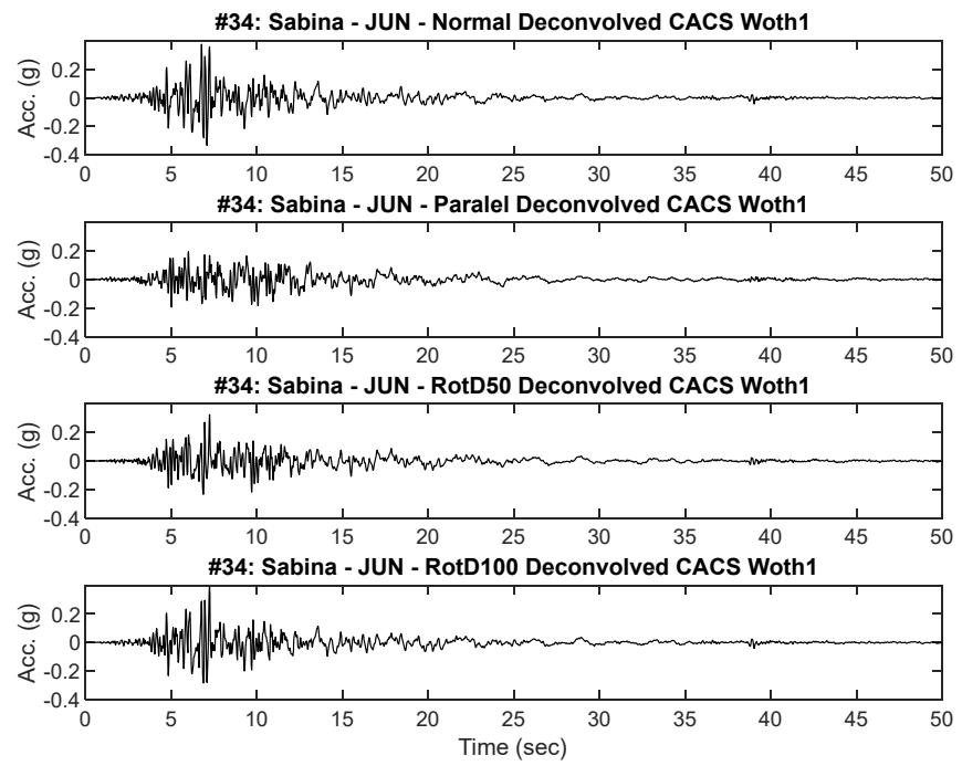
**Figure B34.2 Scaled RHSC and CACS Deconvolved input motion acceleration time history placed at Riccarton Gravel elevation for dynamic analysis**
