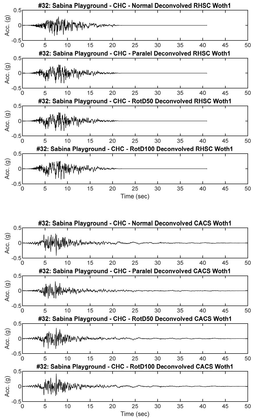
**Figure B32.2 Scaled RHSC and CACS Deconvolved input motion acceleration time history placed at Riccarton Gravel elevation for dynamic analysis**
