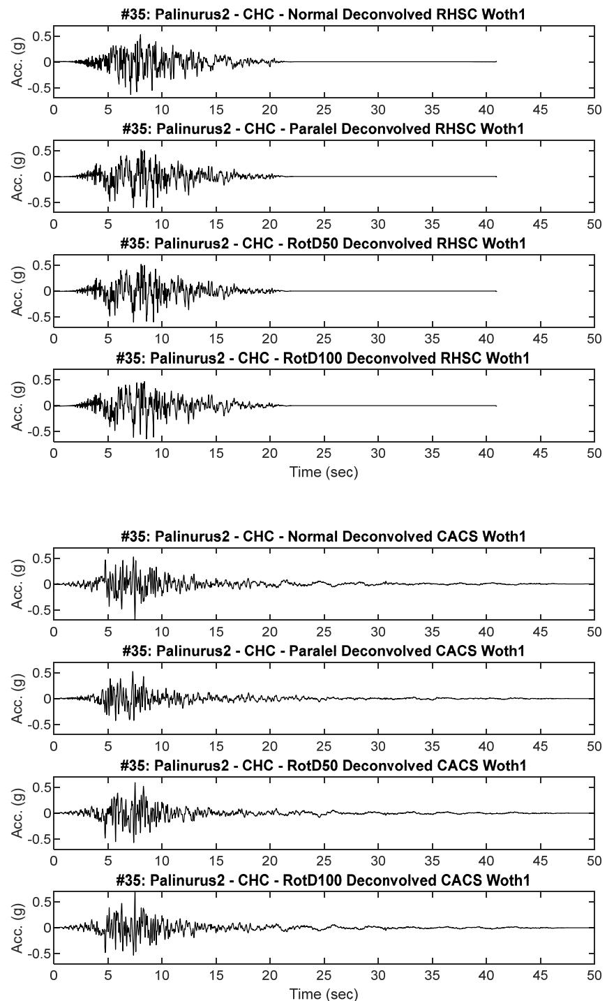
**Figure B35.2 Scaled RHSC and CACS Deconvolved input motion acceleration time history placed at Riccarton Gravel elevation for dynamic analysis**
