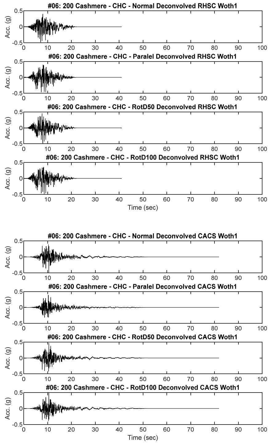
**Figure B6.2 Scaled RHSC and CACS Deconvolved input motion acceleration time history placed at Riccarton Gravel elevation for dynamic analysis**
