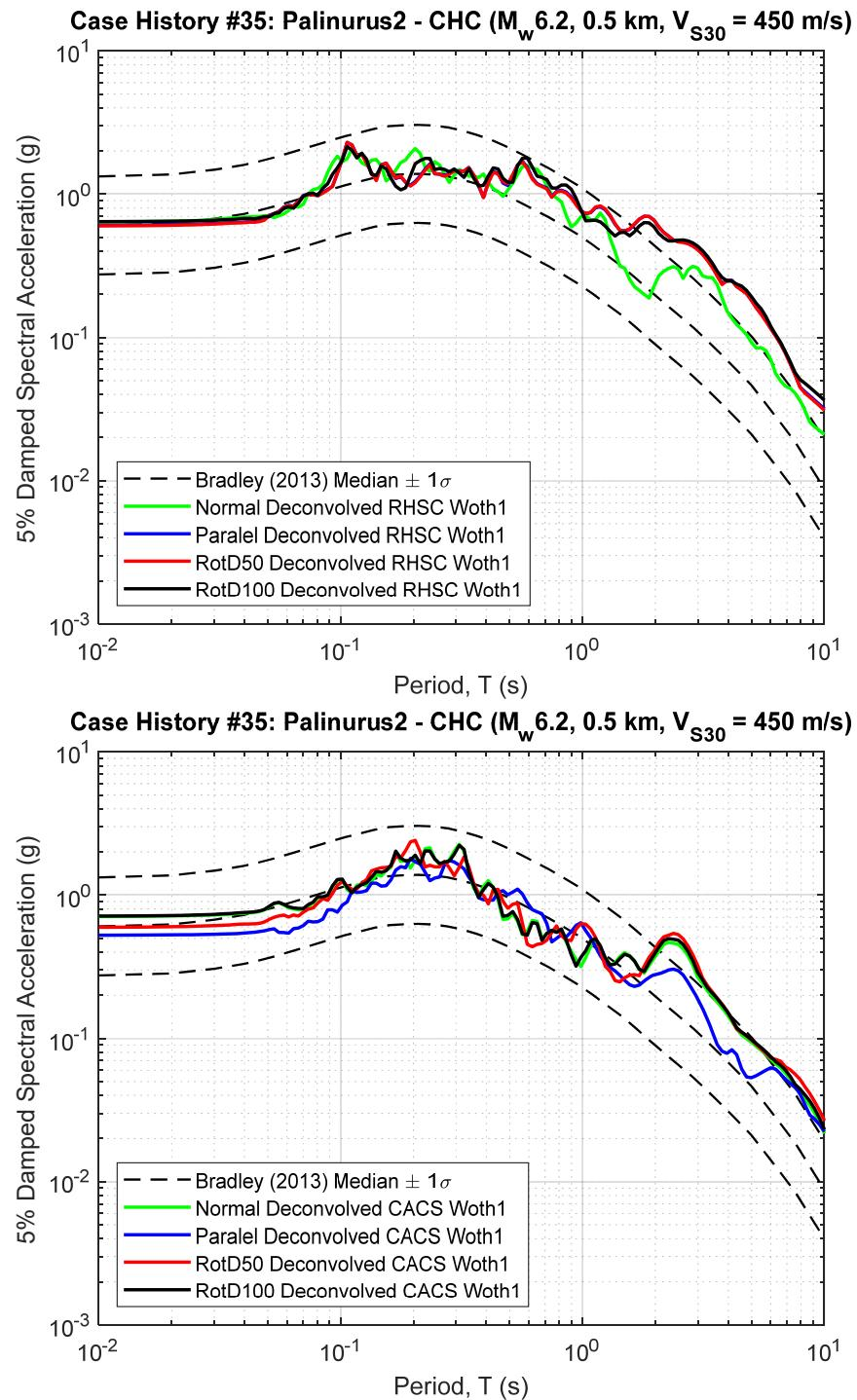
**Figure B35.1 5% Damped Response Spectra of RHSC and CACS Deconvolved Input Motion at Riccarton Gravel (multiplied by the scaling factor to represent the  $R_{rup}$  and  $V_{S30}$  of studied site)**
