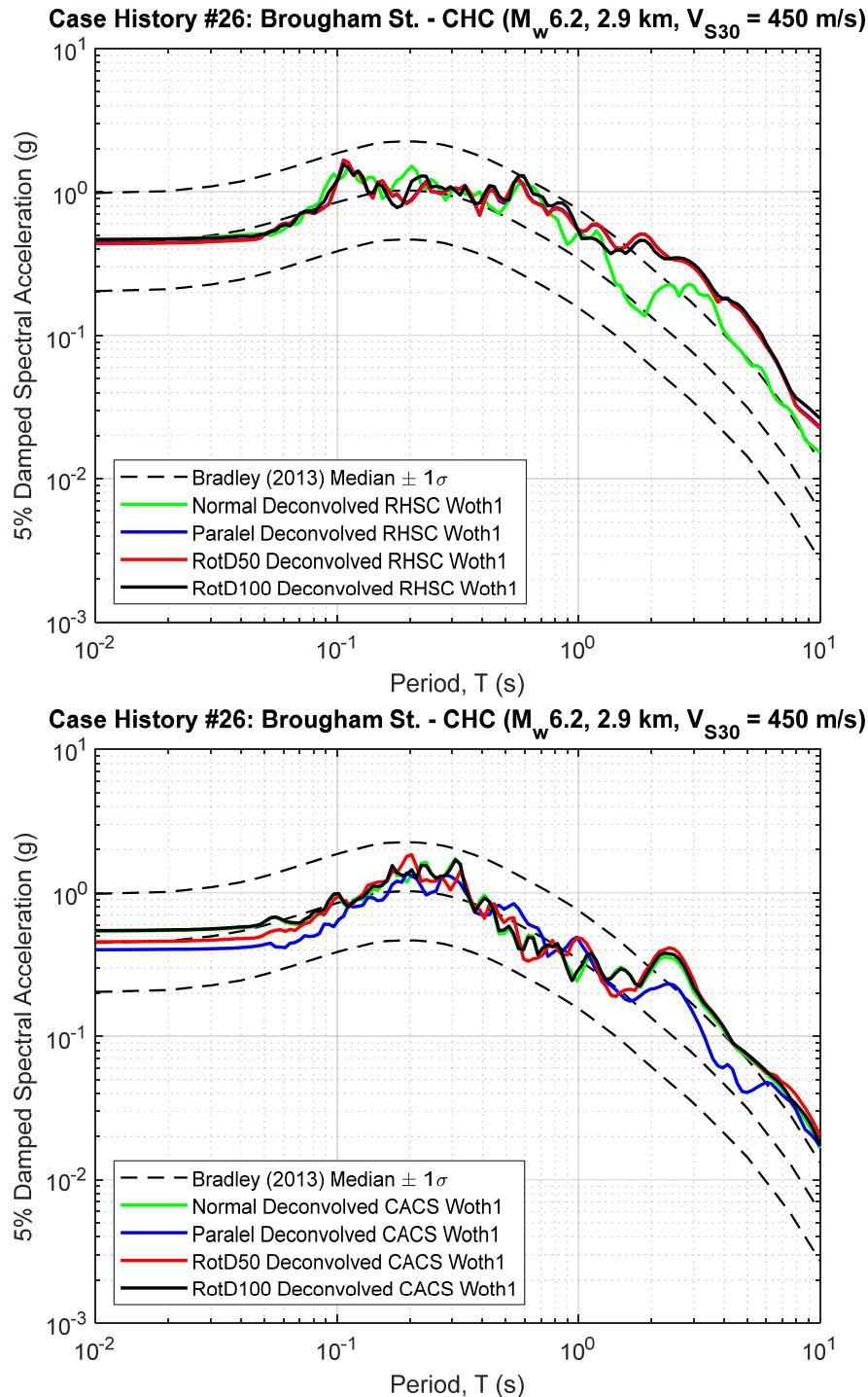
**Figure B26.1 5% Damped Response Spectra of RHSC and CACS Deconvolved Input Motion at Riccarton Gravel (multiplied by the scaling factor to represent the  $R_{rup}$  and  $V_{S30}$  of studied site)**
