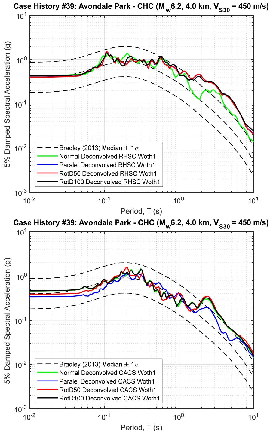
**Figure B39.1 5% Damped Response Spectra of RHSC and CACS Deconvolved Input Motion at Riccarton Gravel (multiplied by the scaling factor to represent the  $R_{rup}$  and  $V_{S30}$  of studied site)**
