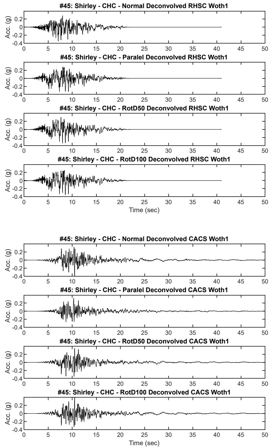
**Figure B45.2 Scaled RHSC and CACS Deconvolved input motion acceleration time history placed at Riccarton Gravel elevation for dynamic analysis**
