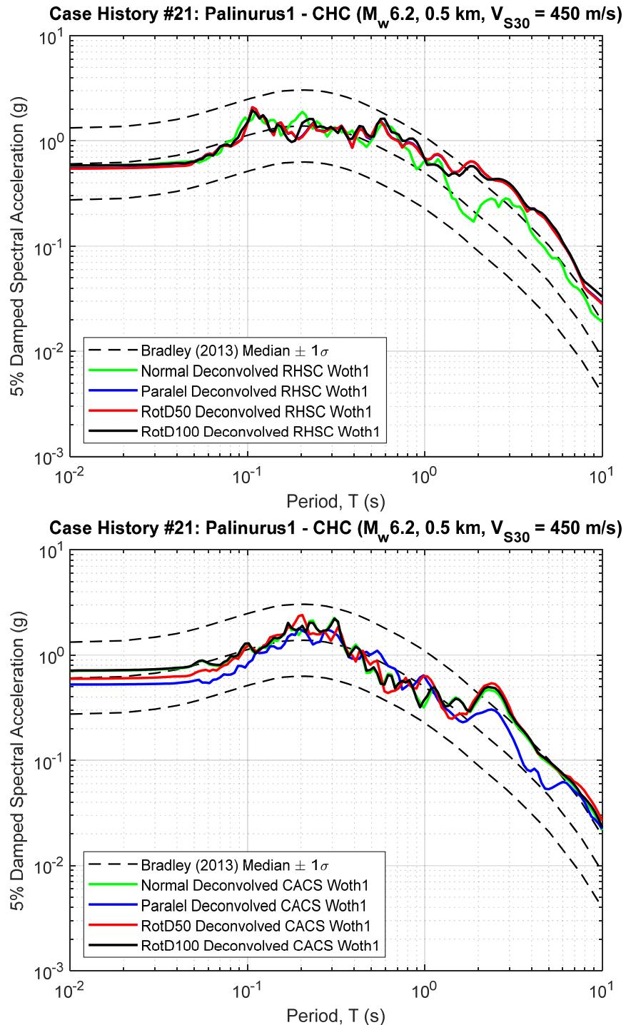
**Figure B21.1 5% Damped Response Spectra of RHSC and CACS Deconvolved Input Motion at Riccarton Gravel (multiplied by the scaling factor to represent the  $R_{rup}$  and  $V_{S30}$  of studied site)**
