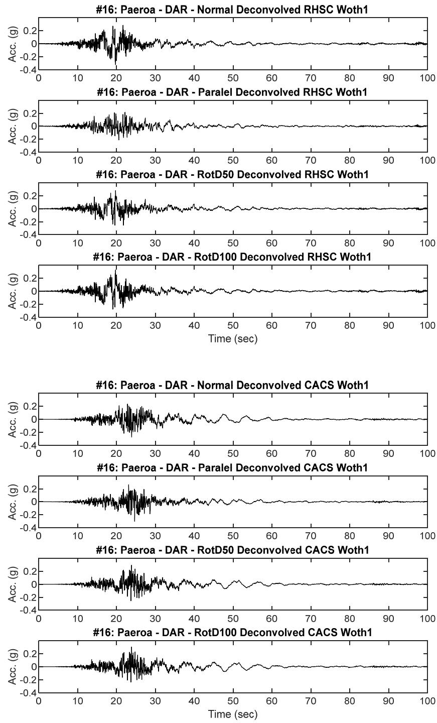
**Figure B16.2 Scaled RHSC and CACS Deconvolved input motion acceleration time history placed at Riccarton Gravel elevation for dynamic analysis**
