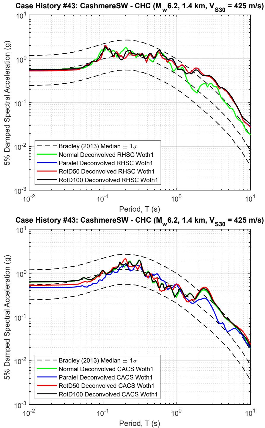
**Figure B43.1 5% Damped Response Spectra of RHSC and CACS Deconvolved Input Motion at Riccarton Gravel (multiplied by the scaling factor to represent the  $R_{rup}$  and  $V_{S30}$  of studied site)**
