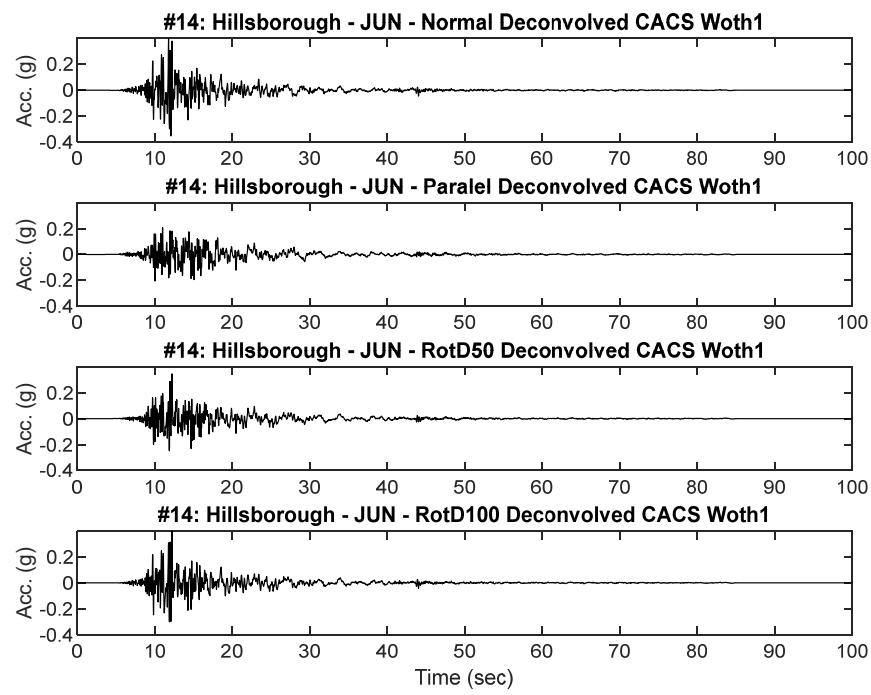
**Figure B14.2 Scaled RHSC and CACS Deconvolved input motion acceleration time history placed at Riccarton Gravel elevation for dynamic analysis**
