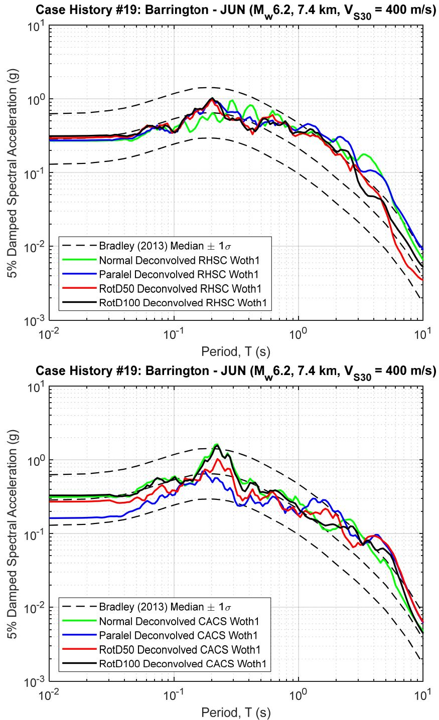
**Figure B18.1 5% Damped Response Spectra of RHSC and CACS Deconvolved Input Motion at Riccarton Gravel (multiplied by the scaling factor to represent the  $R_{rup}$  and  $V_{S30}$  of studied site)**
