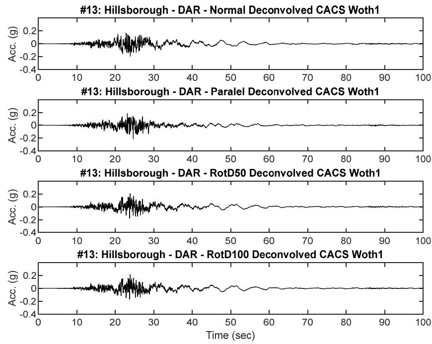
**Figure B13.2 Scaled RHSC and CACS Deconvolved input motion acceleration time history placed at Riccarton Gravel elevation for dynamic analysis**
