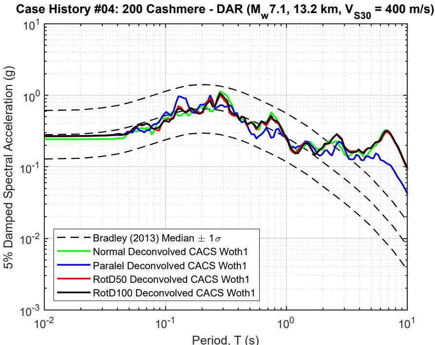
**Figure B4.1 5% Damped Response Spectra of RHSC and CACS Deconvolved Input Motion at Riccarton Gravel (multiplied by the scaling factor to represent the  $R_{rup}$  and  $V_{S30}$  of studied site)**
