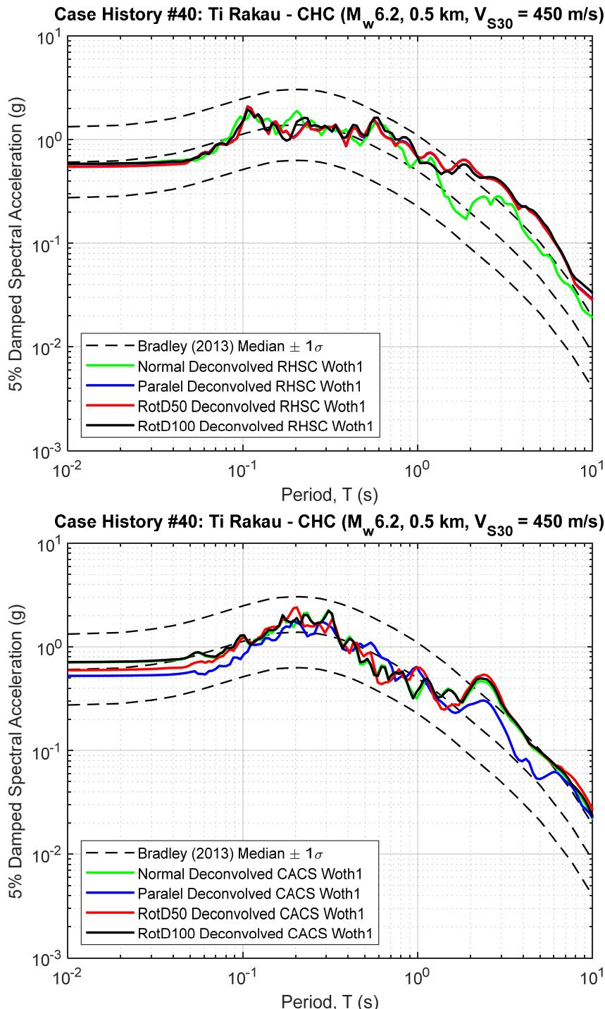
**Figure B40.1 5% Damped Response Spectra of RHSC and CACS Deconvolved Input Motion at Riccarton Gravel (multiplied by the scaling factor to represent the  $R_{rup}$  and  $V_{S30}$  of studied site)**
