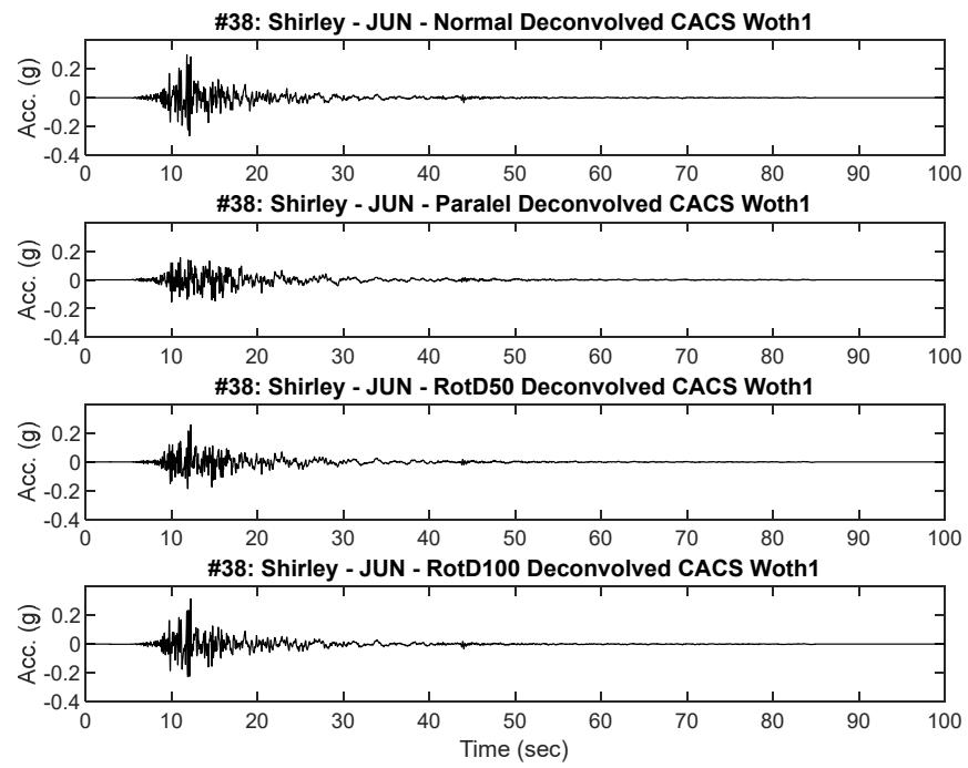
**Figure B38.2 Scaled RHSC and CACS Deconvolved input motion acceleration time history placed at Riccarton Gravel elevation for dynamic analysis**
