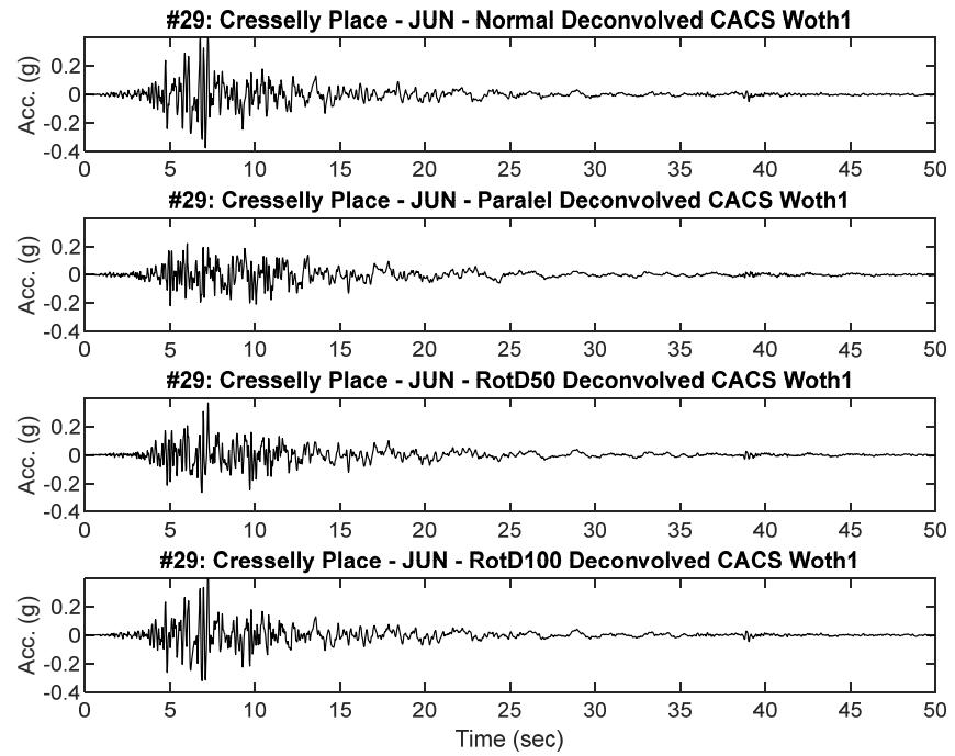
**Figure B29.2 Scaled RHSC and CACS Deconvolved input motion acceleration time history placed at Riccarton Gravel elevation for dynamic analysis**
