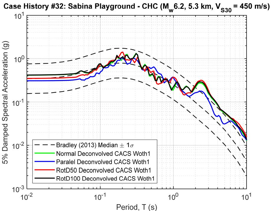
**Figure B32.1 5% Damped Response Spectra of RHSC and CACS Deconvolved Input Motion at Riccarton Gravel (multiplied by the scaling factor to represent the  $R_{rup}$  and  $V_{S30}$  of studied site)**
