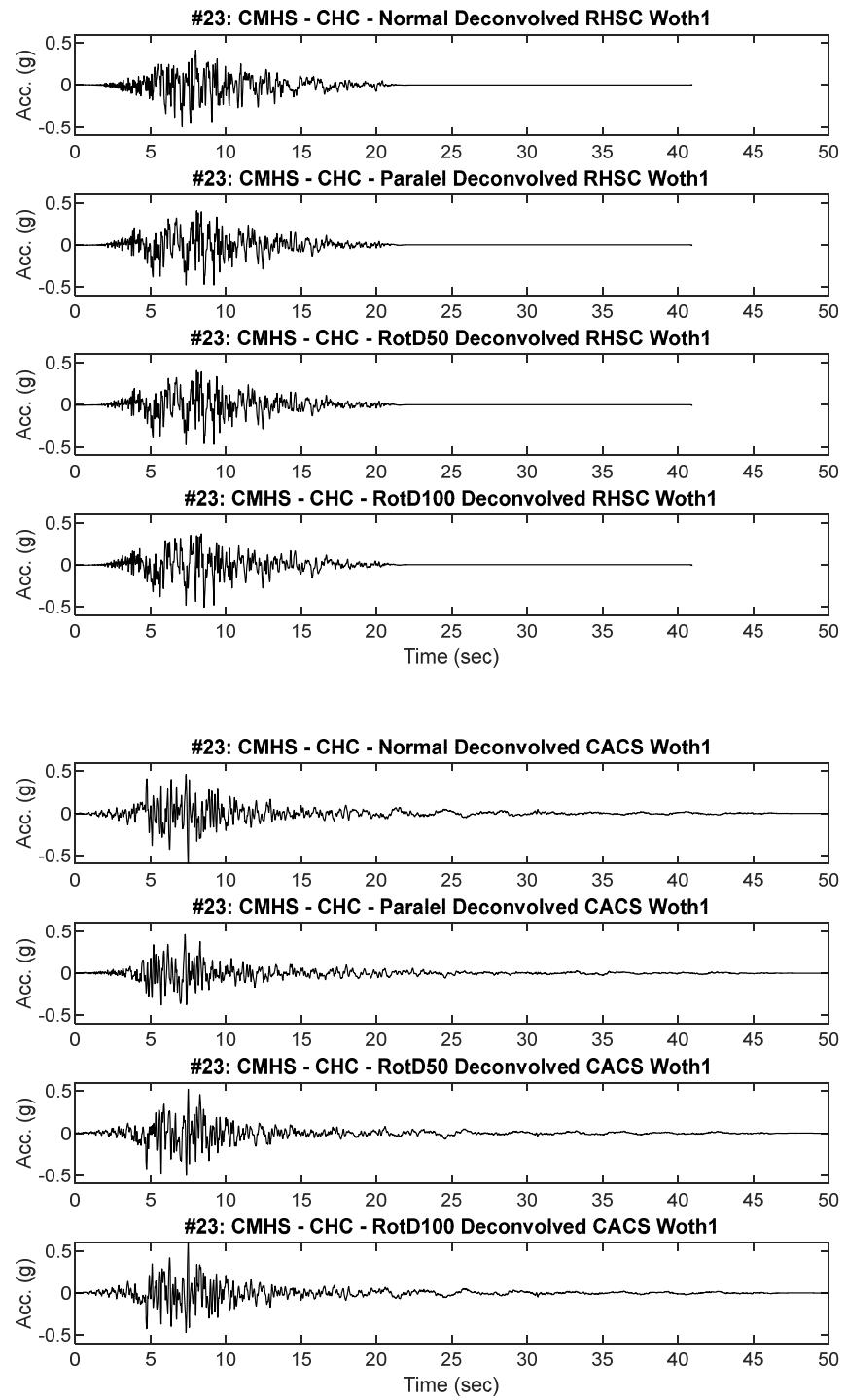
**Figure B23.2 Scaled RHSC and CACS Deconvolved input motion acceleration time history placed at Riccarton Gravel elevation for dynamic analysis**
