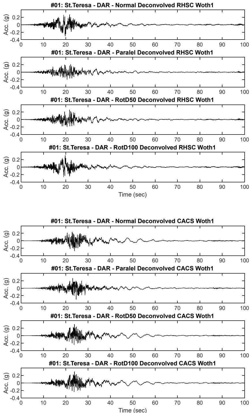
**Figure B1.2 Scaled RHSC and CACS Deconvolved input motion acceleration time history placed at Riccarton Gravel elevation for dynamic analysis**
