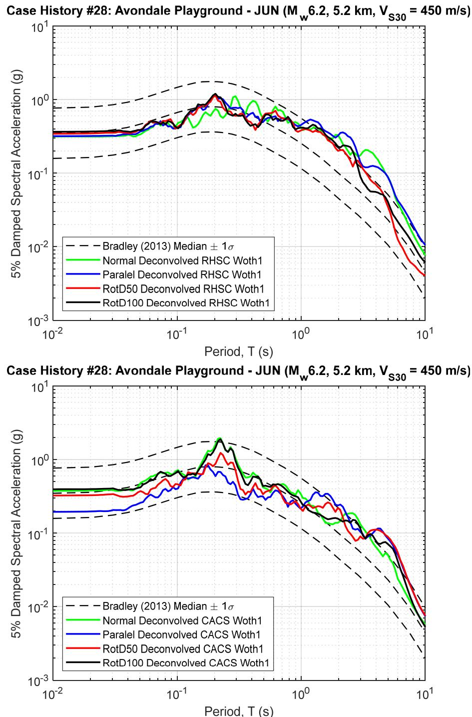
**Figure B28.1 5% Damped Response Spectra of RHSC and CACS Deconvolved Input Motion at Riccarton Gravel (multiplied by the scaling factor to represent the  $R_{rup}$  and  $V_{S30}$  of studied site)**
