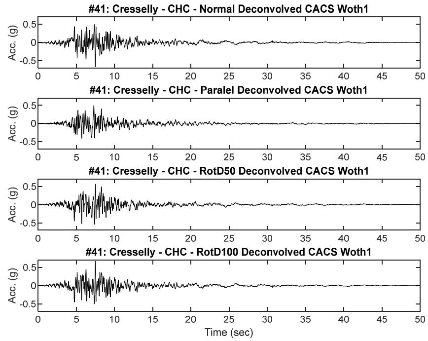
**Figure B41.2 Scaled RHSC and CACS Deconvolved input motion acceleration time history placed at Riccarton Gravel elevation for dynamic analysis**
