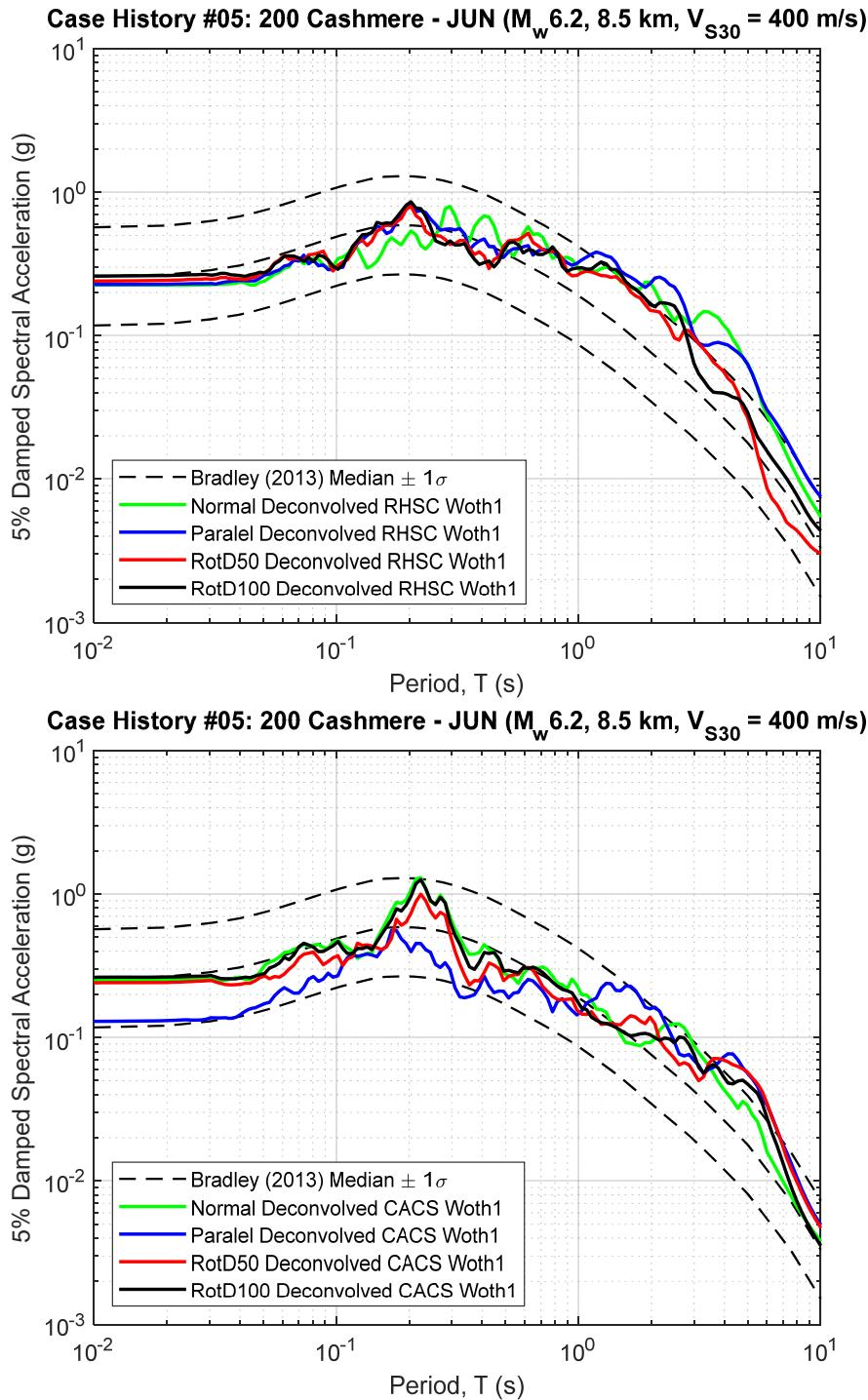
**Figure B5.1 5% Damped Response Spectra of RHSC and CACS Deconvolved Input Motion at Riccarton Gravel (multiplied by the scaling factor to represent the  $R_{rup}$  and  $V_{S30}$  of studied site)**
