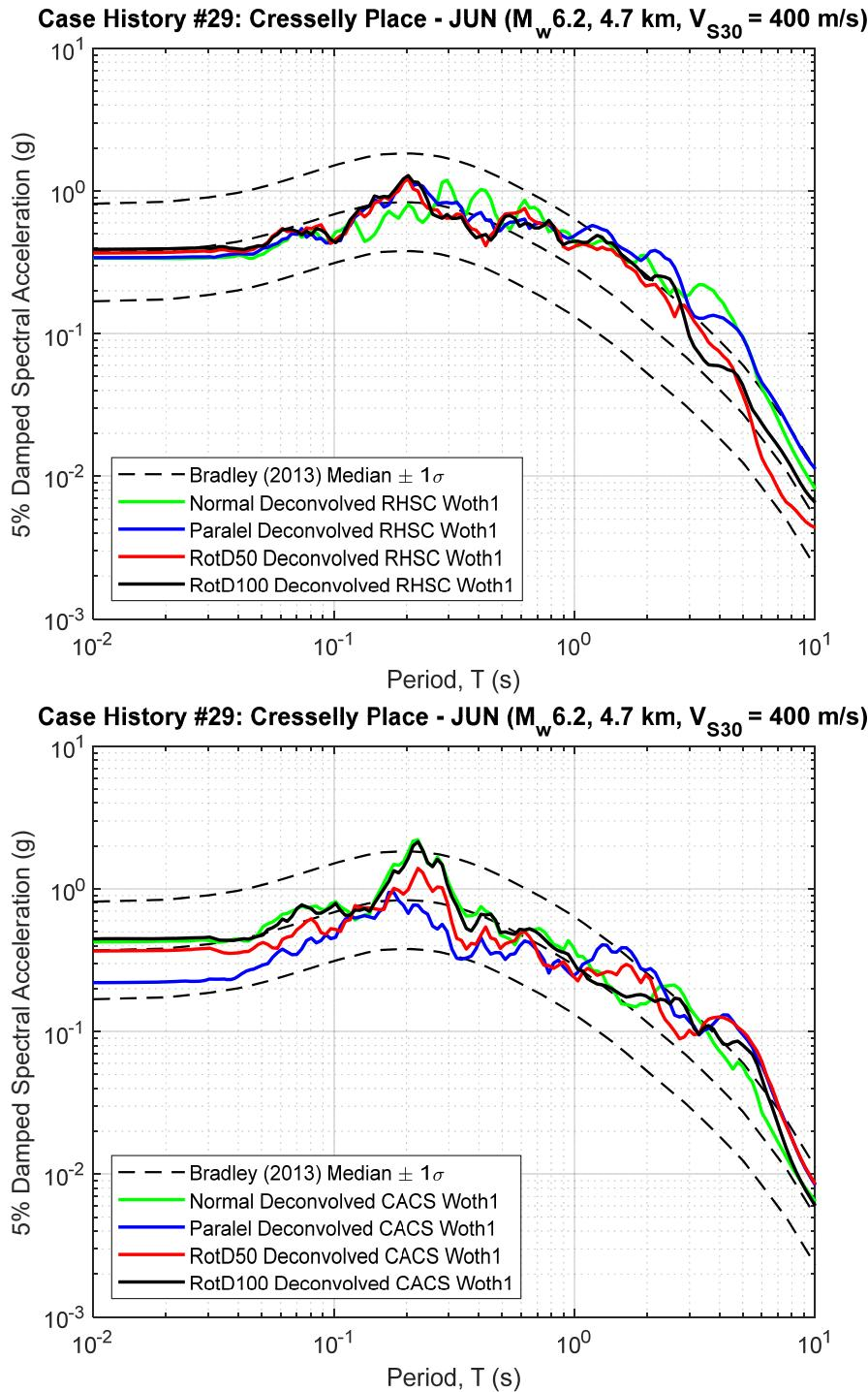
**Figure B29.1 5% Damped Response Spectra of RHSC and CACS Deconvolved Input Motion at Riccarton Gravel (multiplied by the scaling factor to represent the  $R_{rup}$  and  $V_{S30}$  of studied site)**
