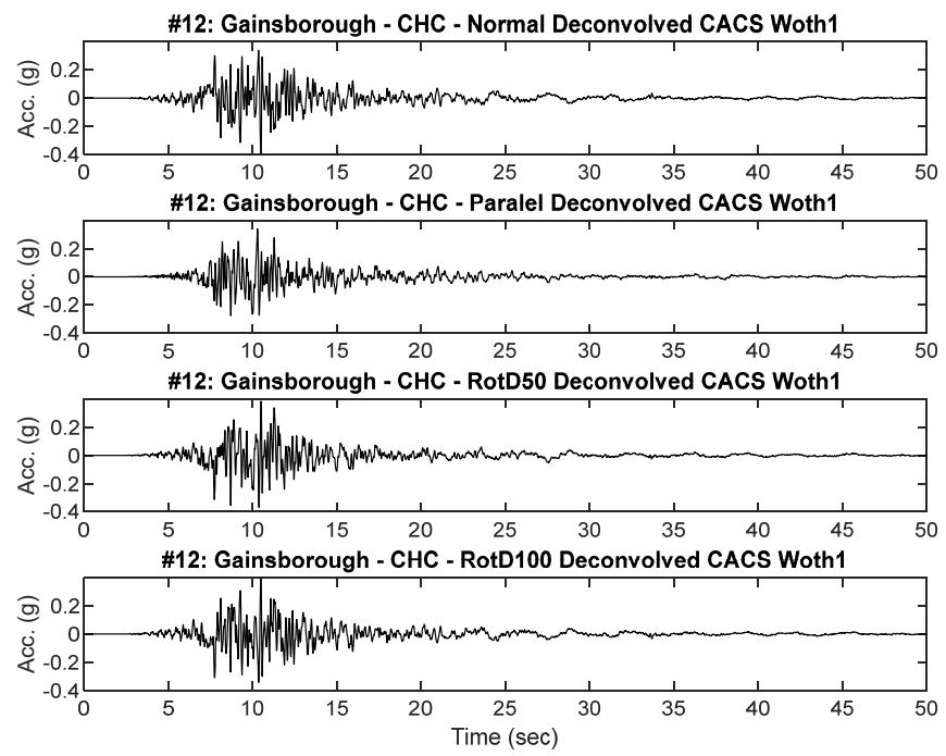
**Figure B12.2 Scaled RHSC and CACS Deconvolved input motion acceleration time history placed at Riccarton Gravel elevation for dynamic analysis**
