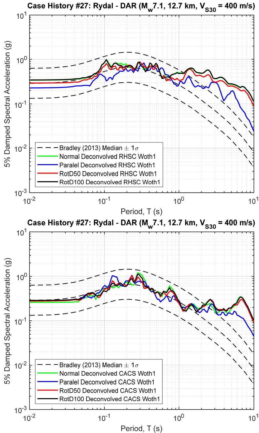
**Figure B27.1 5% Damped Response Spectra of RHSC and CACS Deconvolved Input Motion at Riccarton Gravel (multiplied by the scaling factor to represent the  $R_{rup}$  and  $V_{S30}$  of studied site)**
