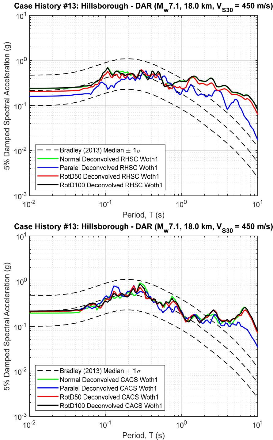
**Figure B13.1 5% Damped Response Spectra of RHSC and CACS Deconvolved Input Motion at Riccarton Gravel (multiplied by the scaling factor to represent the  $R_{rup}$  and  $V_{S30}$  of studied site)**
