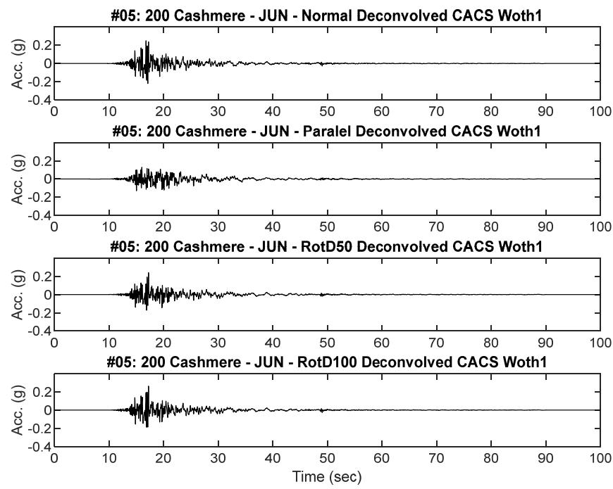
**Figure B5.2 Scaled RHSC and CACS Deconvolved input motion acceleration time history placed at Riccarton Gravel elevation for dynamic analysis**
