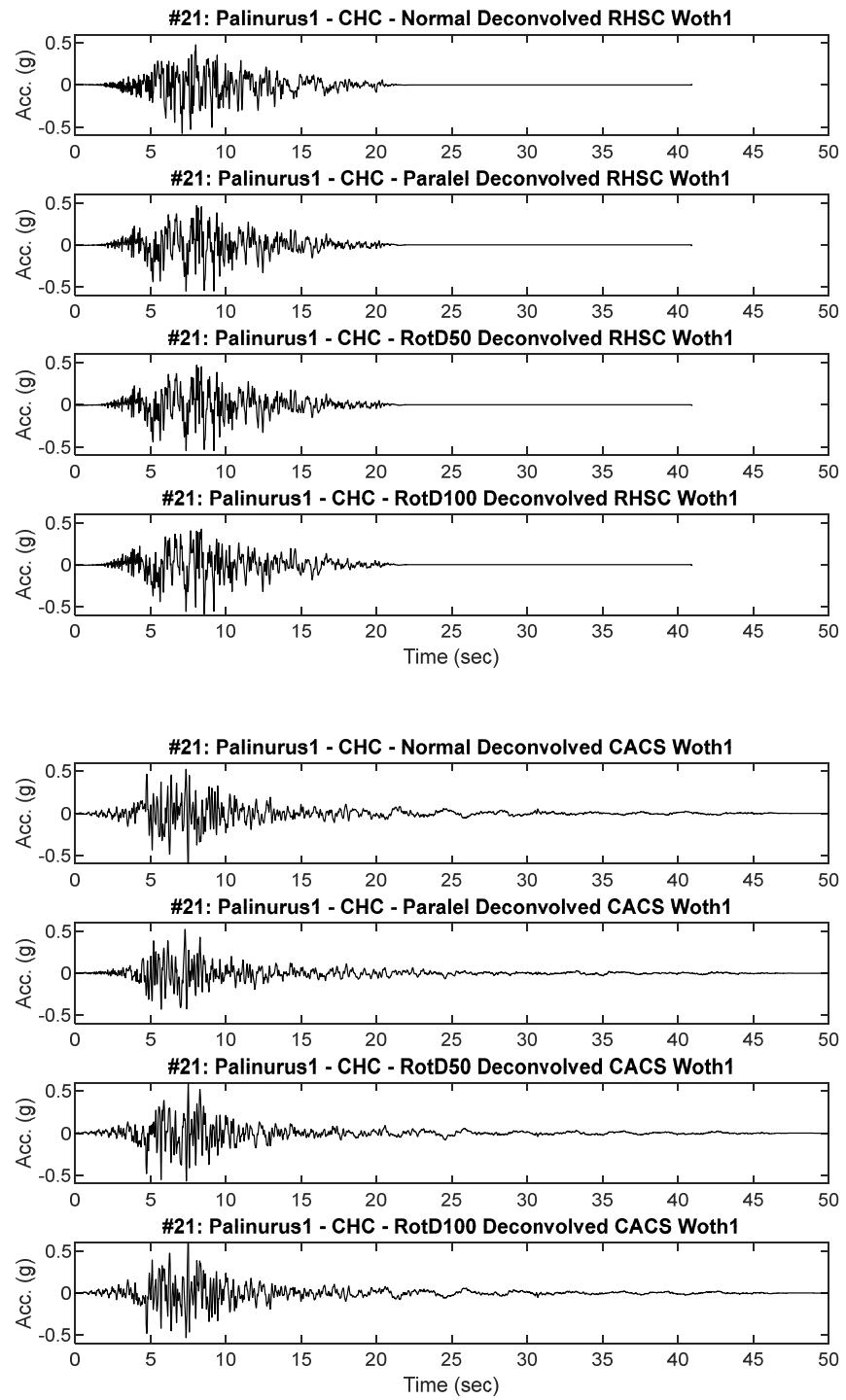
**Figure B21.2 Scaled RHSC and CACS Deconvolved input motion acceleration time history placed at Riccarton Gravel elevation for dynamic analysis**
