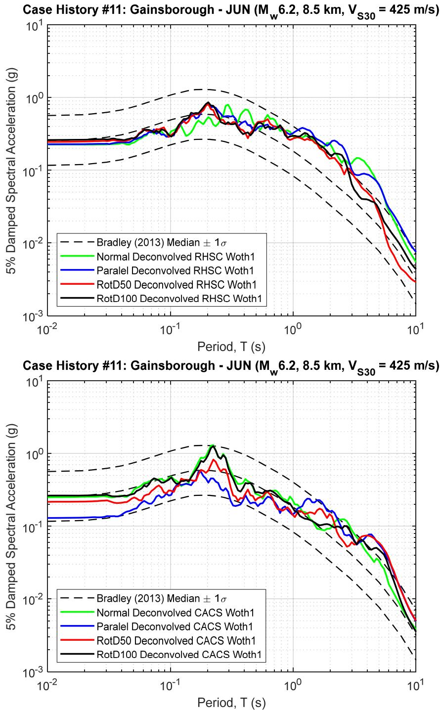
**Figure B11.1 5% Damped Response Spectra of RHSC and CACS Deconvolved Input Motion at Riccarton Gravel (multiplied by the scaling factor to represent the  $R_{rup}$  and  $V_{S30}$  of studied site)**
