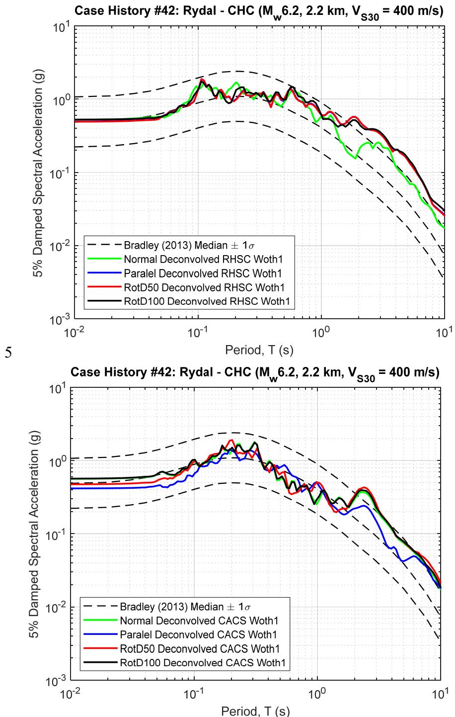
**Figure B42.1 5% Damped Response Spectra of RHSC and CACS Deconvolved Input Motion at Riccarton Gravel (multiplied by the scaling factor to represent the  $R_{rup}$  and  $V_{S30}$  of studied site)**
