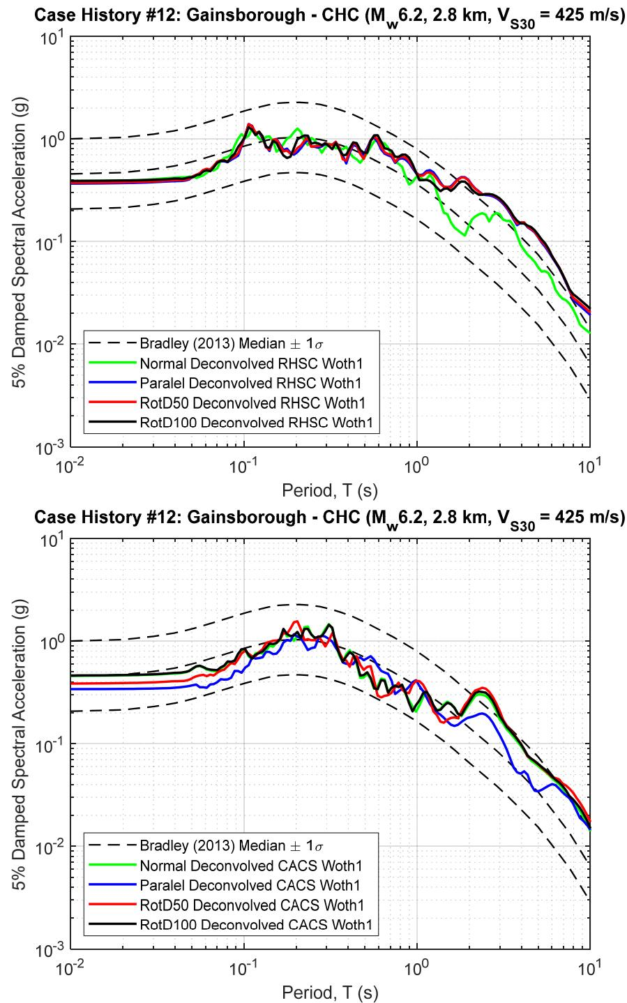
**Figure B12.1 5% Damped Response Spectra of RHSC and CACS Deconvolved Input Motion at Riccarton Gravel (multiplied by the scaling factor to represent the  $R_{rup}$  and  $V_{S30}$  of studied site)**
