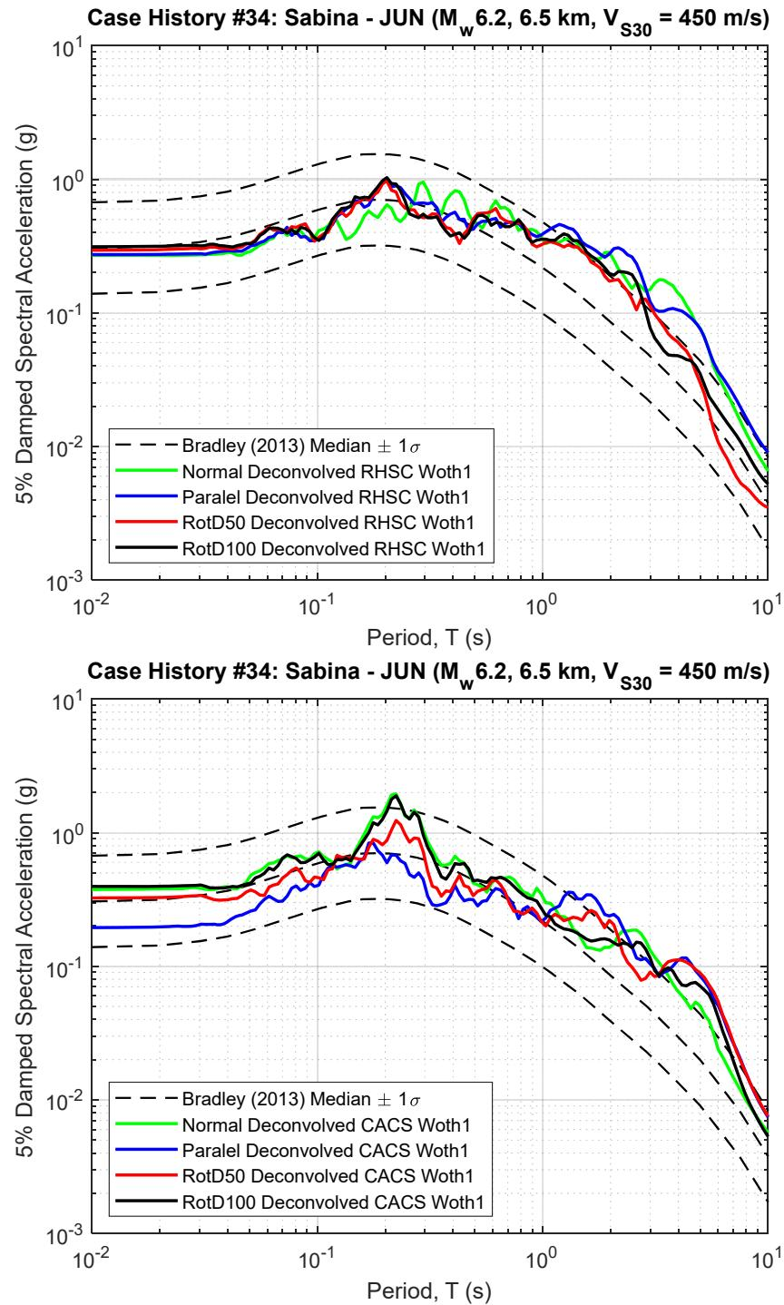
**Figure B34.1 5% Damped Response Spectra of RHSC and CACS Deconvolved Input Motion at Riccarton Gravel (multiplied by the scaling factor to represent the  $R_{rup}$  and  $V_{S30}$  of studied site)**
