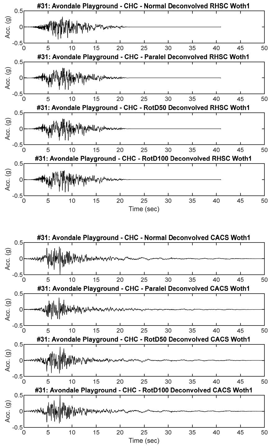
**Figure B31.2 Scaled RHSC and CACS Deconvolved input motion acceleration time history placed at Riccarton Gravel elevation for dynamic analysis**
