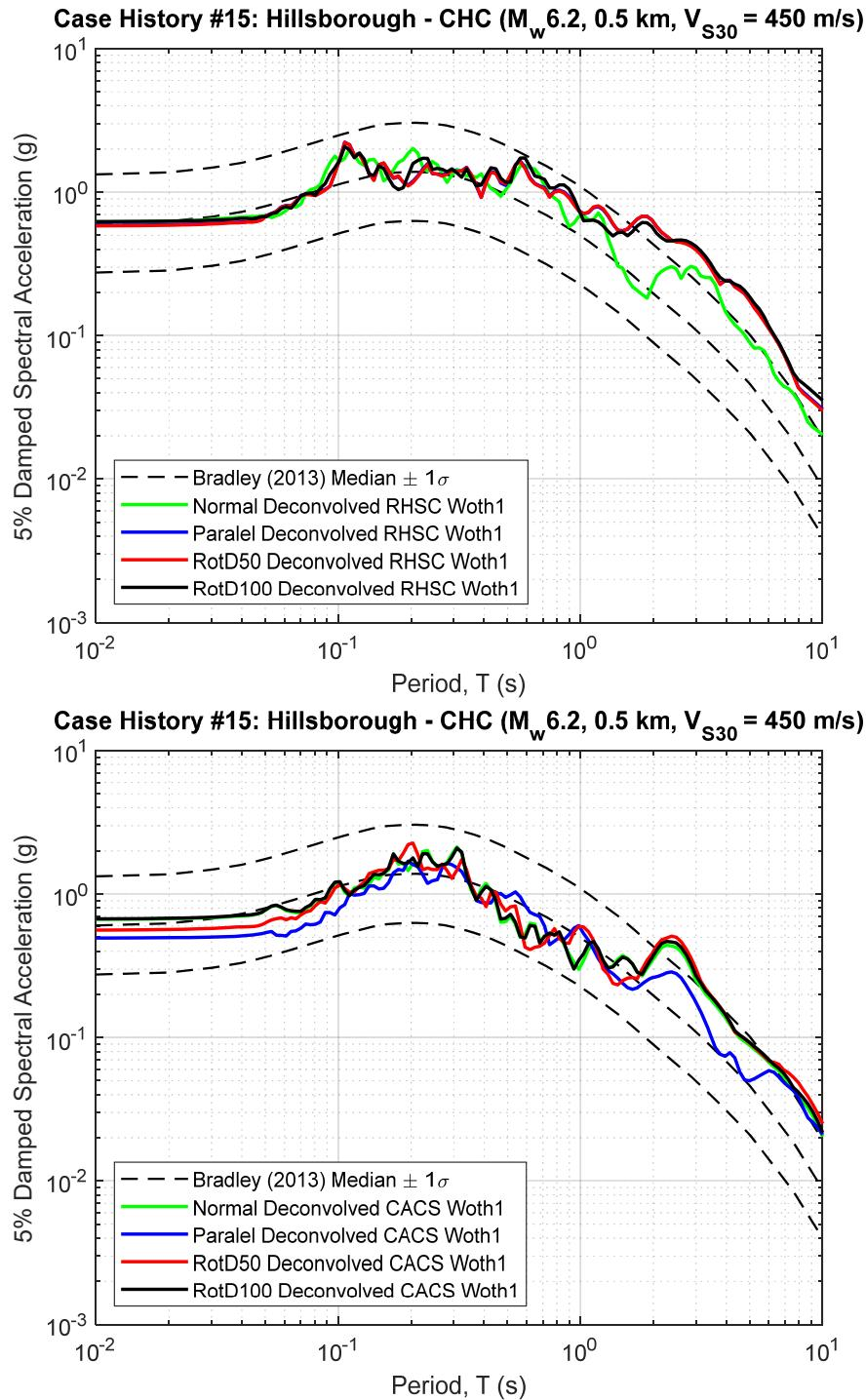
**Figure B15.1 5% Damped Response Spectra of RHSC and CACS Deconvolved Input Motion at Riccarton Gravel (multiplied by the scaling factor to represent the  $R_{rup}$  and  $V_{S30}$  of studied site)**
