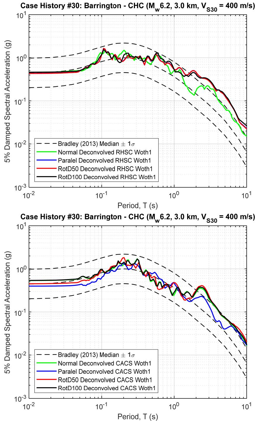
**Figure B30.1 5% Damped Response Spectra of RHSC and CACS Deconvolved Input Motion at Riccarton Gravel (multiplied by the scaling factor to represent the  $R_{rup}$  and  $V_{S30}$  of studied site)**
