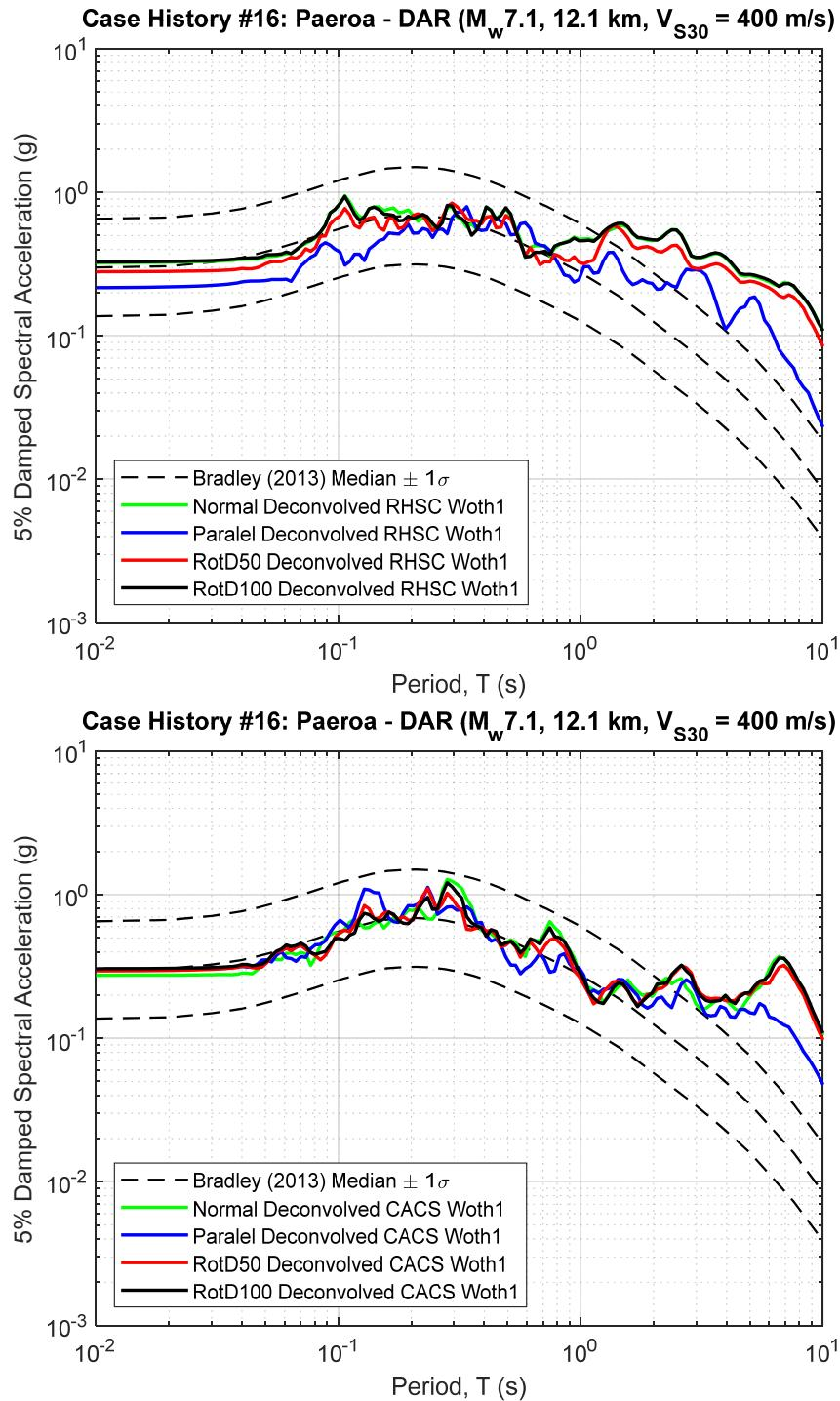
**Figure B16.1 5% Damped Response Spectra of RHSC and CACS Deconvolved Input Motion at Riccarton Gravel (multiplied by the scaling factor to represent the  $R_{rup}$  and  $V_{S30}$  of studied site)**
