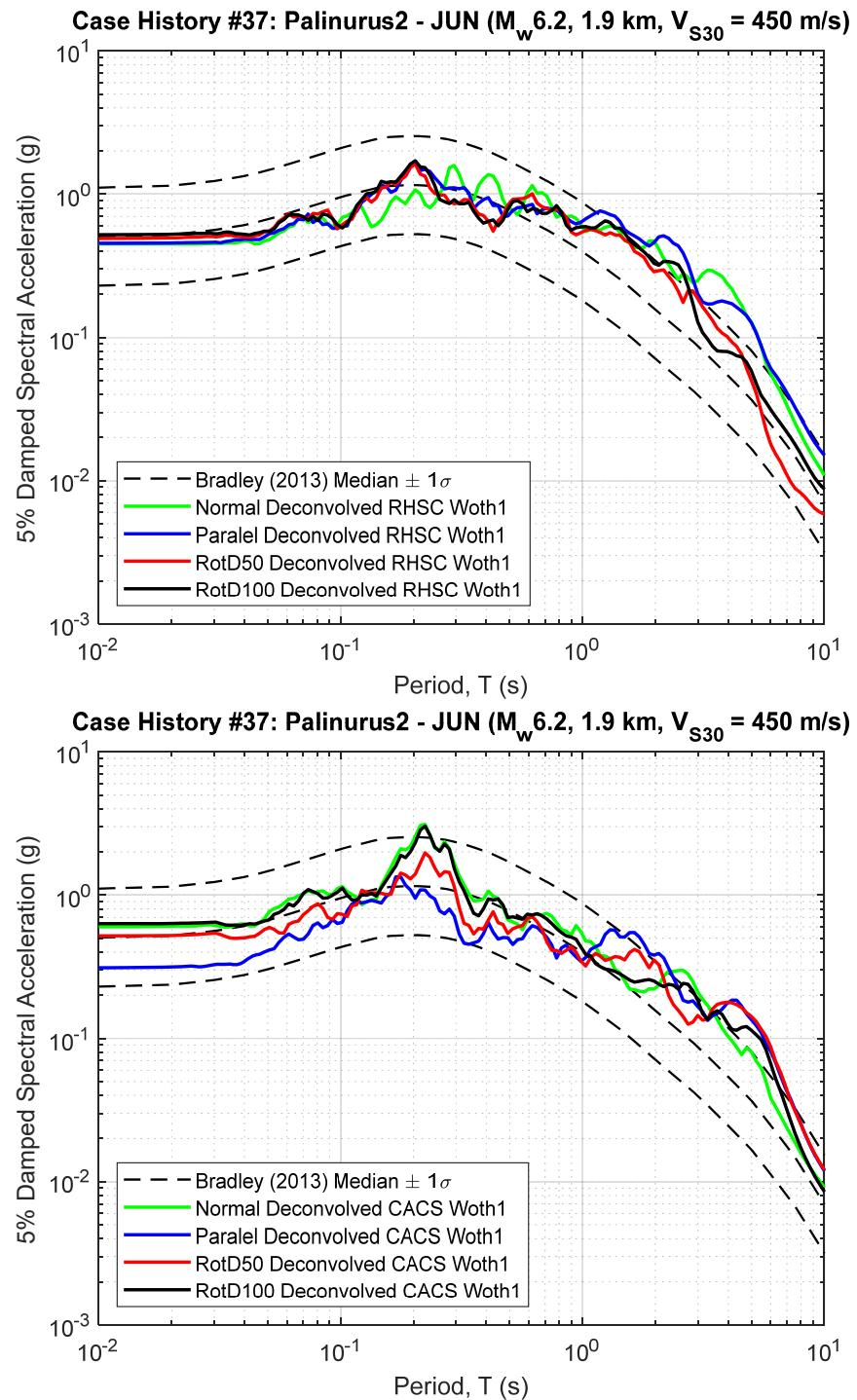
**Figure B37.1 5% Damped Response Spectra of RHSC and CACS Deconvolved Input Motion at Riccarton Gravel (multiplied by the scaling factor to represent the  $R_{rup}$  and  $V_{S30}$  of studied site)**
