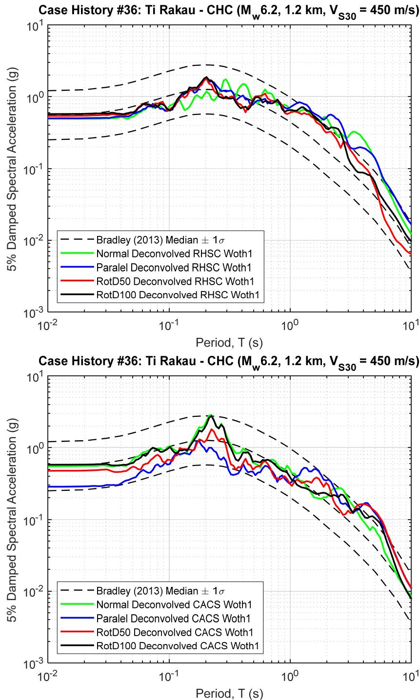
**Figure B36.1 5% Damped Response Spectra of RHSC and CACS Deconvolved Input Motion at Riccarton Gravel (multiplied by the scaling factor to represent the  $R_{rup}$  and  $V_{S30}$  of studied site)**
