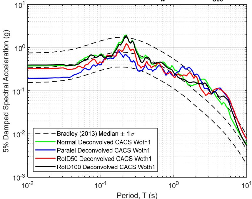
**Figure B33.1 5% Damped Response Spectra of RHSC and CACS Deconvolved Input Motion at Riccarton Gravel (multiplied by the scaling factor to represent the  $R_{rup}$  and  $V_{S30}$  of studied site)**
