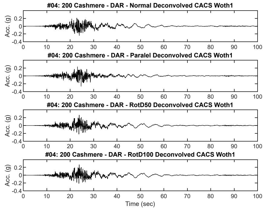
**Figure B4.2 Scaled RHSC and CACS Deconvolved input motion acceleration time history placed at Riccarton Gravel elevation for dynamic analysis**
