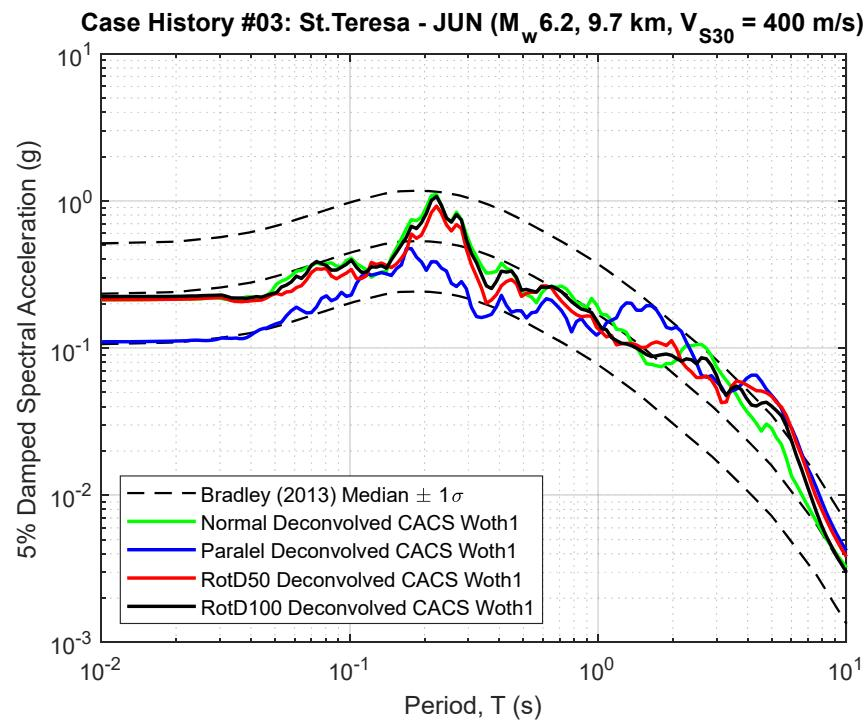
**Figure B3.1 5% Damped Response Spectra of RHSC and CACS Deconvolved Input Motion at Riccarton Gravel (multiplied by the scaling factor to represent the  $R_{rup}$  and  $V_{S30}$  of studied site)**
