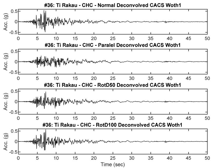
**Figure B36.2 Scaled RHSC and CACS Deconvolved input motion acceleration time history placed at Riccarton Gravel elevation for dynamic analysis**
