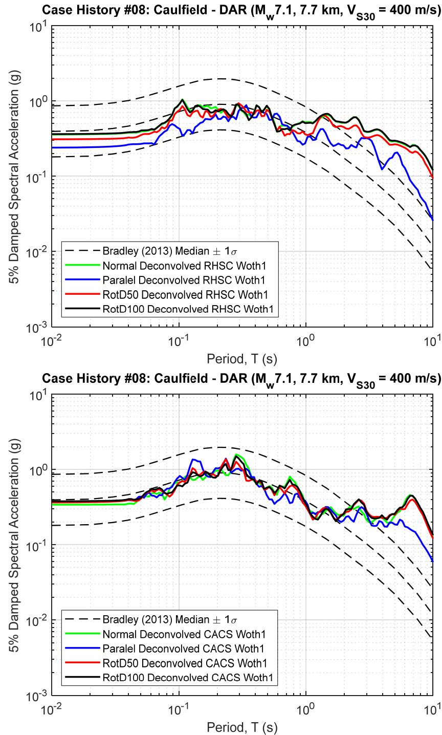
**Figure B8.1 5% Damped Response Spectra of RHSC and CACS Deconvolved Input Motion at Riccarton Gravel (multiplied by the scaling factor to represent the  $R_{rup}$  and  $V_{S30}$  of studied site)**
