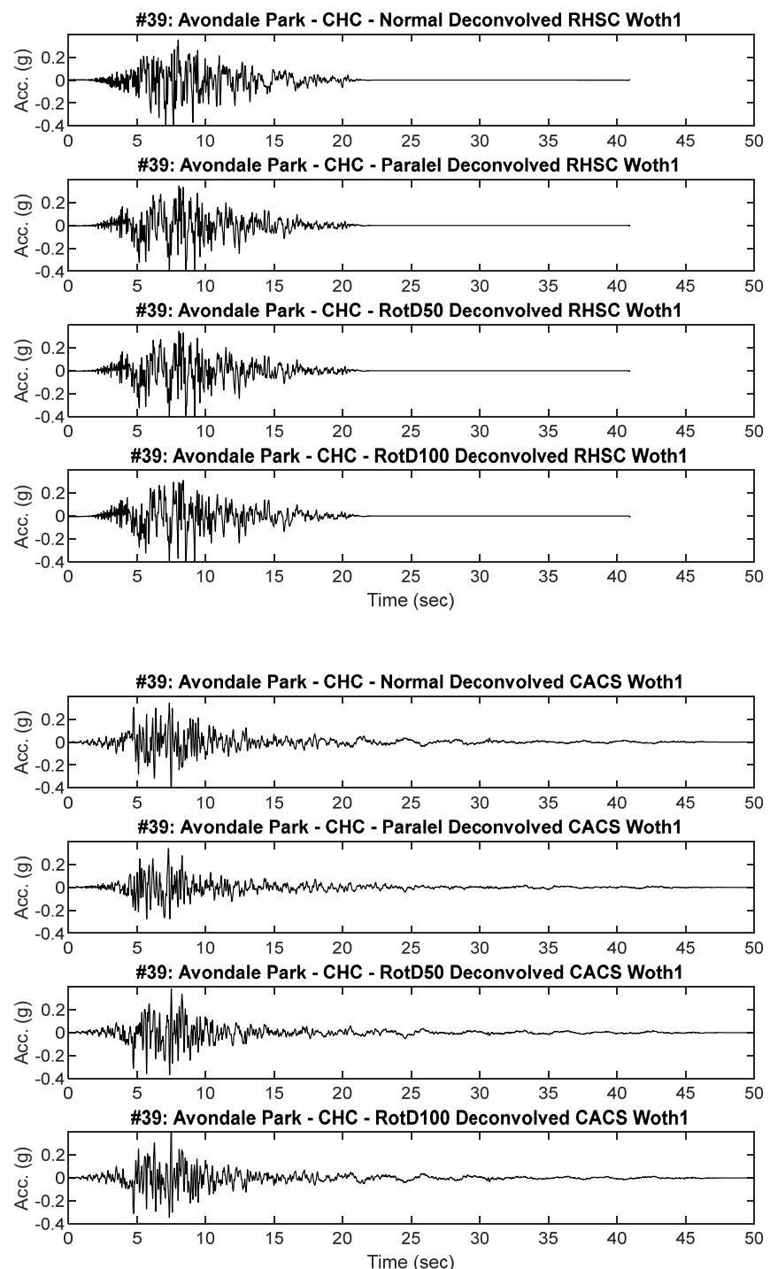
**Figure B39.2 Scaled RHSC and CACS Deconvolved input motion acceleration time history placed at Riccarton Gravel elevation for dynamic analysis**
