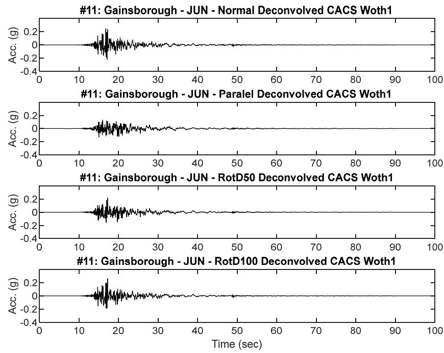
**Figure B11.2 Scaled RHSC and CACS Deconvolved input motion acceleration time history placed at Riccarton Gravel elevation for dynamic analysis**
