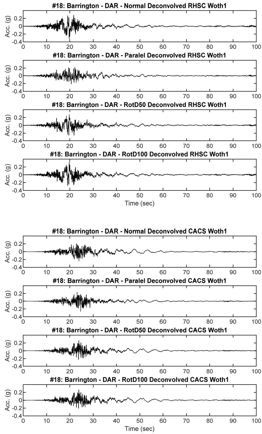
**Figure B18.2 Scaled RHSC and CACS Deconvolved input motion acceleration time history placed at Riccarton Gravel elevation for dynamic analysis**
