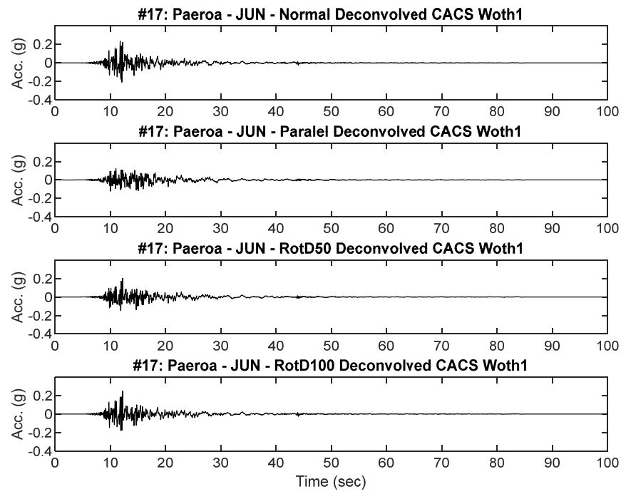
**Figure B17.2 Scaled RHSC and CACS Deconvolved input motion acceleration time history placed at Riccarton Gravel elevation for dynamic analysis**
