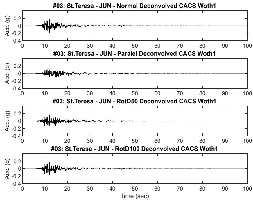
**Figure B3.2 Scaled RHSC and CACS Deconvolved input motion acceleration time history placed at Riccarton Gravel elevation for dynamic analysis**
