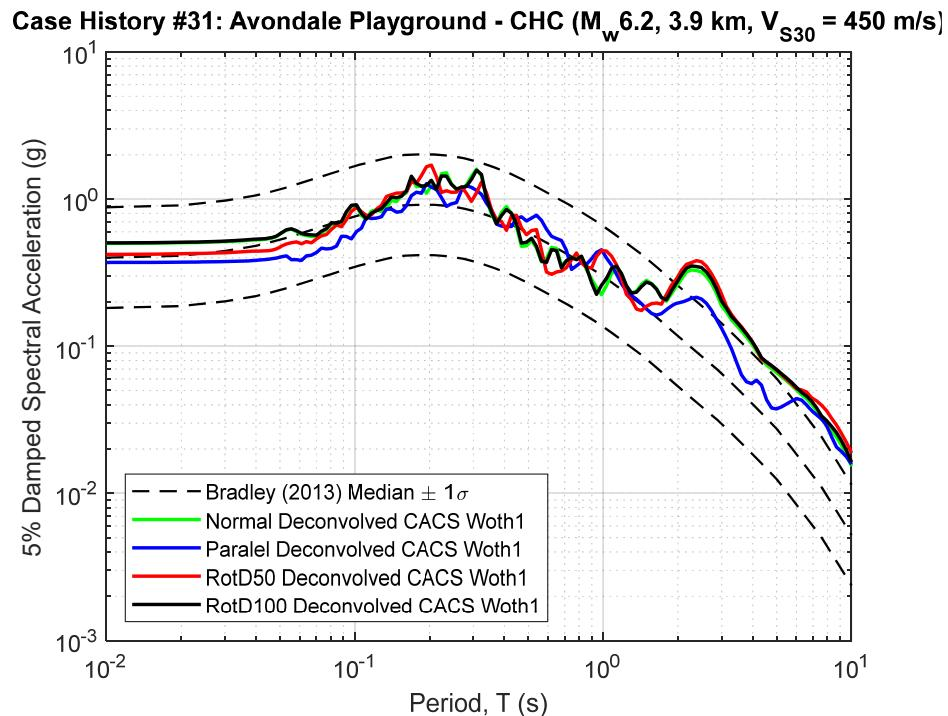
**Figure B31.1 5% Damped Response Spectra of RHSC and CACS Deconvolved Input Motion at Riccarton Gravel (multiplied by the scaling factor to represent the  $R_{rup}$  and  $V_{S30}$  of studied site)**
