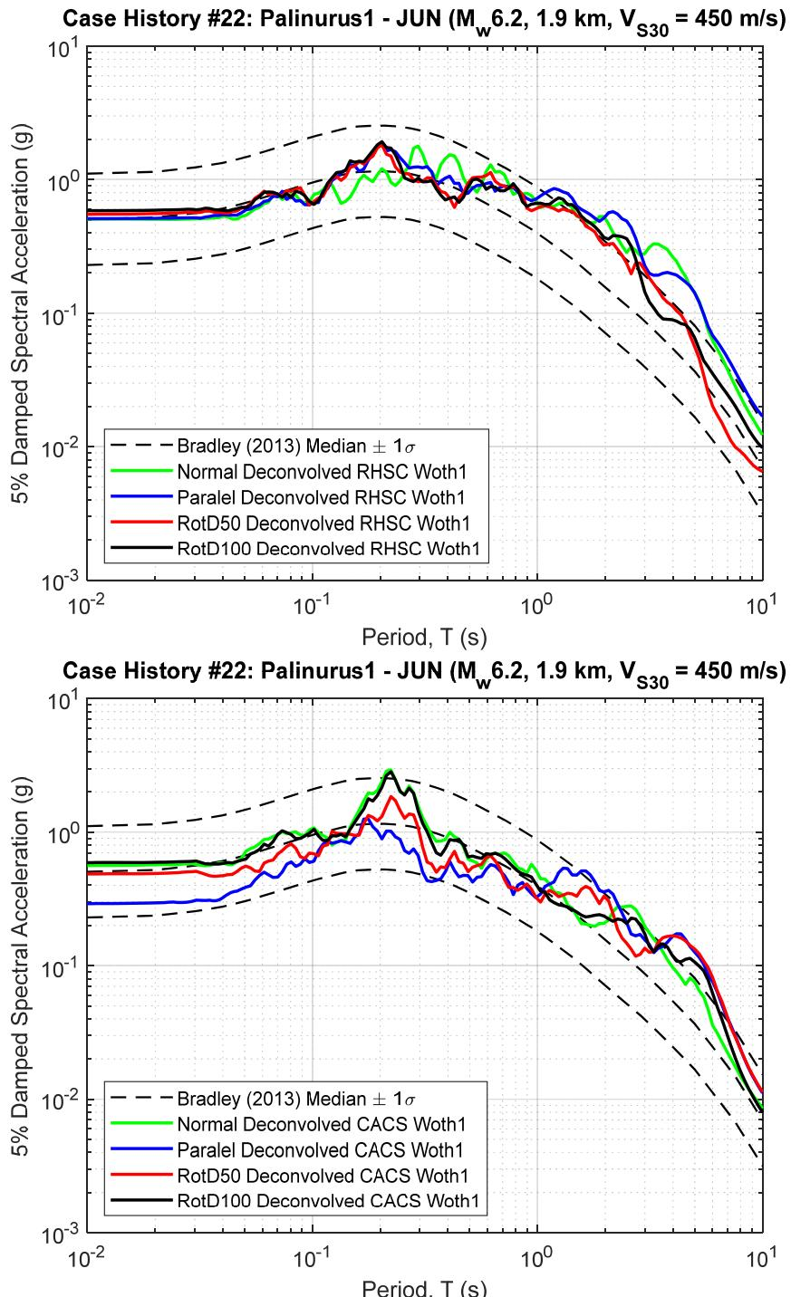
**Figure B22.1 5% Damped Response Spectra of RHSC and CACS Deconvolved Input Motion at Riccarton Gravel (multiplied by the scaling factor to represent the  $R_{rup}$  and  $V_{S30}$  of studied site)**
