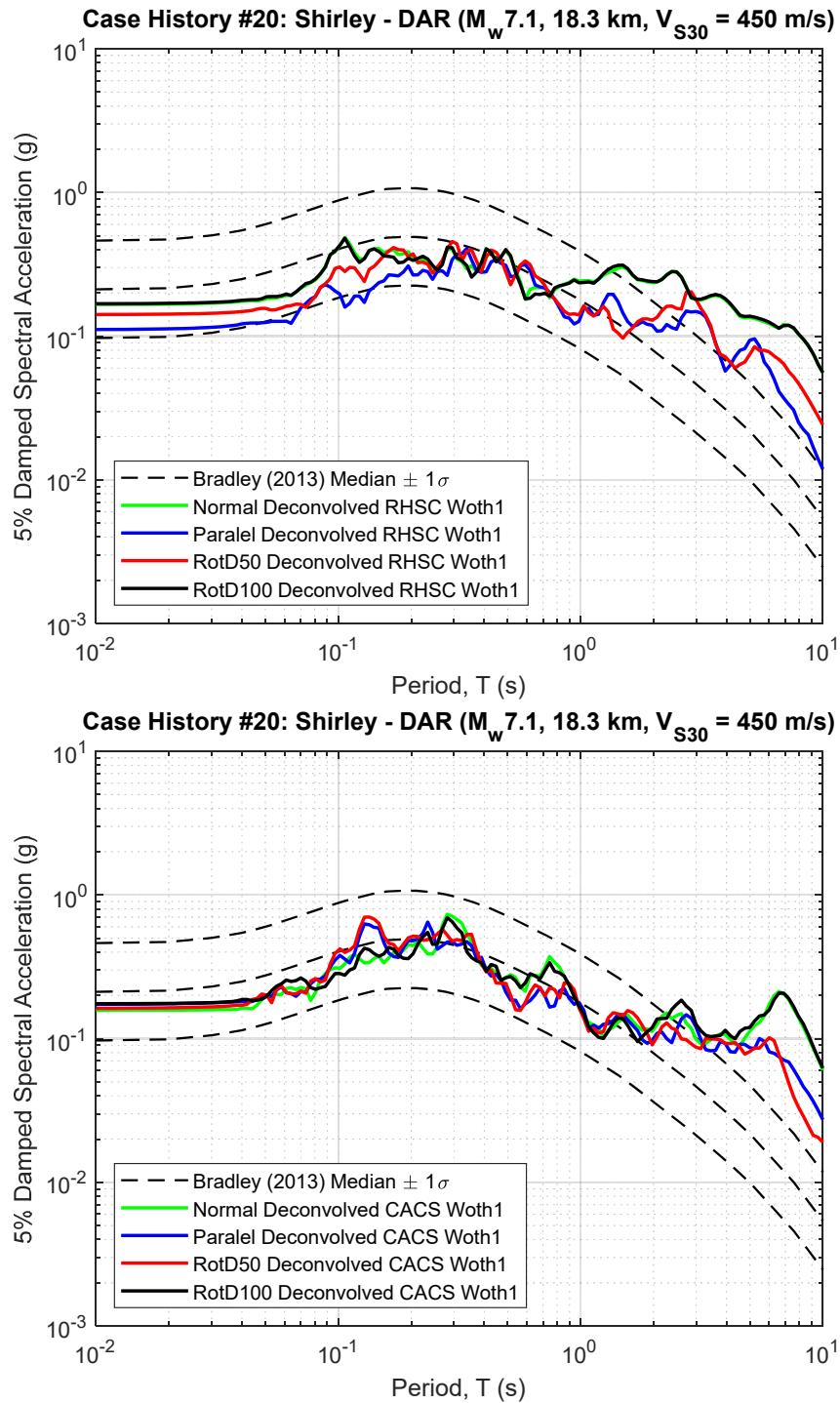
**Figure B20.1 5% Damped Response Spectra of RHSC and CACS Deconvolved Input Motion at Riccarton Gravel (multiplied by the scaling factor to represent the  $R_{rup}$  and  $V_{S30}$  of studied site)**
