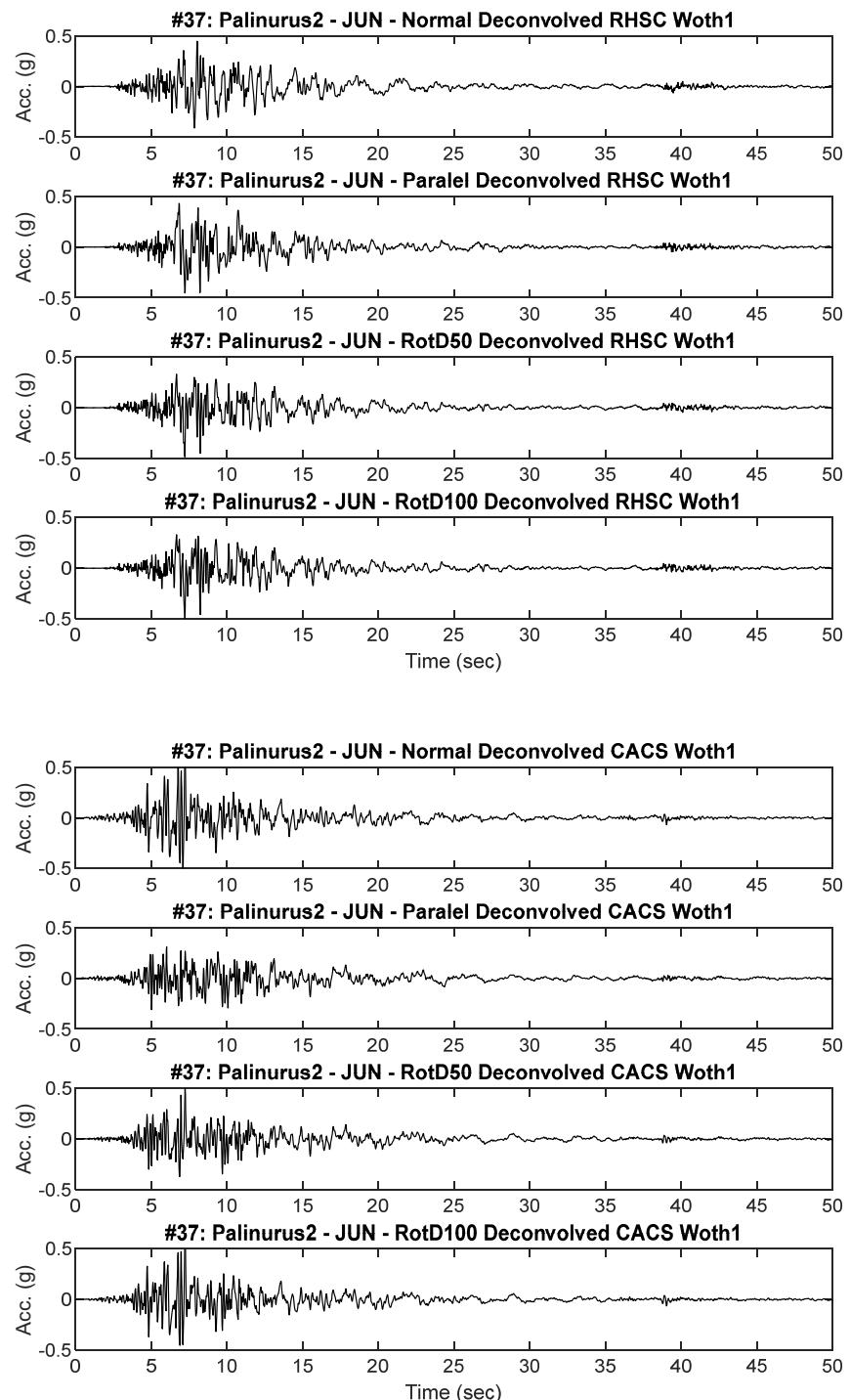
**Figure B37.2 Scaled RHSC and CACS Deconvolved input motion acceleration time history placed at Riccarton Gravel elevation for dynamic analysis**
