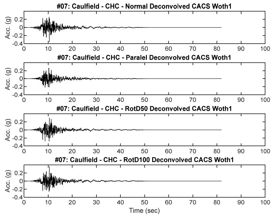
**Figure B7.2 Scaled RHSC and CACS Deconvolved input motion acceleration time history placed at Riccarton Gravel elevation for dynamic analysis**
