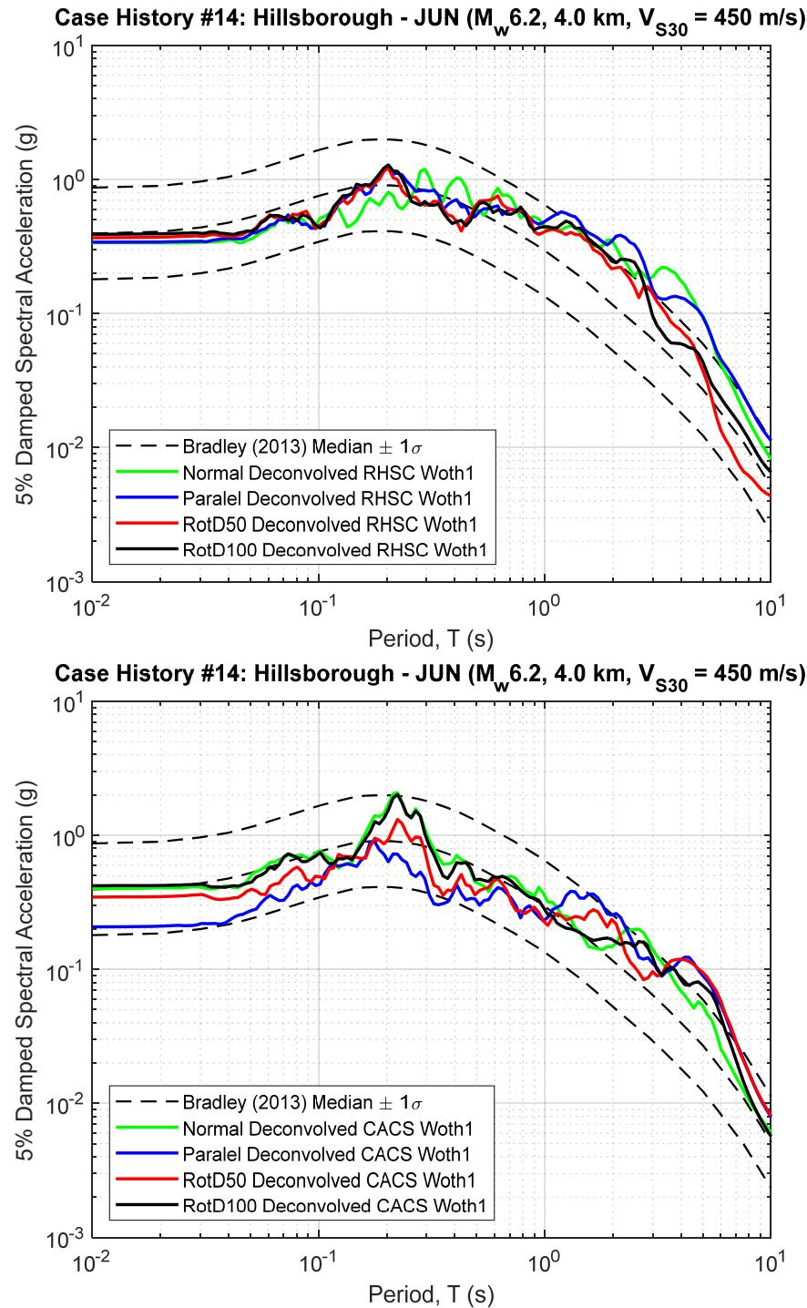
**Figure B14.1 5% Damped Response Spectra of RHSC and CACS Deconvolved Input Motion at Riccarton Gravel (multiplied by the scaling factor to represent the  $R_{rup}$  and  $V_{S30}$  of studied site)**
