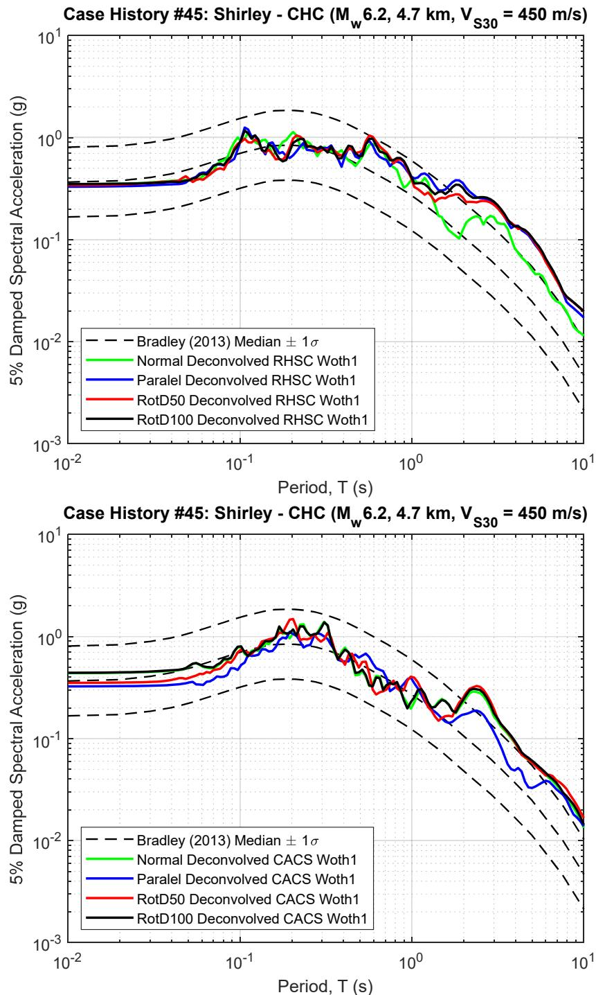
**Figure B45.1 5% Damped Response Spectra of RHSC and CACS Deconvolved Input Motion at Riccarton Gravel (multiplied by the scaling factor to represent the  $R_{rup}$  and  $V_{S30}$  of studied site)**
