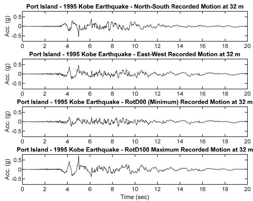
**Figure B44.2 Acceleration time histories of Port Island Input Ground Motion**
