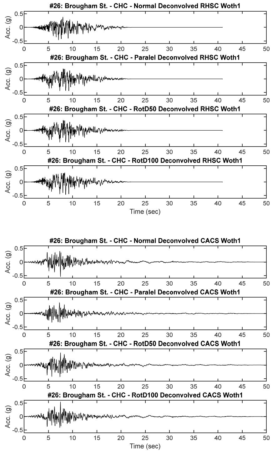
**Figure B26.2 Scaled RHSC and CACS Deconvolved input motion acceleration time history placed at Riccarton Gravel elevation for dynamic analysis**
