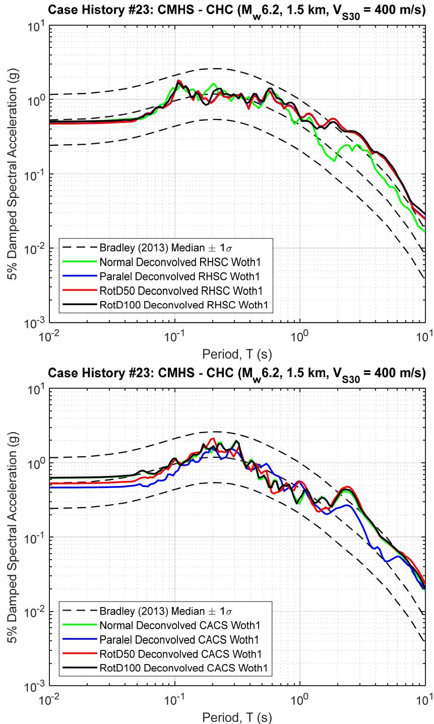
**Figure B23.1 5% Damped Response Spectra of RHSC and CACS Deconvolved Input Motion at Riccarton Gravel (multiplied by the scaling factor to represent the  $R_{rup}$  and  $V_{S30}$  of studied site)**
