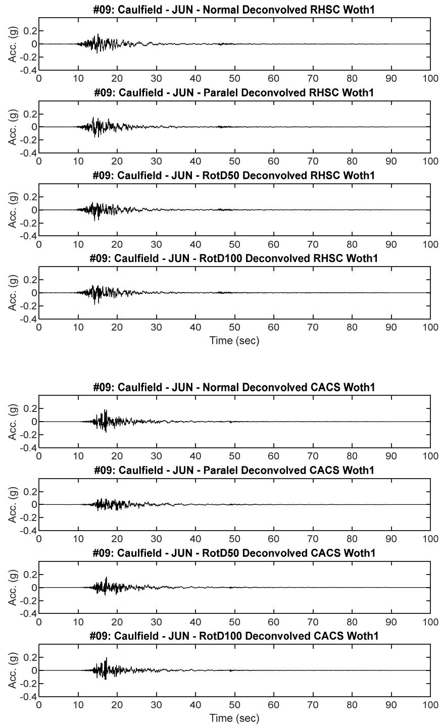
Figure B9.2 Scaled RHSC and CACS Deconvolved input motion acceleration time history placed at Riccarton Gravel elevation for dynamic analysis
