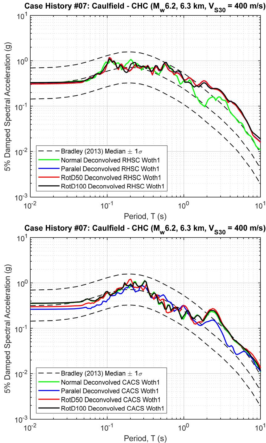
**Figure B7.1 5% Damped Response Spectra of RHSC and CACS Deconvolved Input Motion at Riccarton Gravel (multiplied by the scaling factor to represent the  $R_{rup}$  and  $V_{S30}$  of studied site)**
