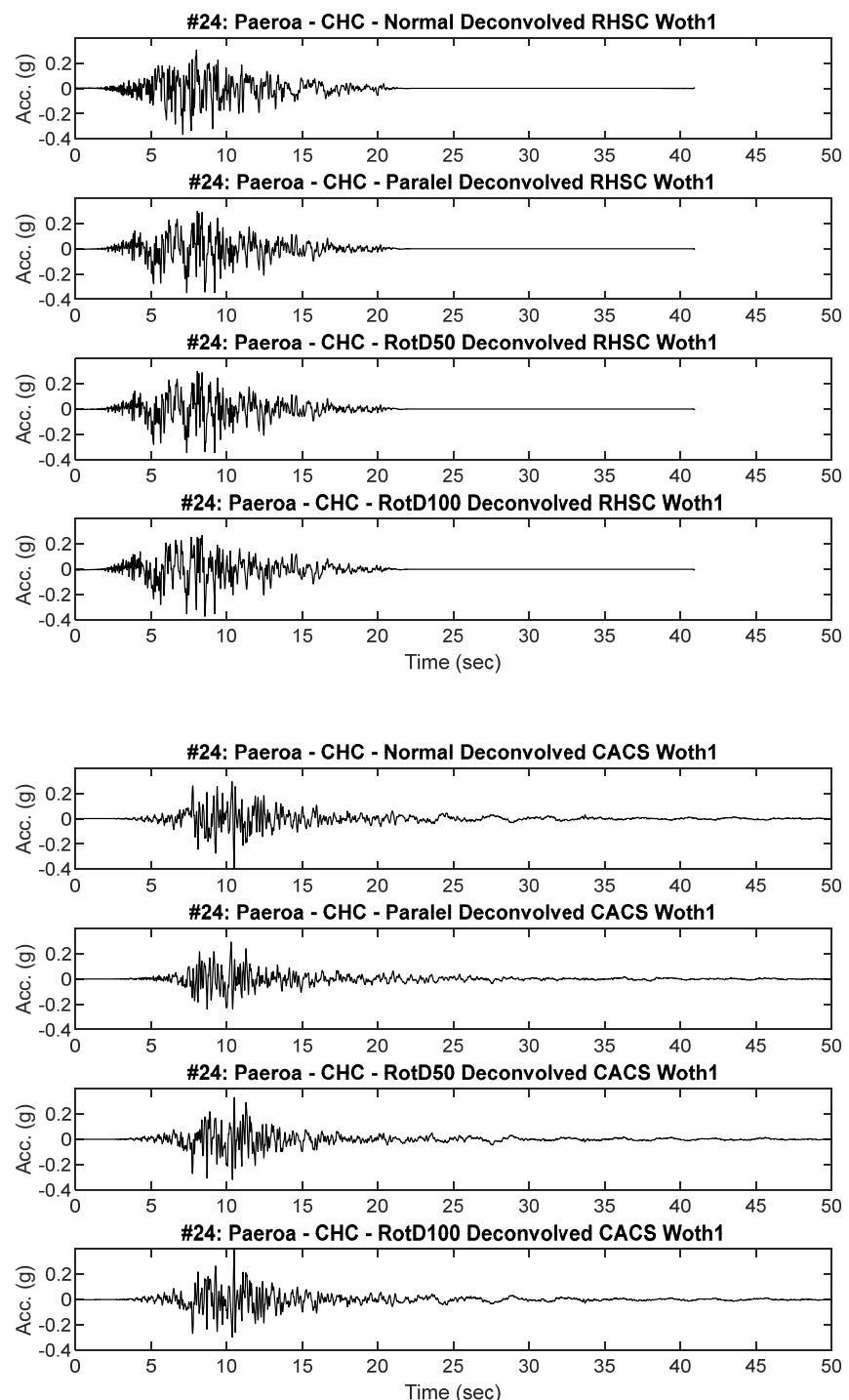
**Figure B24.2 Scaled RHSC and CACS Deconvolved input motion acceleration time history placed at Riccarton Gravel elevation for dynamic analysis**
