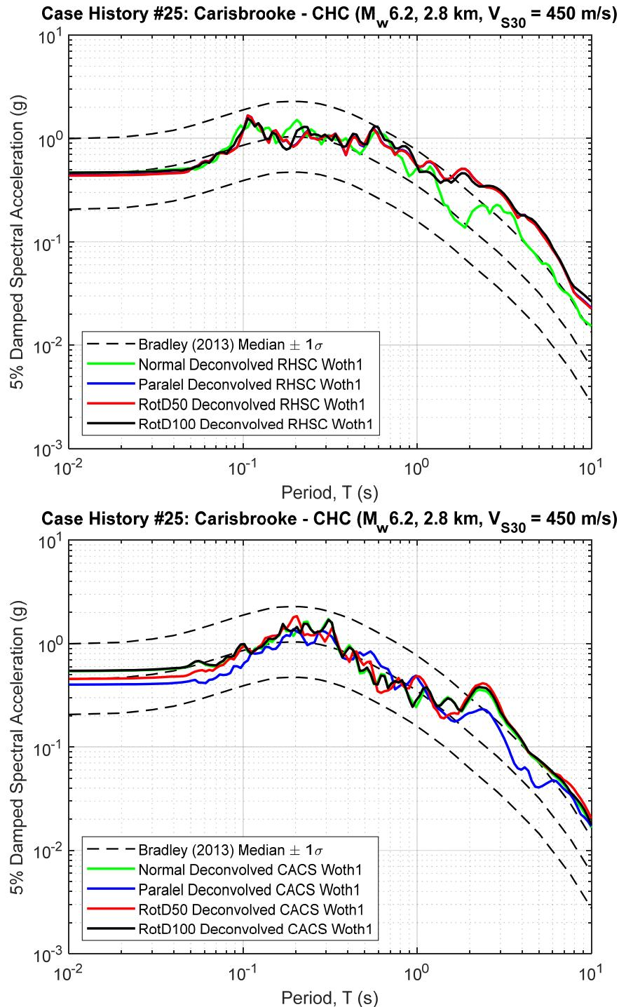
**Figure B25.1 5% Damped Response Spectra of RHSC and CACS Deconvolved Input Motion at Riccarton Gravel (multiplied by the scaling factor to represent the  $R_{rup}$  and  $V_{S30}$  of studied site)**
