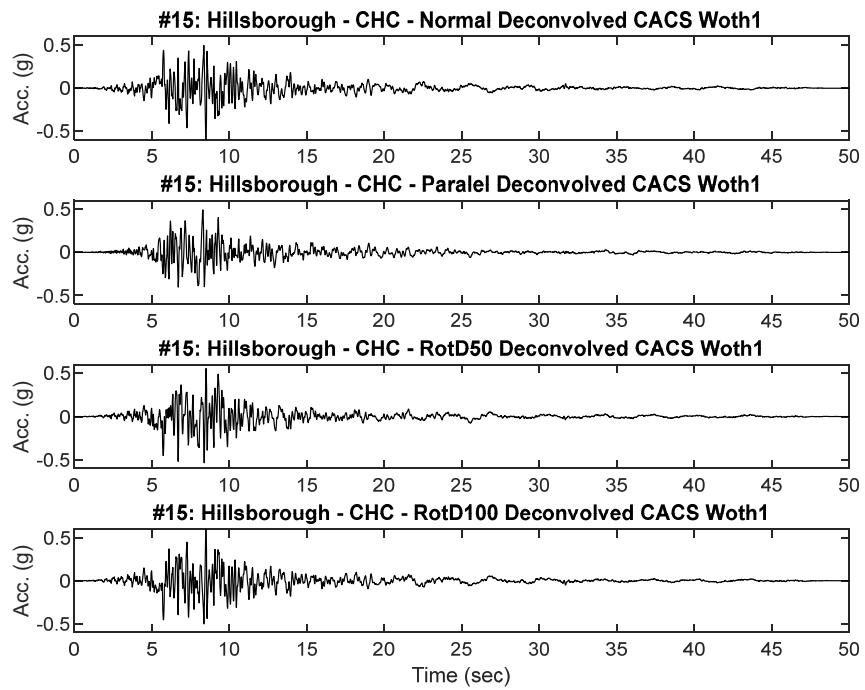
**Figure B15.2 Scaled RHSC and CACS Deconvolved input motion acceleration time history placed at Riccarton Gravel elevation for dynamic analysis**
