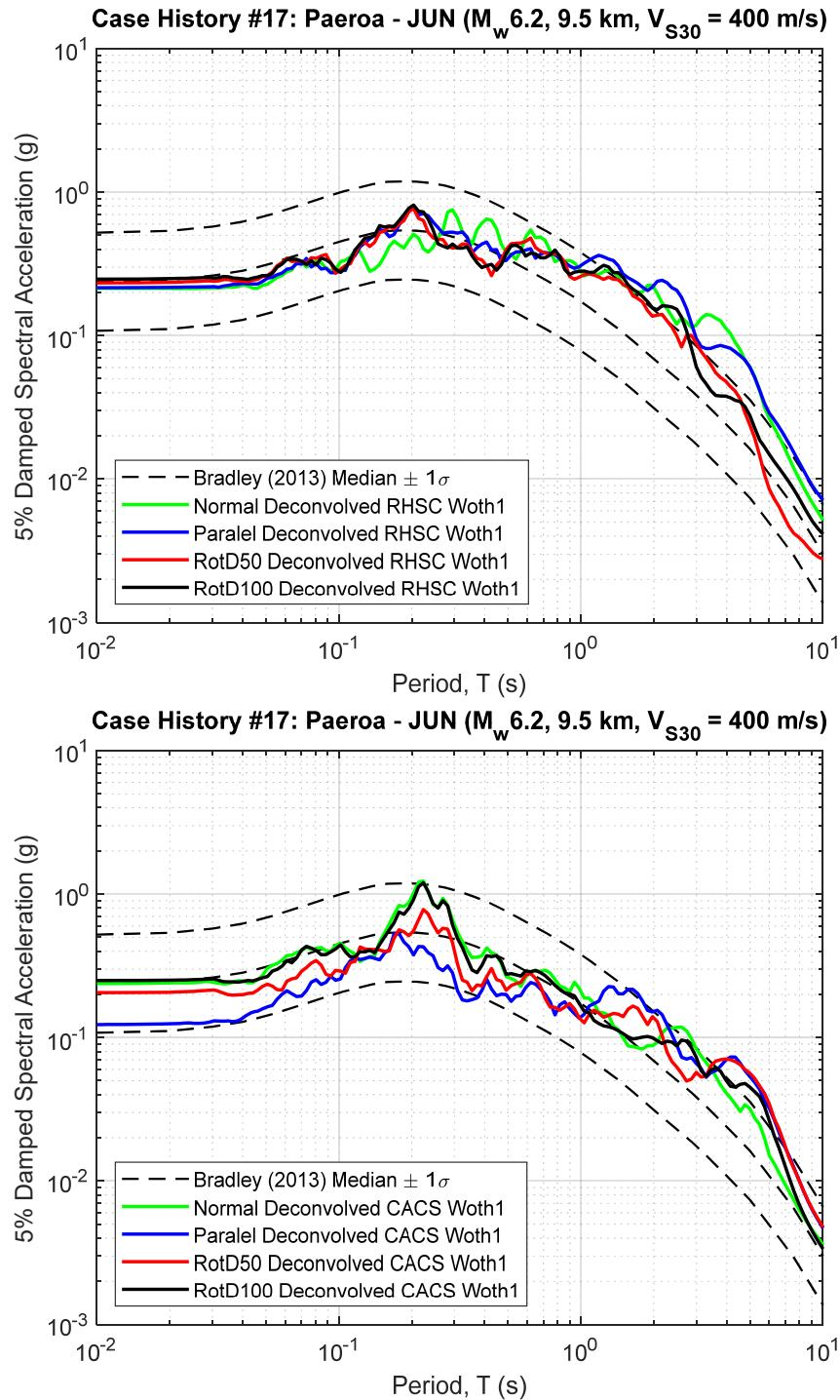
**Figure B17.1 5% Damped Response Spectra of RHSC and CACS Deconvolved Input Motion at Riccarton Gravel (multiplied by the scaling factor to represent the  $R_{rup}$  and  $V_{S30}$  of studied site)**
