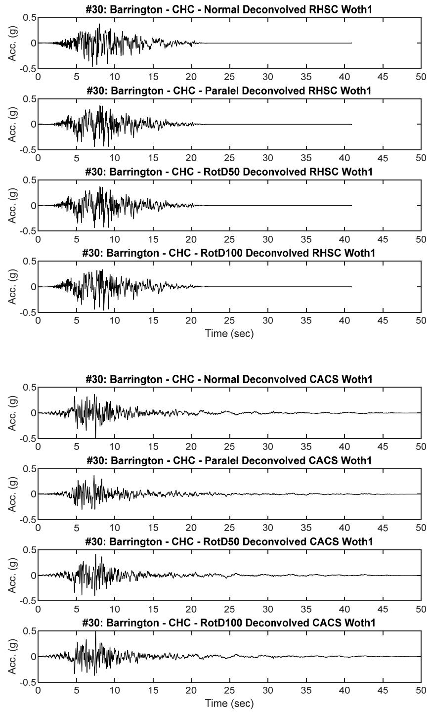
**Figure B30.2 Scaled RHSC and CACS Deconvolved input motion acceleration time history placed at Riccarton Gravel elevation for dynamic analysis**
