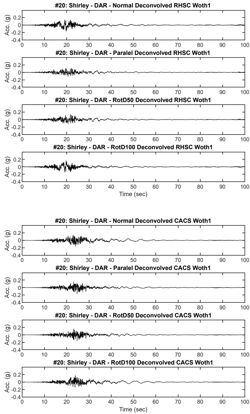
**Figure B20.2 Scaled RHSC and CACS Deconvolved input motion acceleration time history placed at Riccarton Gravel elevation for dynamic analysis**
