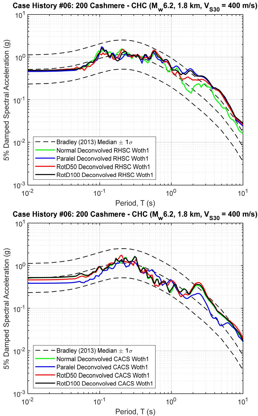
**Figure B6.1 5% Damped Response Spectra of RHSC and CACS Deconvolved Input Motion at Riccarton Gravel (multiplied by the scaling factor to represent the  $R_{rup}$  and  $V_{S30}$  of studied site)**
