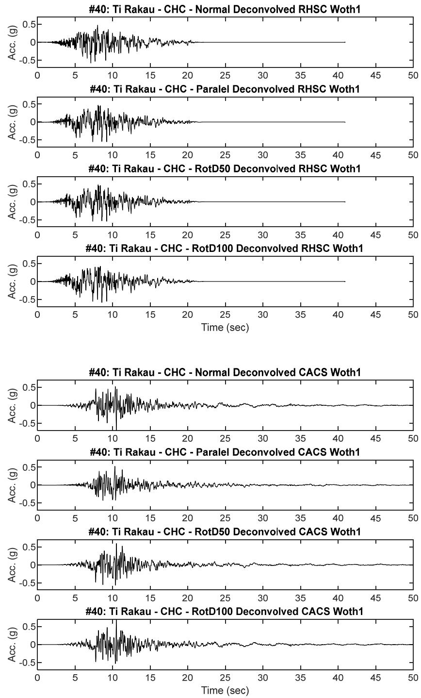
**Figure B40.2 Scaled RHSC and CACS Deconvolved input motion acceleration time history placed at Riccarton Gravel elevation for dynamic analysis**
