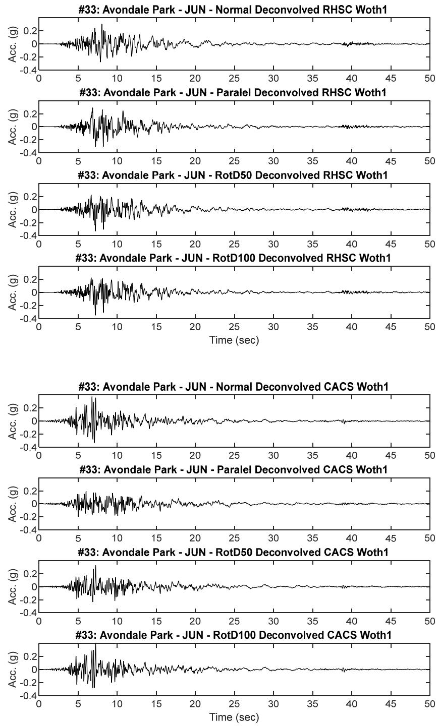
**Figure B33.2 Scaled RHSC and CACS Deconvolved input motion acceleration time history placed at Riccarton Gravel elevation for dynamic analysis**
