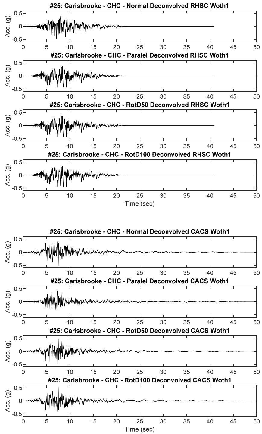
**Figure B25.2 Scaled RHSC and CACS Deconvolved input motion acceleration time history placed at Riccarton Gravel elevation for dynamic analysis**
