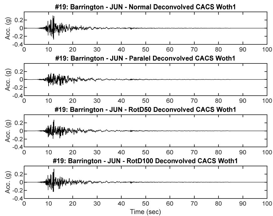
**Figure B19.2 Scaled RHSC and CACS Deconvolved input motion acceleration time history placed at Riccarton Gravel elevation for dynamic analysis**
