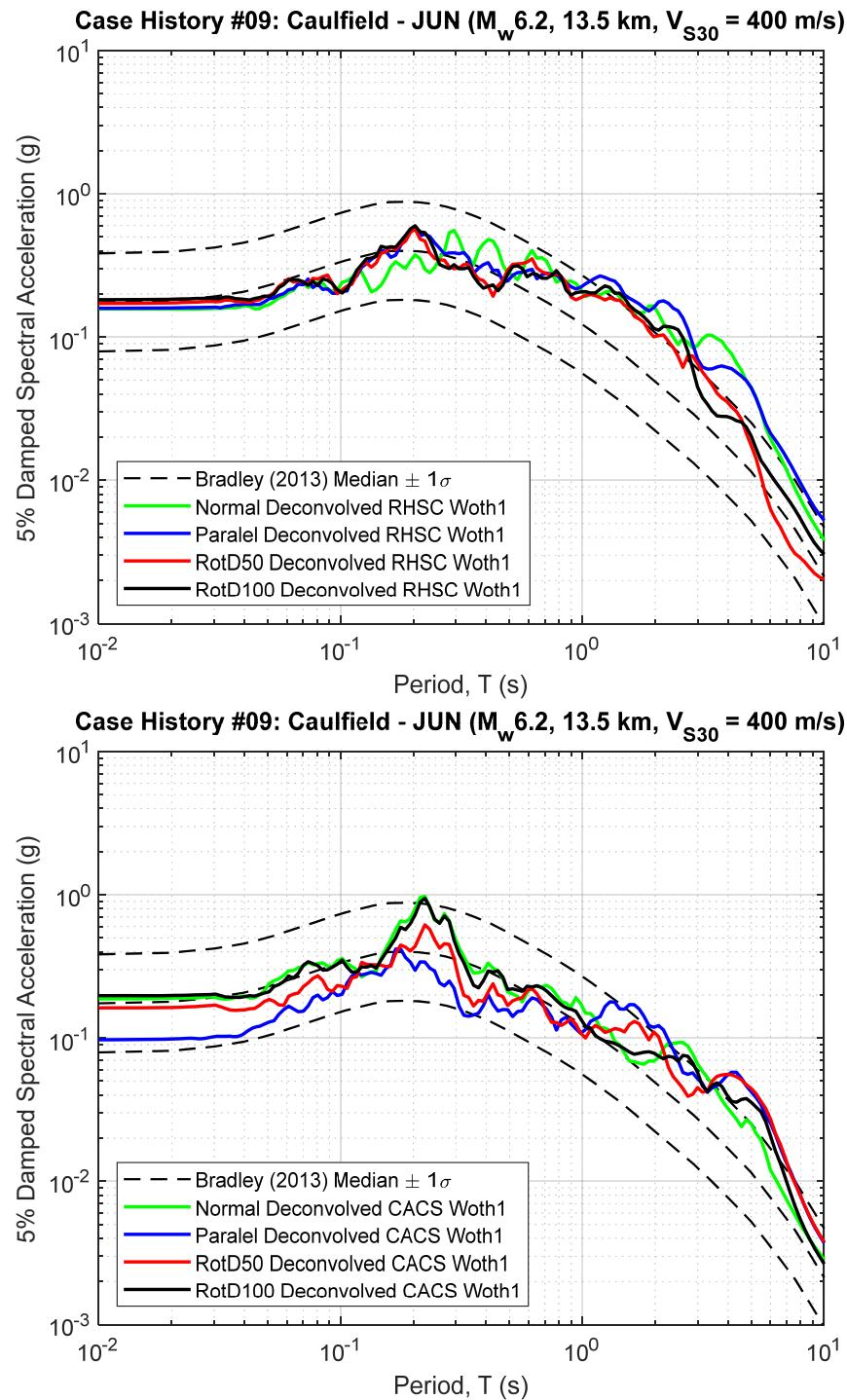
**Figure B9.1 5% Damped Response Spectra of RHSC and CACS Deconvolved Input Motion at Riccarton Gravel (multiplied by the scaling factor to represent the  $R_{rup}$  and  $V_{S30}$  of studied site)**
