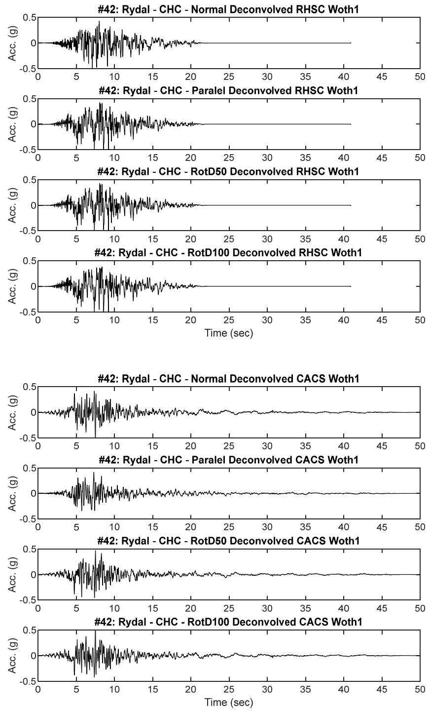
**Figure B42.2 Scaled RHSC and CACS Deconvolved input motion acceleration time history placed at Riccarton Gravel elevation for dynamic analysis**
