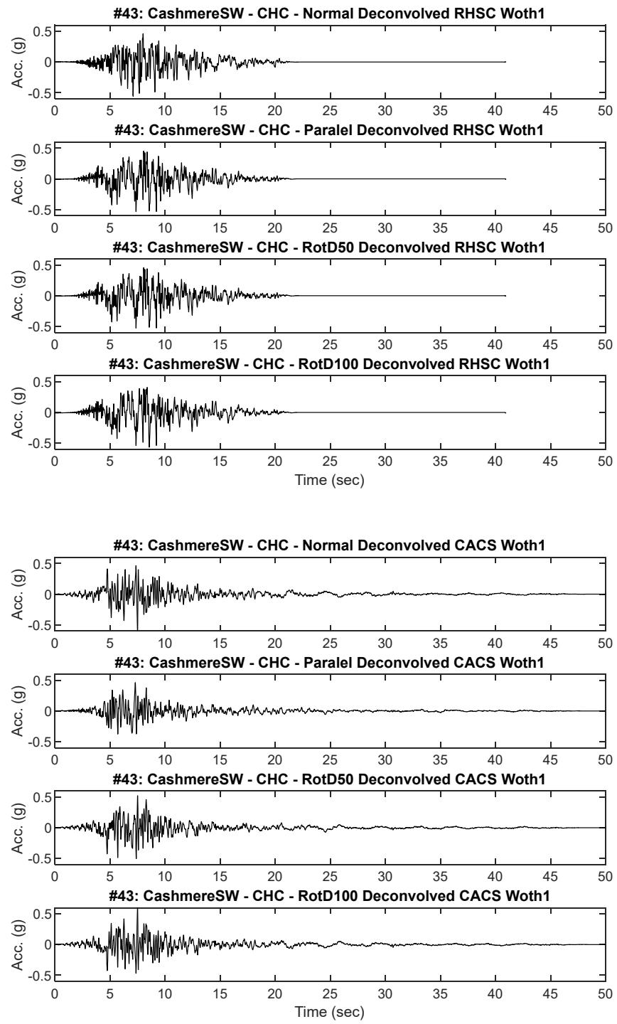
**Figure B43.2 Scaled RHSC and CACS Deconvolved input motion acceleration time history placed at Riccarton Gravel elevation for dynamic analysis**
