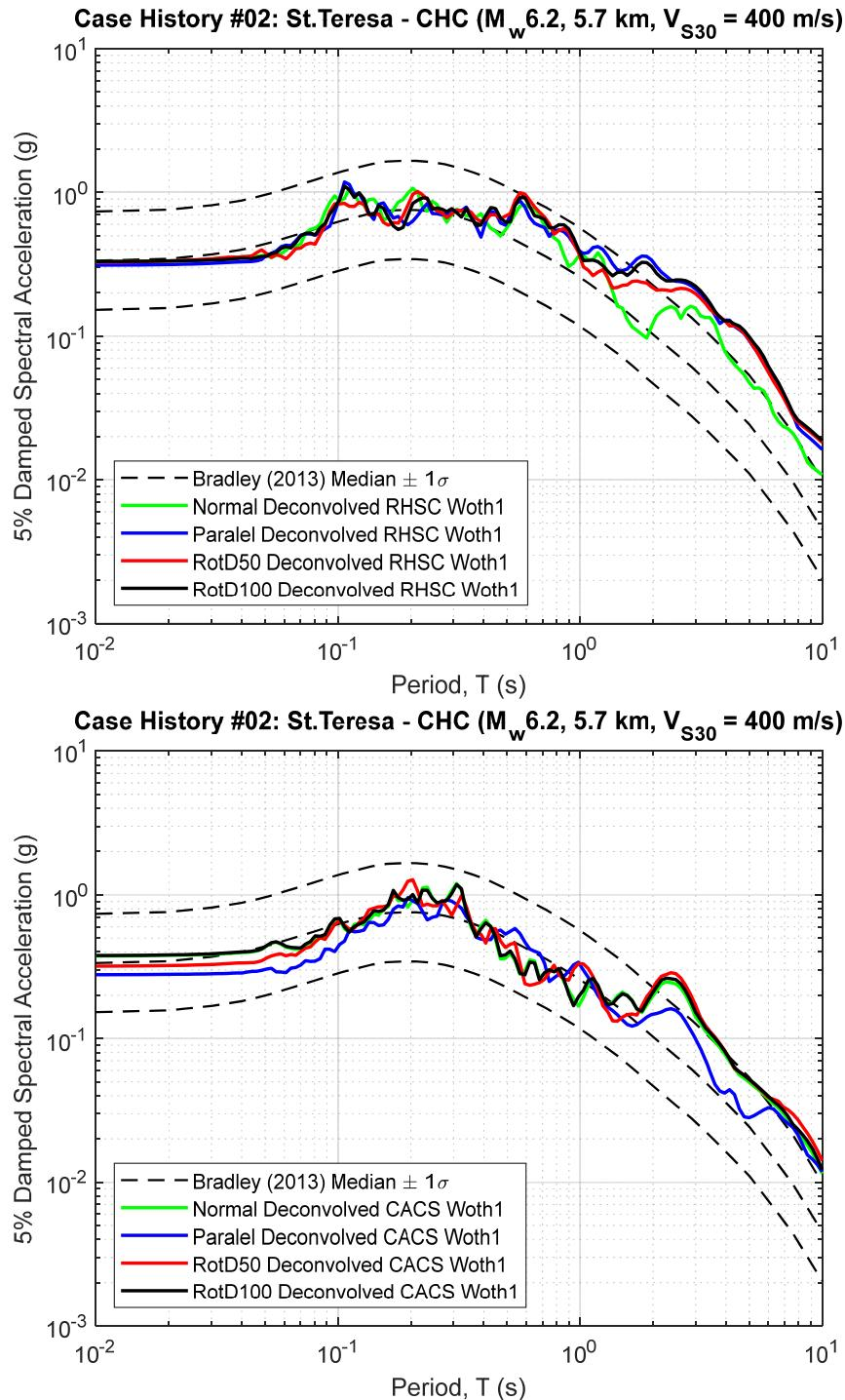
**Figure B2.1 5% Damped Response Spectra of RHSC and CACS Deconvolved Input Motion at Riccarton Gravel (multiplied by the scaling factor to represent the  $R_{rup}$  and  $V_{S30}$  of studied site)**
