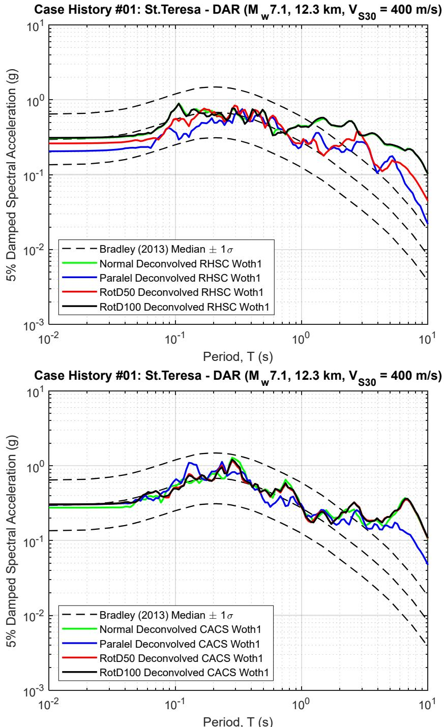
**Figure B1.1 5% Damped Response Spectra of RHSC and CACS Deconvolved Input Motion at Riccarton Gravel (multiplied by the scaling factor to represent the  $R_{rup}$  and  $V_{S30}$  of studied site)**
