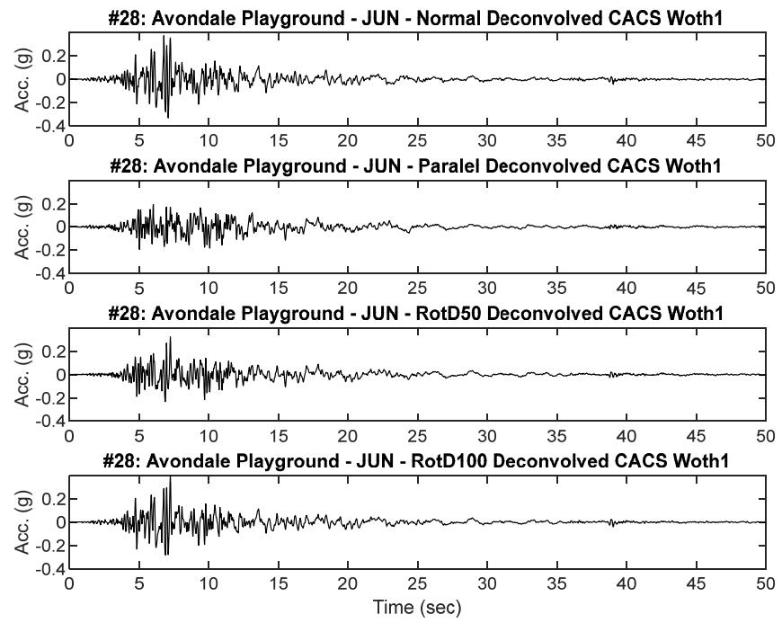
**Figure B28.2 Scaled RHSC and CACS Deconvolved input motion acceleration time history placed at Riccarton Gravel elevation for dynamic analysis**
