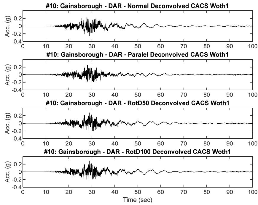
**Figure B10.2 Scaled RHSC and CACS Deconvolved input motion acceleration time history placed at Riccarton Gravel elevation for dynamic analysis**
