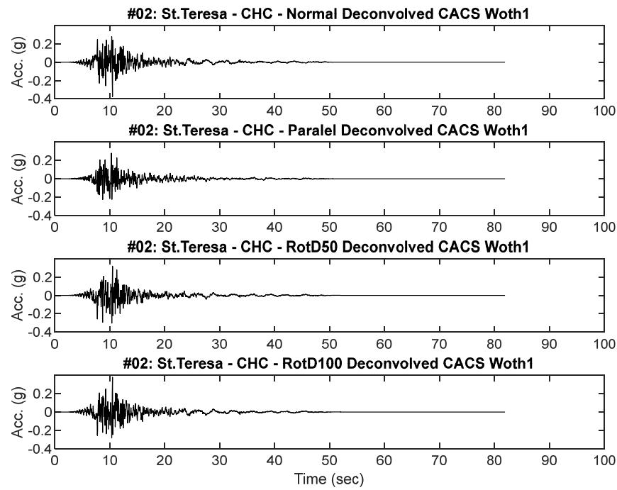
**Figure B2.2 Scaled RHSC and CACS Deconvolved input motion acceleration time history placed at Riccarton Gravel elevation for dynamic analysis**
