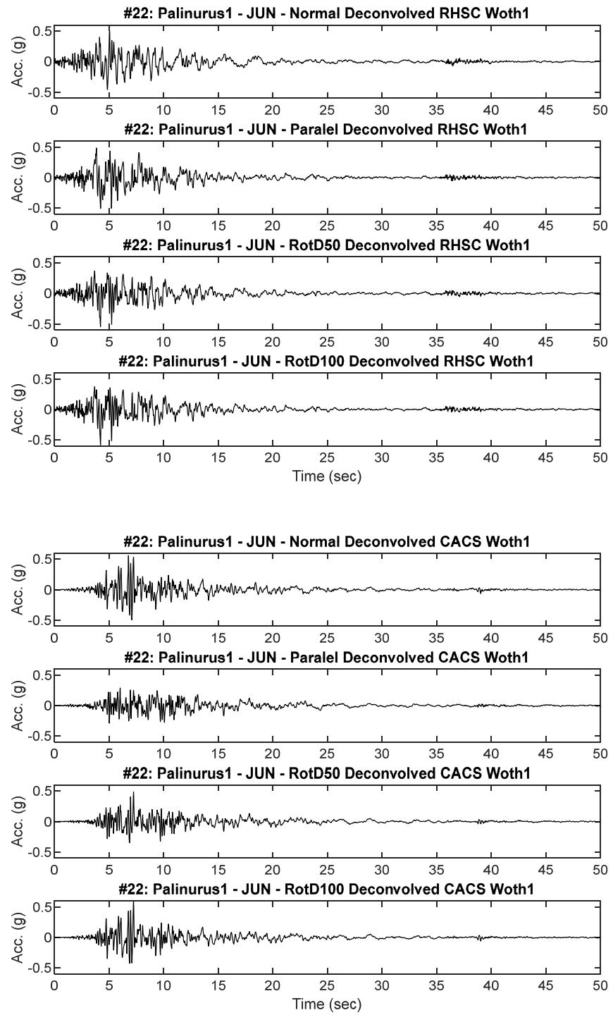
**Figure B22.2 Scaled RHSC and CACS Deconvolved input motion acceleration time history placed at Riccarton Gravel elevation for dynamic analysis**
