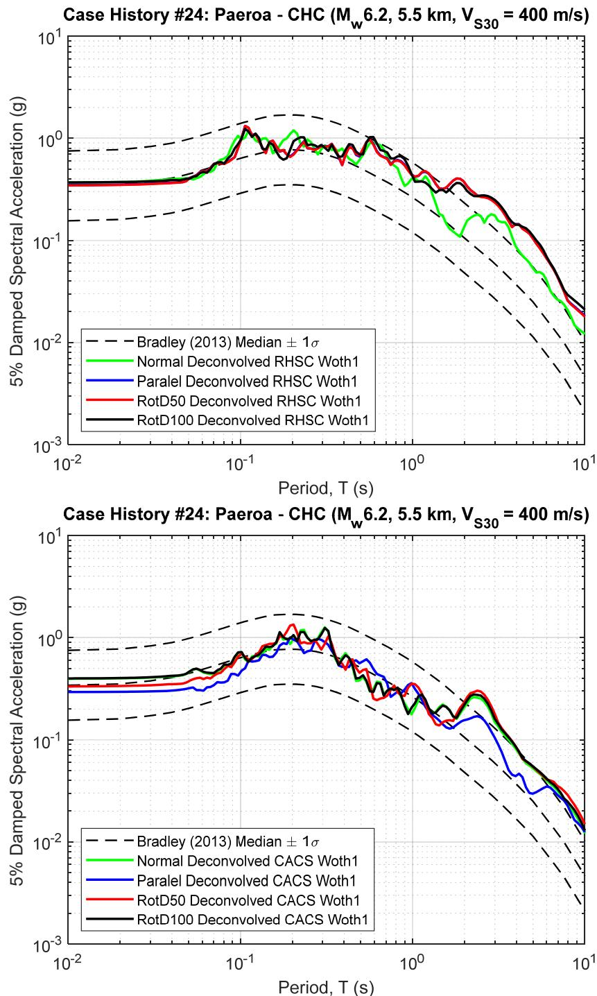
**Figure B24.1 5% Damped Response Spectra of RHSC and CACS Deconvolved Input Motion at Riccarton Gravel (multiplied by the scaling factor to represent the  $R_{rup}$  and  $V_{S30}$  of studied site)**
