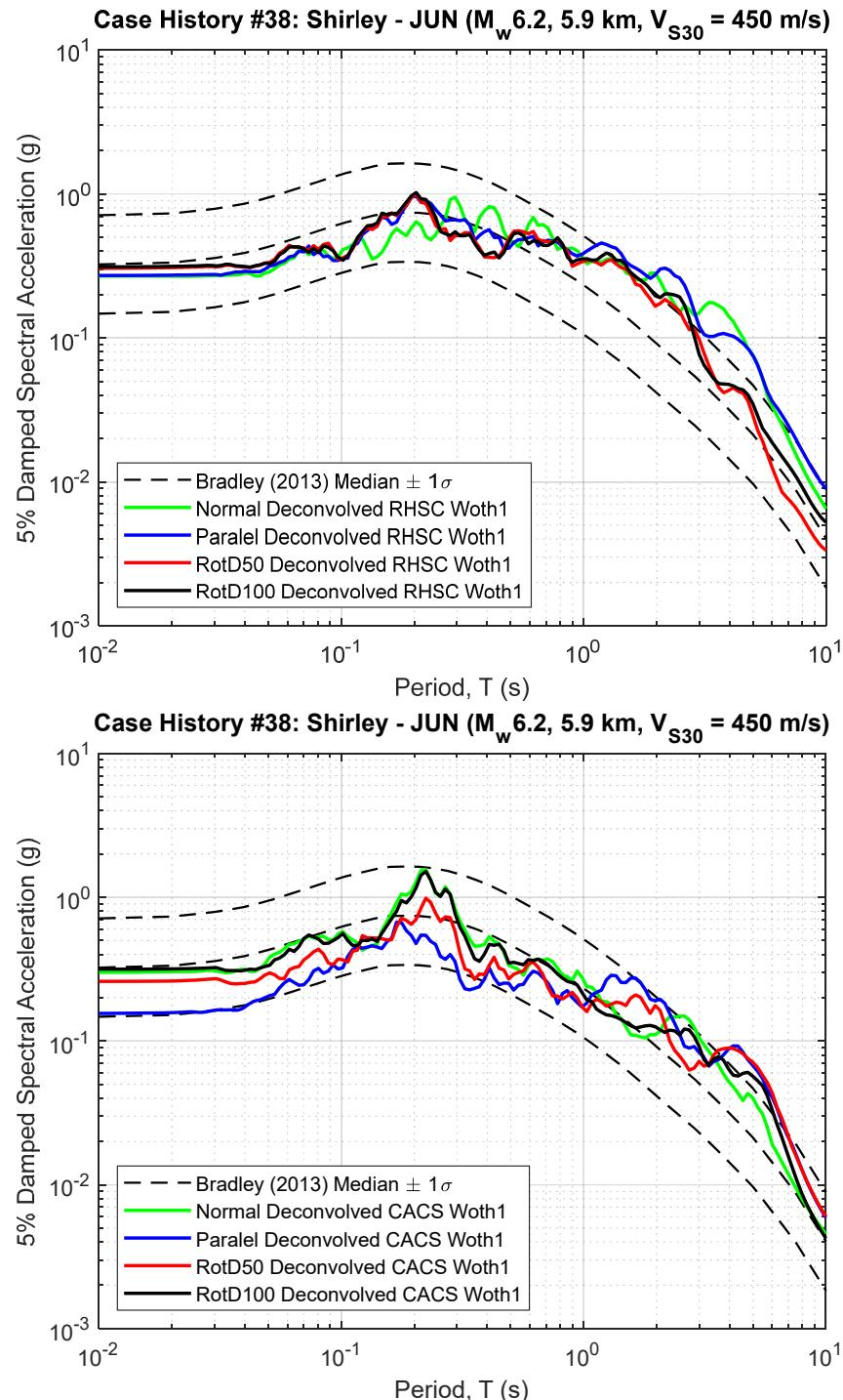
**Figure B38.1 5% Damped Response Spectra of RHSC and CACS Deconvolved Input Motion at Riccarton Gravel (multiplied by the scaling factor to represent the  $R_{rup}$  and  $V_{S30}$  of studied site)**
