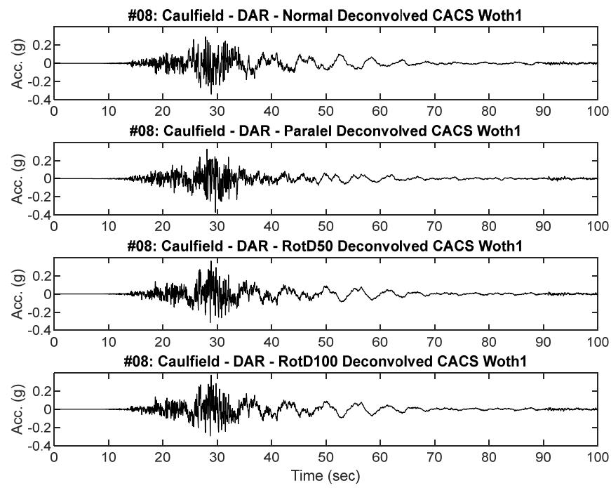
**Figure B8.2 Scaled RHSC and CACS Deconvolved input motion acceleration time history placed at Riccarton Gravel elevation for dynamic analysis**
