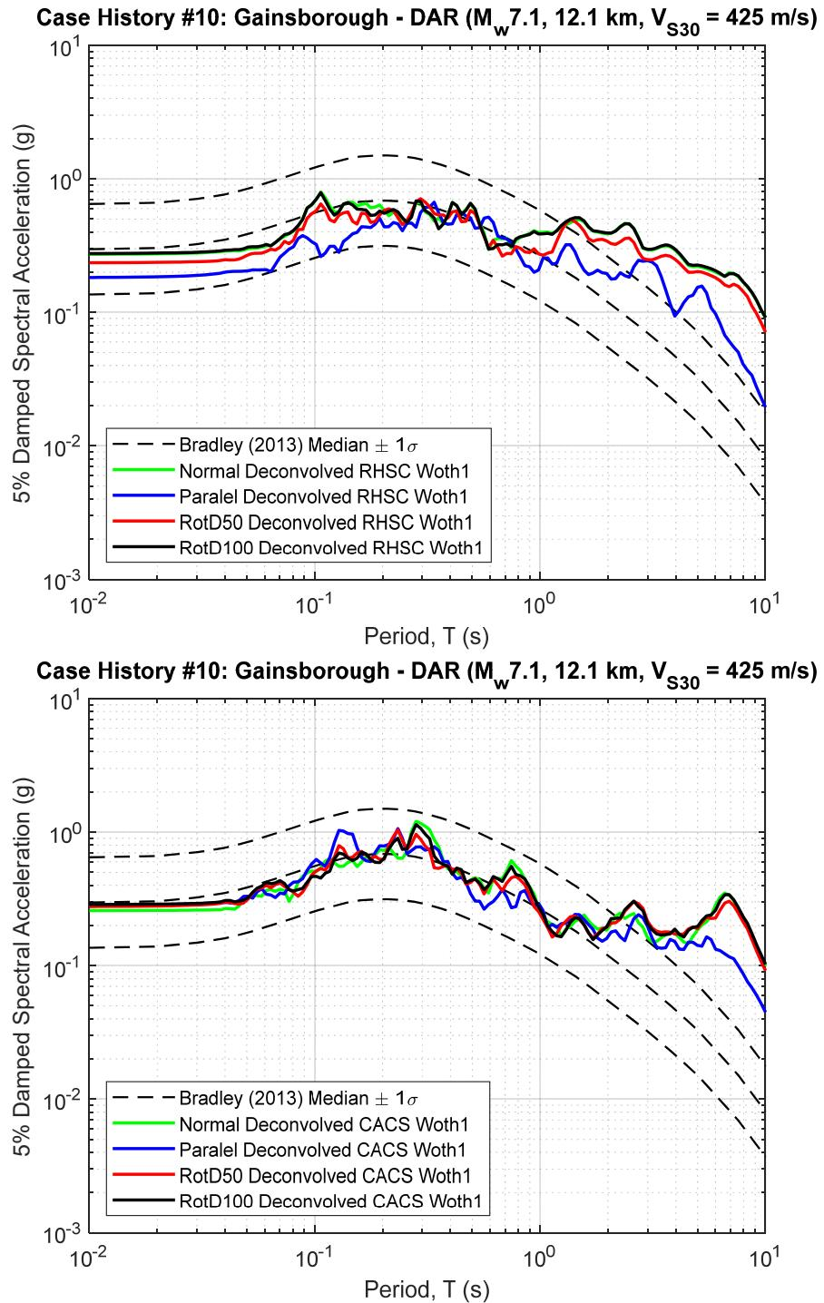
**Figure B10.1 5% Damped Response Spectra of RHSC and CACS Deconvolved Input Motion at Riccarton Gravel (multiplied by the scaling factor to represent the  $R_{rup}$  and  $V_{S30}$  of studied site)**
