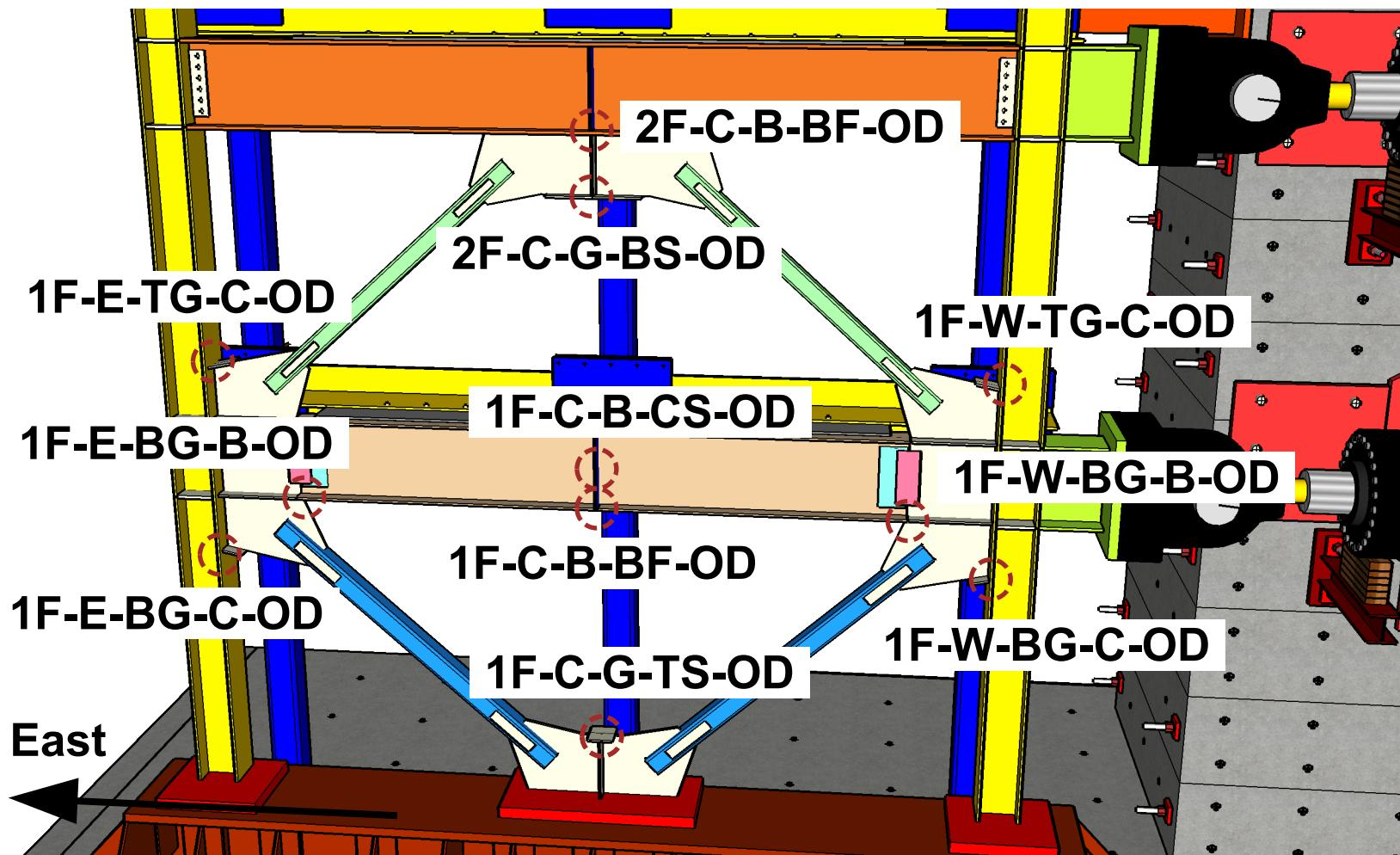
C: column side corner; B: beam side corner
