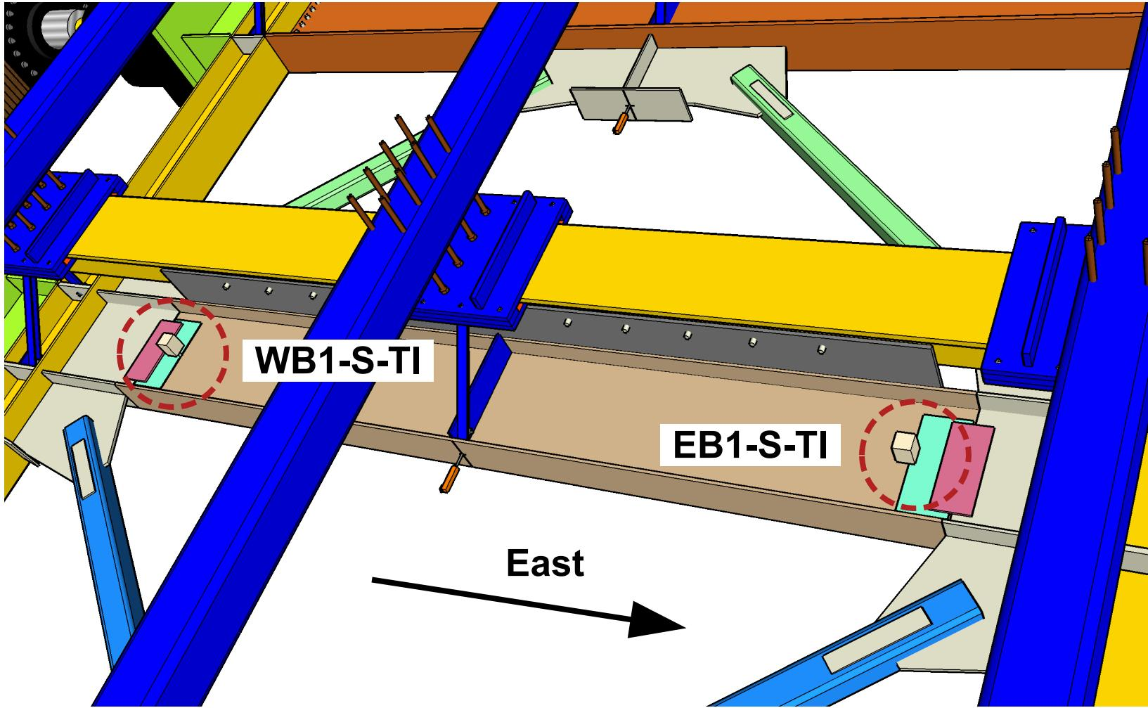
**WB1-S-TI: west lower beam (1F) rotation monitoring**
