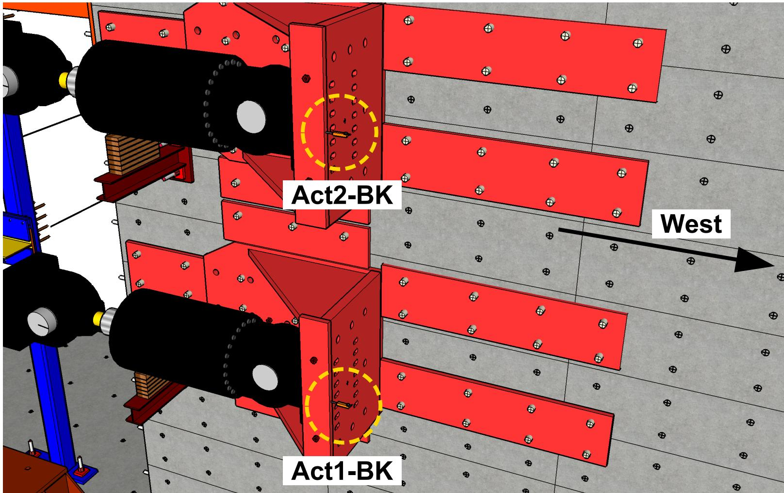
**Act1-BK:** lower actuator bracket deformation monitoring
