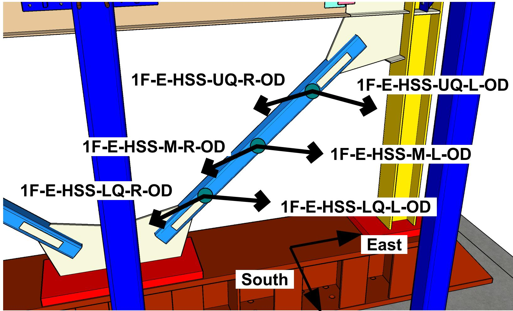
**Typical brace out-of-plane deformation monitoring (wire pot directions are shown in the figure for one brace, other braces are similar, six wire pots per brace)**
