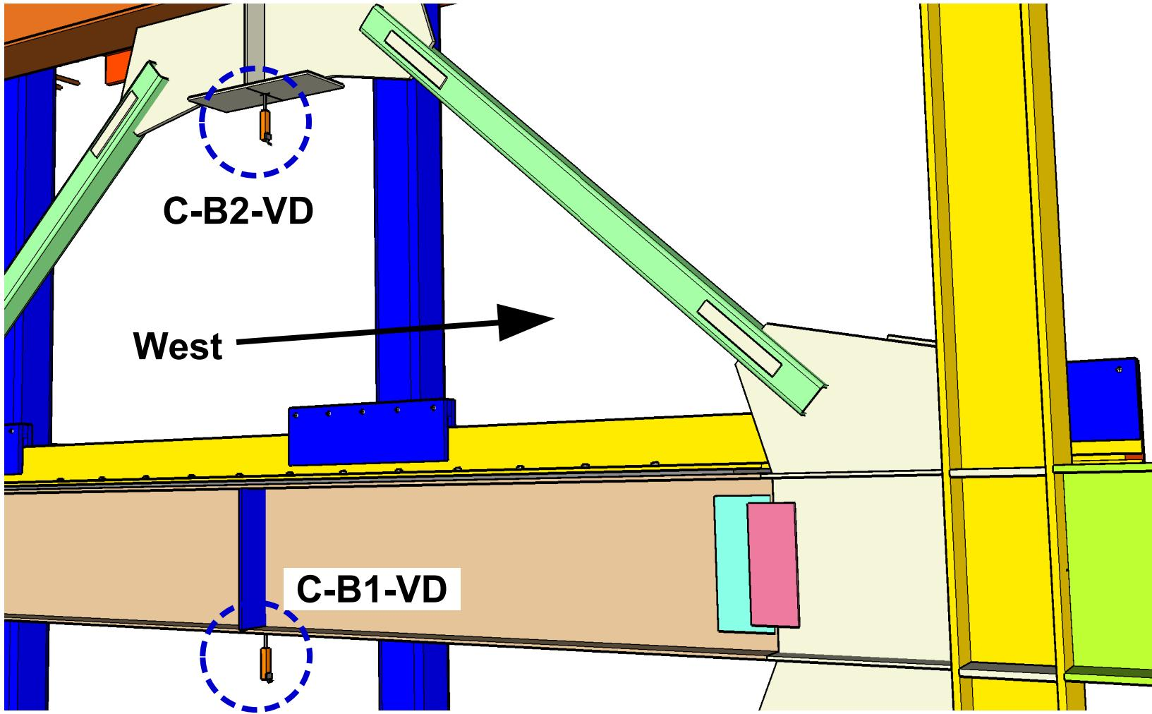
**C-B2-VD: roof beam (2F) center deflection monitoring**
