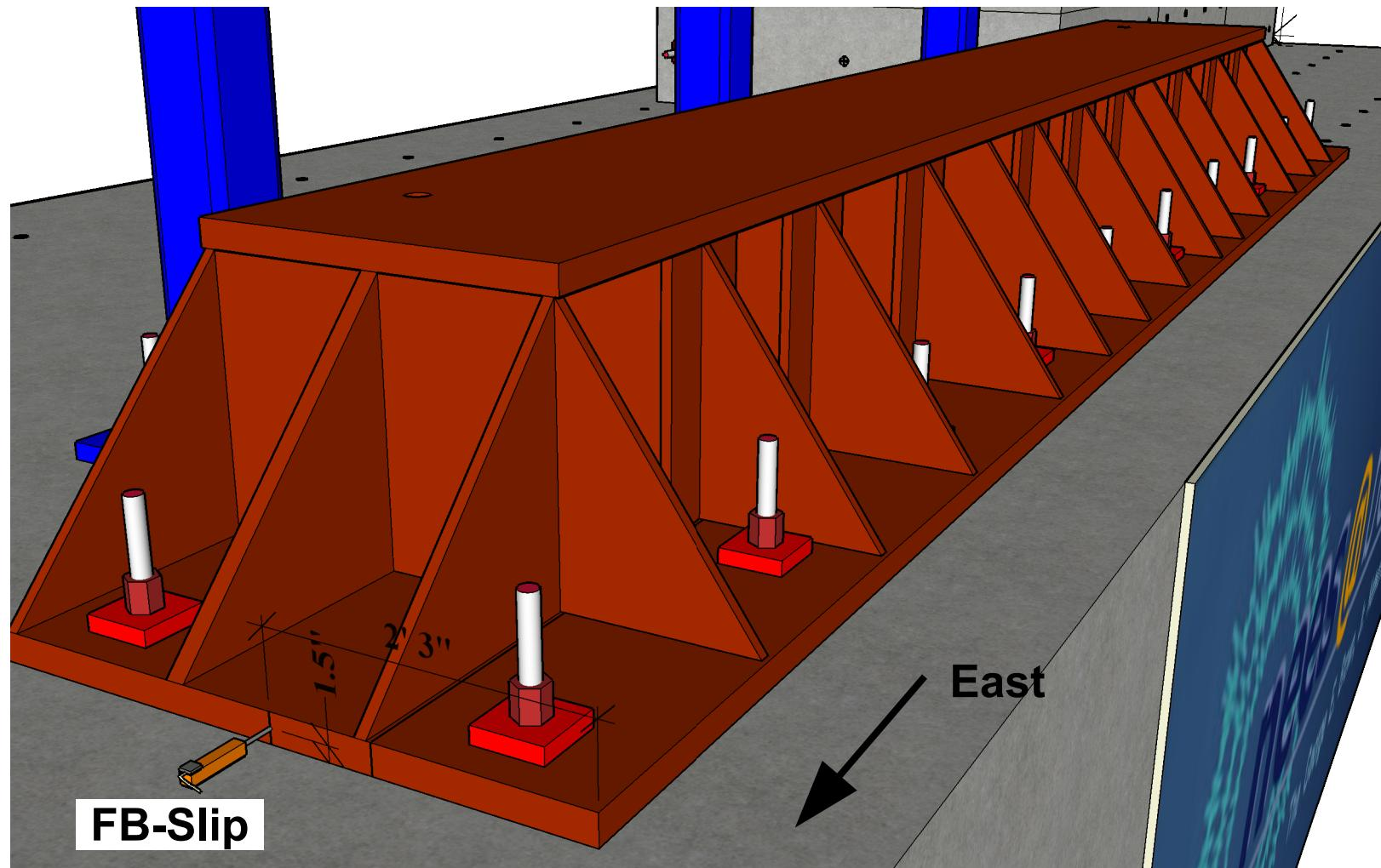
**FB-Slip: floor beam slip monitoring (east side, location is shown in the figure)**
