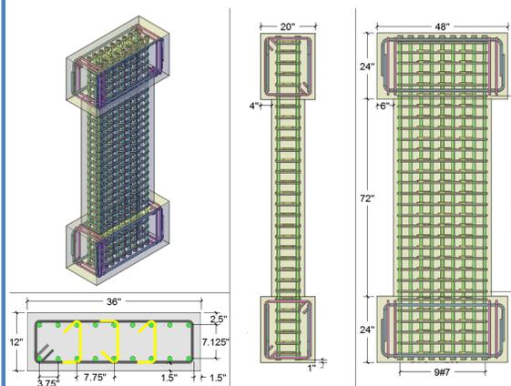
Figure 2. Reinforcement layout.
