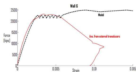
Figure 4. Comparison of Structural response of Wall 6 and the predicted model.
