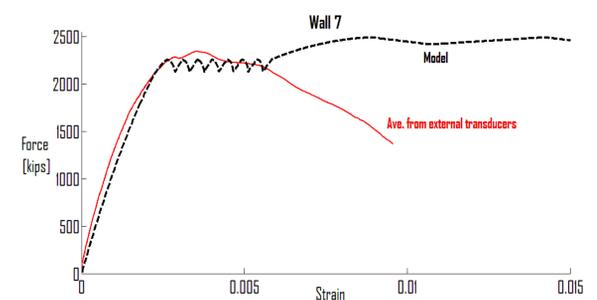
Figure 5. Comparison of Structural response of Wall 7 and the predicted model.
