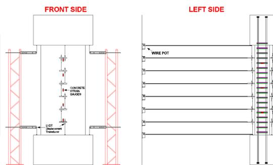
Figure 3. Layout of the instrumentation used during testing.
