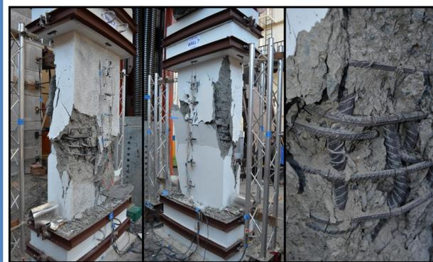
Figure 6. Wall 7 after failure. Brittle failure can be attributed to buckling of the longitudinal rebar.
