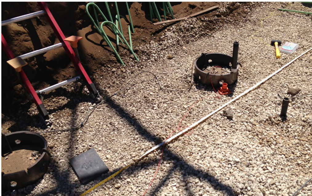
Figure B.3 Pilot study test piles and free-field accelerometers.
