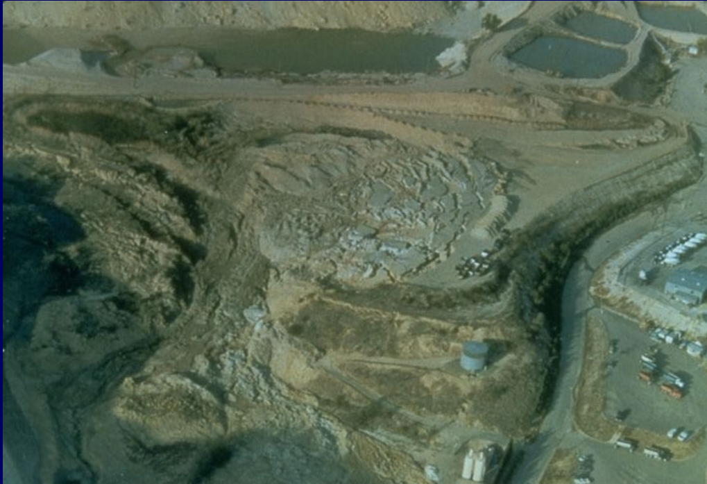
Tapo Canyon Liquefaction-Induced Tailings Dam Failure (picture from Y. Moriwaki)
