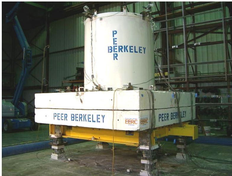
Fig. 2. Fully instrumented test specimen on the shaking table.
