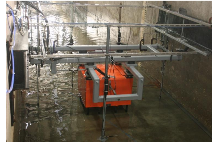
Elevated Structure instrumented at Hinsdale Wave Research Laboratory (HWRL) Oregon State University
