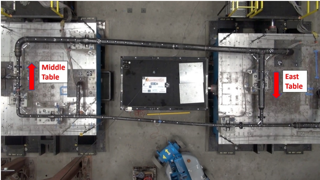
Figure 27: Piping deformation at 17 in of relative shake table displacement
