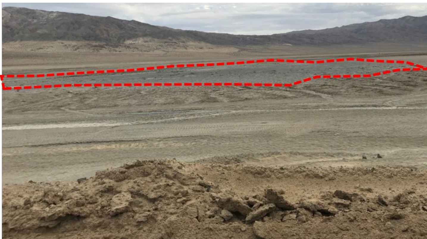
Figure 6. Photograph of Narrow band of ejecta from liquefaction in Searles Lake
