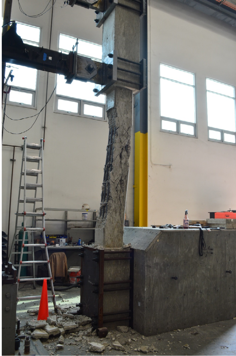
Column specimen after shear failure in diagonal tension, shown after displacements up to 6 inches. The shear failure occurred on the first cycle to 2-inch displacement.
