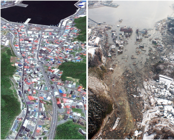
Fig. 1. Tsunami destruction pattern in the town of Onagawa, Japan: (left – before the 2011 Tsunami [source: Google Earth]; right – after the event [source: Satake]). A pair of sturdy buildings at the waterfront acted as barriers for the buildings behind. The gap between the buildings created a swift jet flow, wiping out everything in the flow path.
