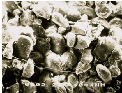
Figure 2. Photograph of the fabric in fine to medium beach sand showing the intimate packing of the grains with concave-convex mating surfaces (N. Sitar original)
