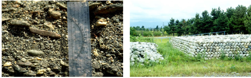
Figure 1. Left: Elongate gravel particles arranged in an imbricate (shingle-like) fabric in glacial outwash gravels, Utah. Right: Oval, well rounded boulders arranged in a tight packing stand at a much steeper slope than randomly deposited boulders of the same type, Japan (N. Sitar originals).
