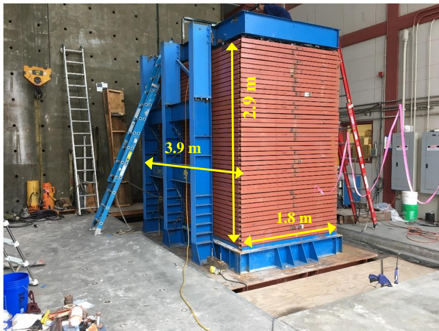
Fig. 1: Laminar Soil Box at UCSD Powell Laboratory (H2.9m×L3.9m×W1.8m)
