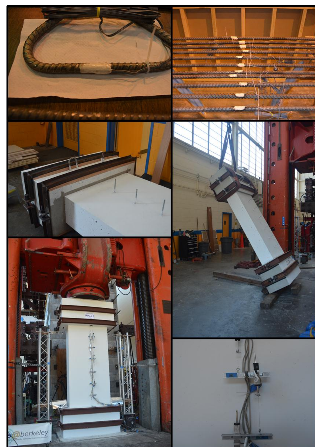
Figure 2. stages in the instrumentation and set up process of Wall 5 test
