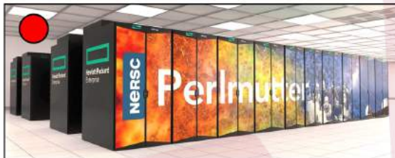
Perlmutter (completed 2022) Lawrence Berkeley National Lab National Energy Research Scientific Computing Center (NERSC) 1536 GPU accelerated nodes 4 NVIDIA A100 GPUs / node 71 PetaFlops Top500.org #8
