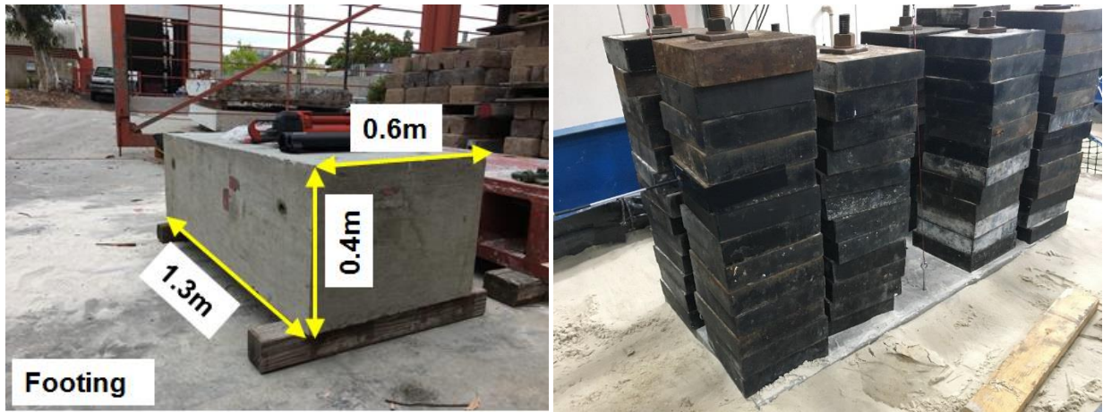
Fig. 2: Model footing prior to placement and weights to replicate target contact pressure
