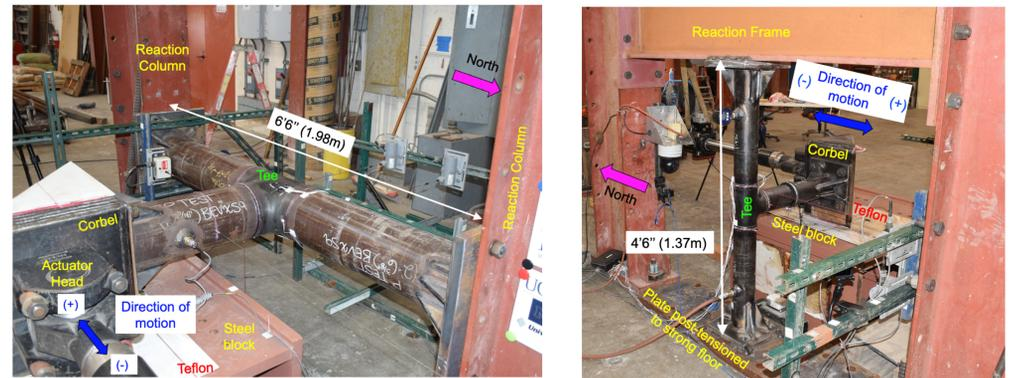
Figure 1. Test setup for in-plane loading (left) and out-of-plane loading (right).
