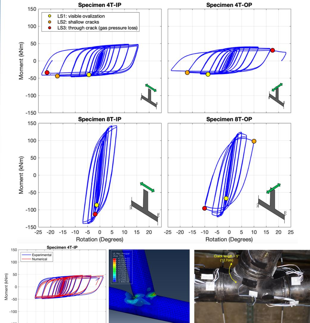
Figure 2. Select experimental moment-rotation hysteretic response of tee-joint specimens (top) and comparison with Abaqus FE modeling (bottom).
