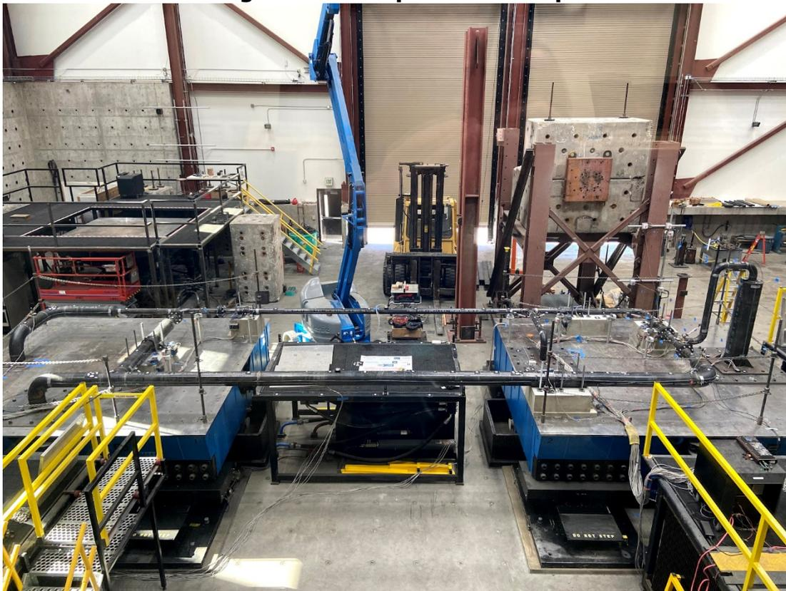
Strain sensing fiber cables were attached onto the pipeline specimen along the longitudinal directions of the pipeline to measure the permanent strain distribution changes after each shaking cycle. A Brillouin Optical Time Domain Reflectometry (BOTDR) based analyzer was used for strain measurements. The specification of the analyzer is given in Table A-3. The distributed strain data was also used for calculating bending curvature and deformation.
