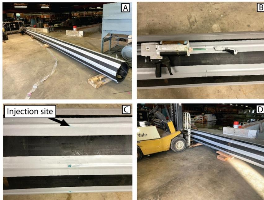
**(A) The instrumented HDPE prior to the vertical bending test, (B) The tools used for DP8010 epoxy injection, (C) Injection sited for DP8010 epoxy and (D) the bending test in progress (Hubbard et al., 2021)**
