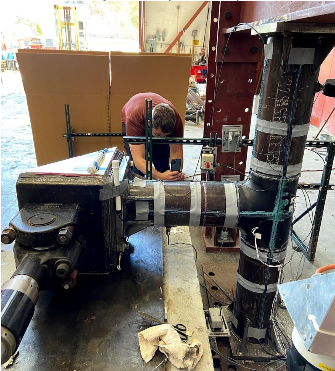
Figure A-22 shows the instrumentation of the fiber optical strain sensing cables, whereas Figure A-23 shows a close-up photo of the two different attachments.
