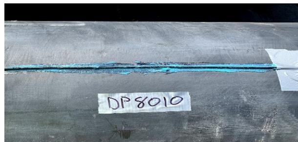
The Tapecoat and DP8010 epoxy both performed well during application. They were simple to apply and provided an initial hold of the cable keeping it in place quickly. This initial hold was instant for the Tapecoat H35 and after about 10 minutes for the DP8010. The pipes and attachment were examined after one week of being kept in an outdoor storage yard. After one week the both the Tapecoat H35 and DP8010 provided a strong bond between the sensing cable and the pipe based on manual examination.
