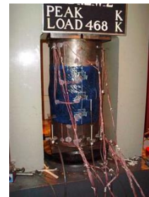
Fiber wrapped joint
