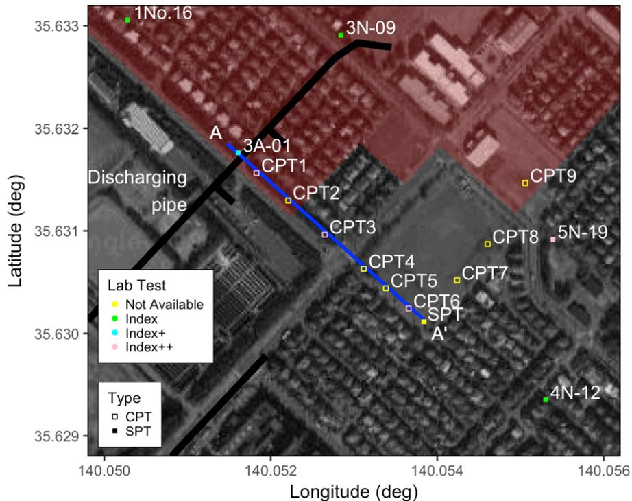
Plan view of 8 Chome Meeting Place site in Mihama Ward, Chiba, Japan. Soil discharging pipe and area with sand boils and ground failure (red shading) are shown. Adapted from: Sekiguchi T, Nakai S. Effects of local site conditions on liquefaction damage in Mihama Ward of Chiba City. *Proceedings of the international symposium on engineering lessons learned from the 2011 greatest Japan earthquake*; March 1–4, 2012; Tokyo, Japan.
